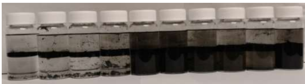
Figure 89: 0.03 wt% MWNTs dispersed in aqueous solutions containing various amounts of CTAB and then mixed with undecanol. The concentrations of CTAB in each vial from left to right is 0 \mu\text{M} , 15 \mu\text{M} , 25 \mu\text{M} , 50 \mu\text{M} , 75 \mu\text{M} , 100 \mu\text{M} , 150 \mu\text{M} , 200 \mu\text{M} , 250 \mu\text{M} , 2500 \mu\text{M} . In the photo it may appear the middle vials have MWNTs entirely in the aqueous phase, but this is due to the quality of the photo. Only the vial at the far right do the MWNTs appear to entirely be in the aqueous phase.
