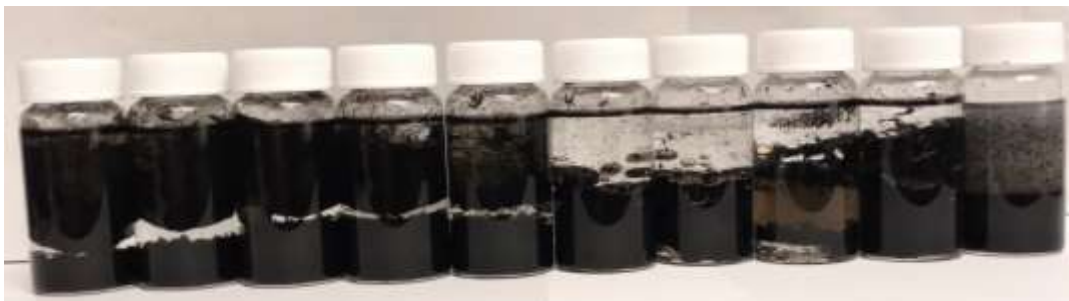
Figure 90: 0.03 wt% MWNTs dispersed in aqueous solutions containing various amounts of CTAB and then mixed with decalin. The concentrations of CTAB in each vial from left to right is 0 \mu\text{M} , 15 \mu\text{M} , 25 \mu\text{M} , 50 \mu\text{M} , 75 \mu\text{M} , 100 \mu\text{M} , 150 \mu\text{M} , 200 \mu\text{M} , 250 \mu\text{M} , 2500 \mu\text{M} .
