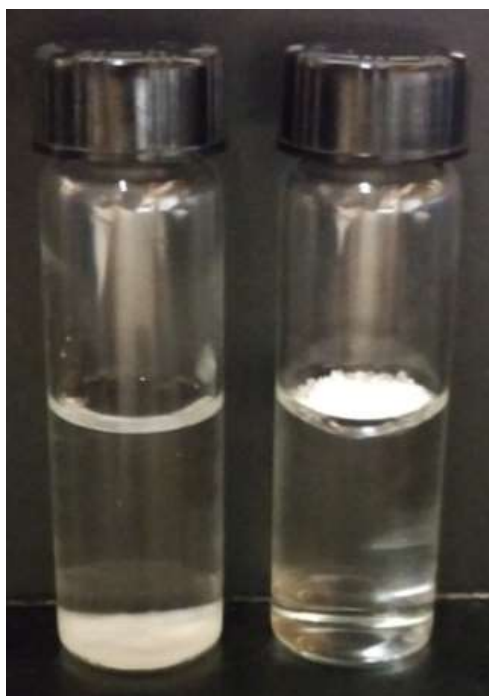
Figure 29: Hydrophilic silica in the vial on the left and hydrophobic silica in the vial on the right.
