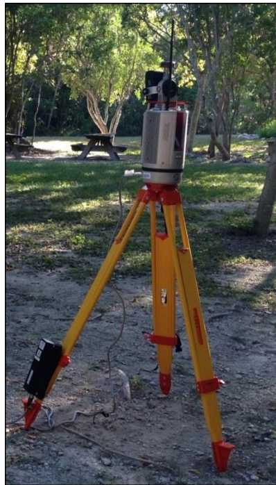
Figure 14: LIDAR mounted on a tripod in the field
