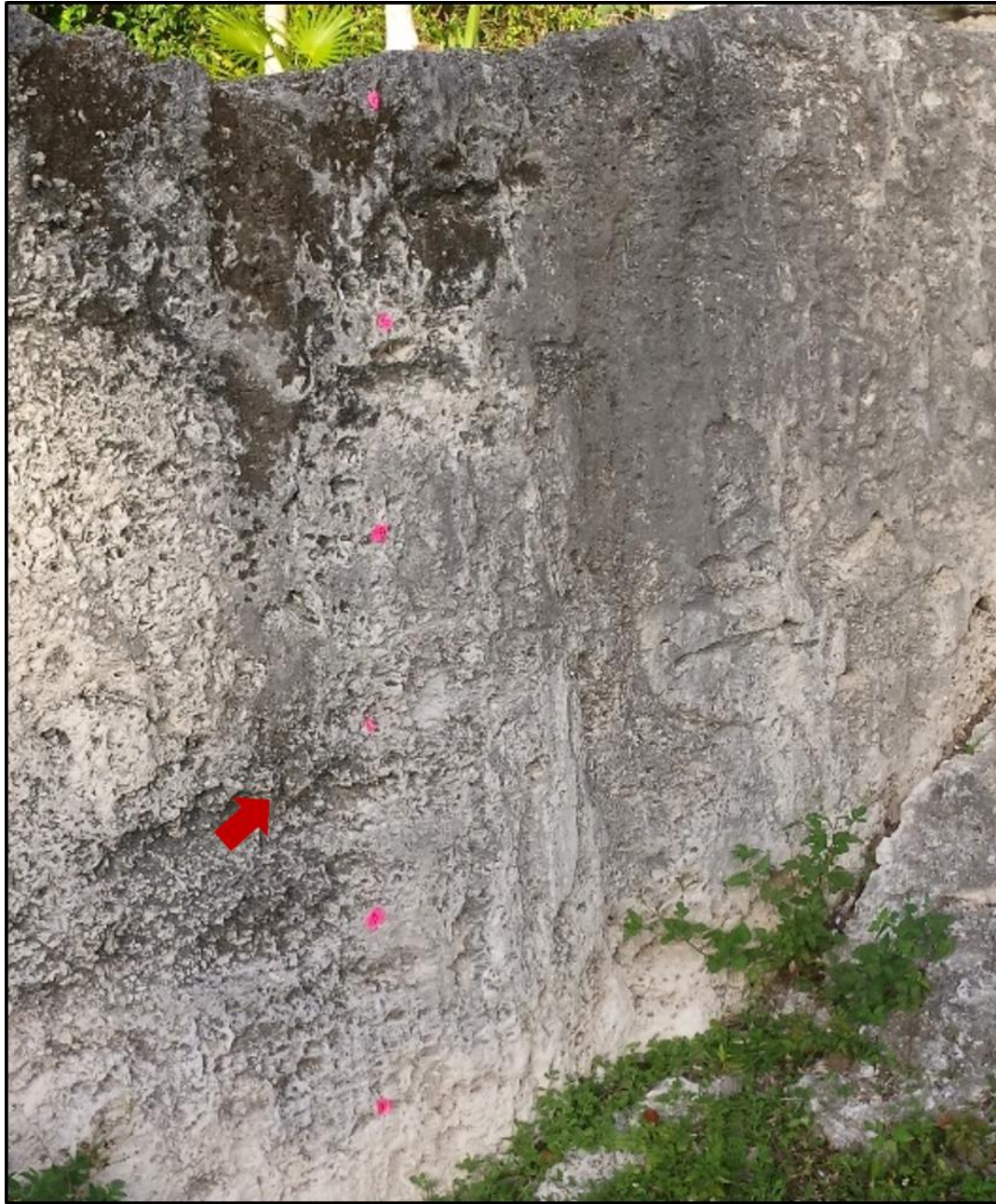
Figure 32: It is not clear where to draw the white line indicating the discontinuity surface from the previous figure. Also, note the lichen near the top of the wall. On the previous figure, this 'vegetation' is more reflective (red).
