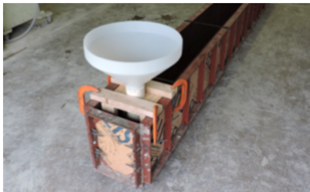
Figure 3.1 Flow Test Fill Hole Set-Up
