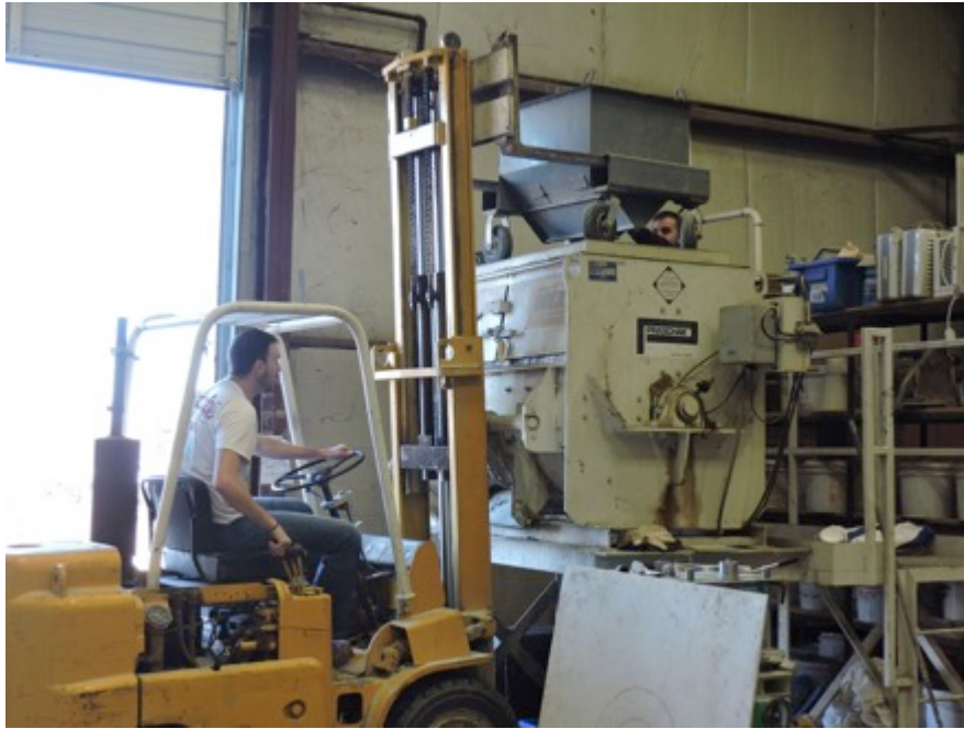
Figure 4.23 Forklift Bucket Transporting Coarse Aggregate
