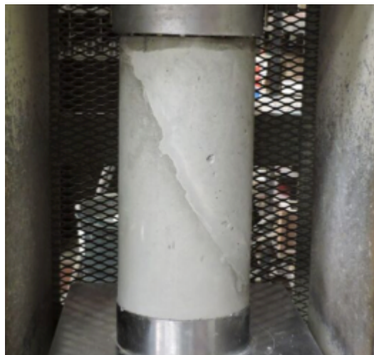
Figure 5.5 Bond Strength Test Set-Up
