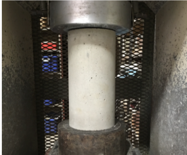
Figure 3.3 4x8 Compression Cylinder Test Set-Up
