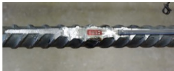
Figure 4.4 Strain Gauge on Tension Bars
