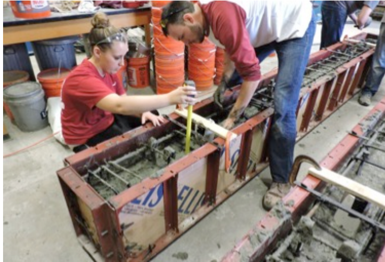
Figure 4.16 Measuring the Slope of the Control Concrete
