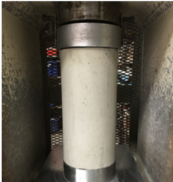
Figure 3.4 6x12 Compression Cylinder Test Set-Up
