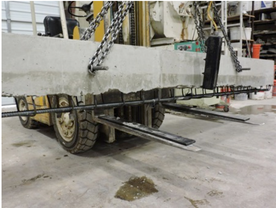
Figure 4.19 Beam Flipped and Tension Bars In Place
