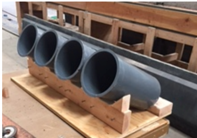
Figure 5.4 Incline Table for Casting the Control Portion
