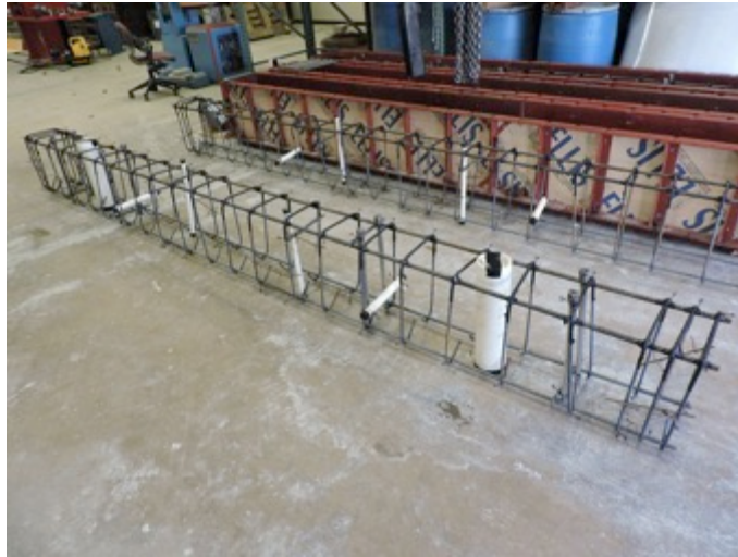
Figure 4.13 FR-SCC Repair Beam Cage
