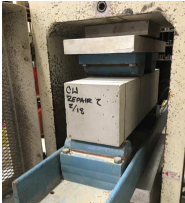
Figure 3.5 Modulus of Rupture Test Set-Up
