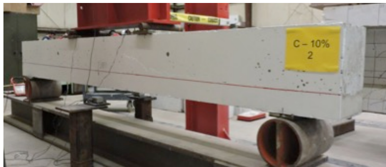
Figure 4.27 FR-SCC Repair Beam Test Set-Up
