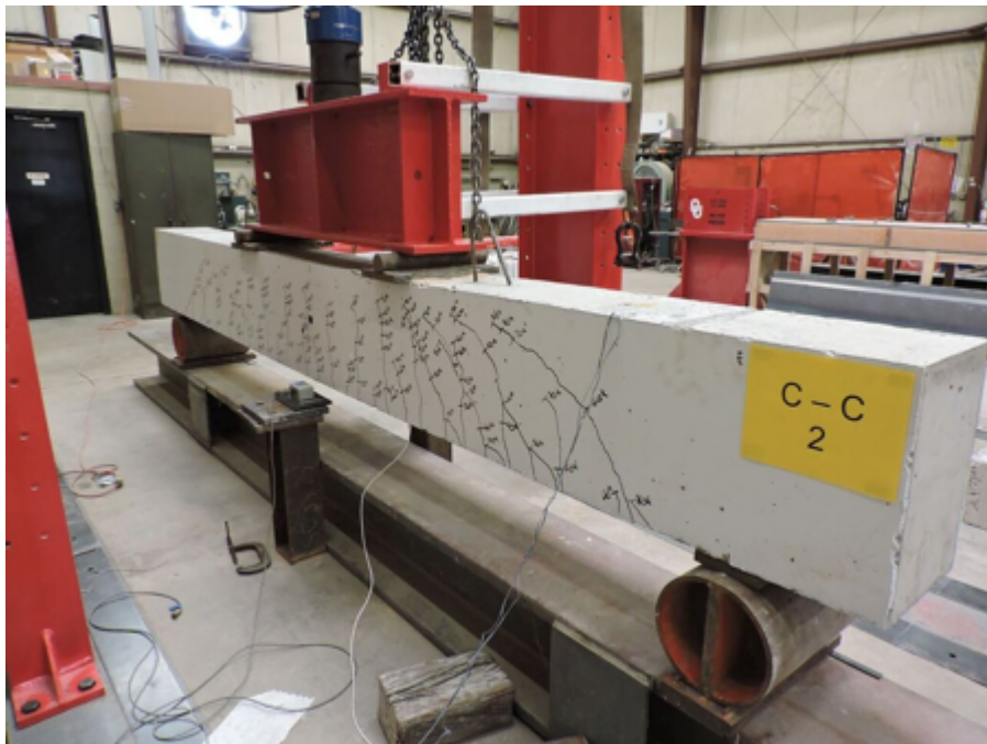
Figure C.2b C-C-2 at Failure
