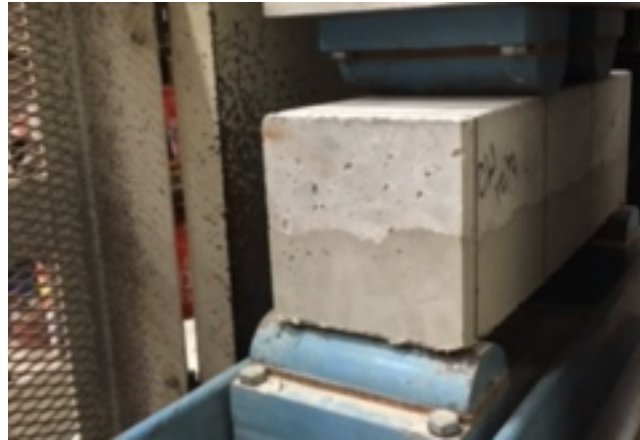
Figure 5.2 Composite Modulus of Rupture Test Set-Up
