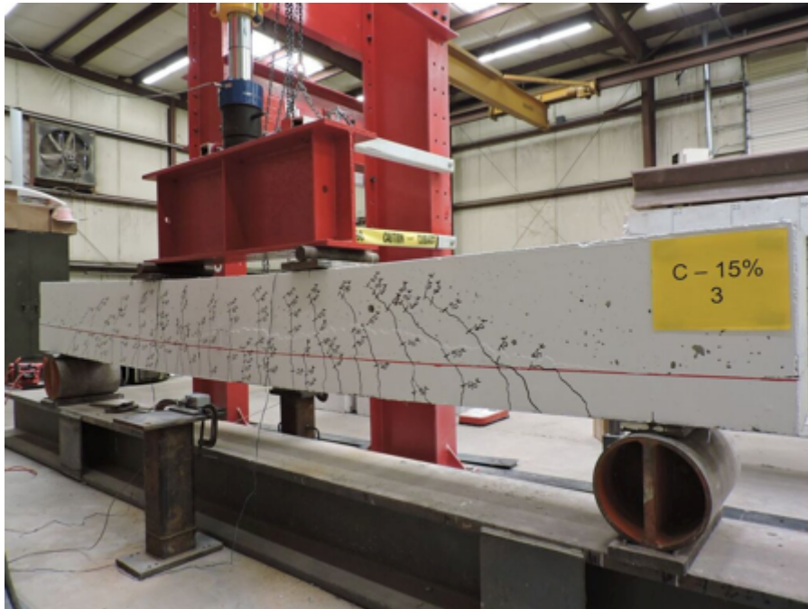
Figure C.9b C-15%-3 at Failure
