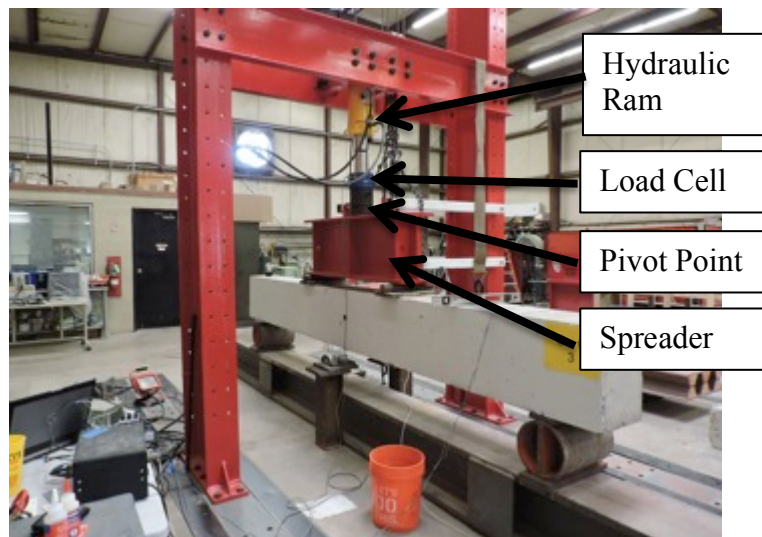
Figure 4.9 Control Beam Load Set-Up
