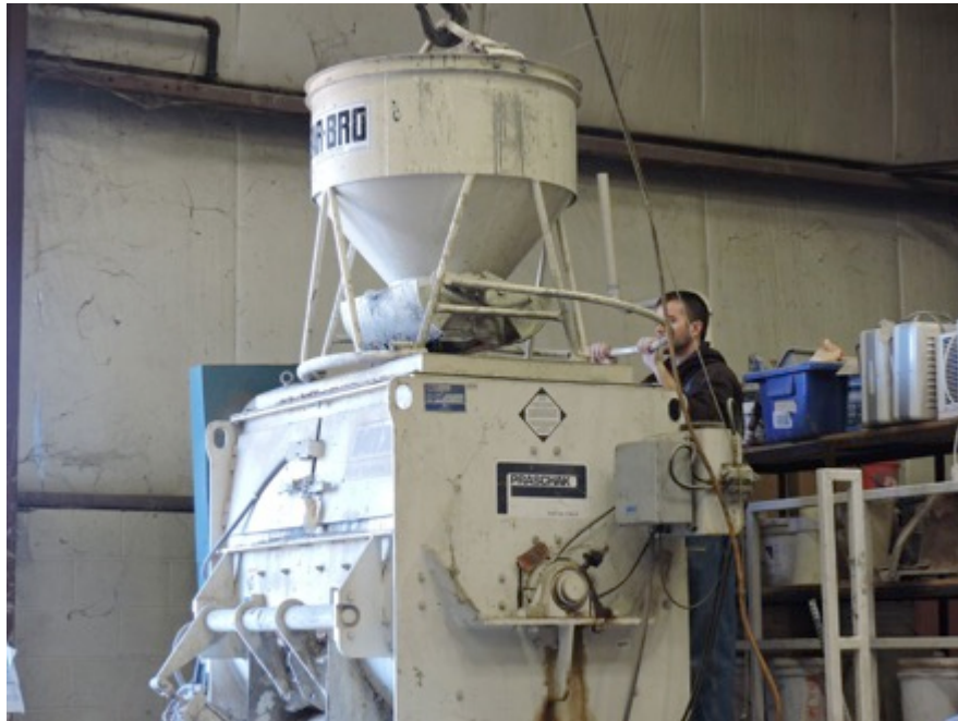
Figure 4.22 Overhead Crane Bucket Transporting Fine Aggregate
