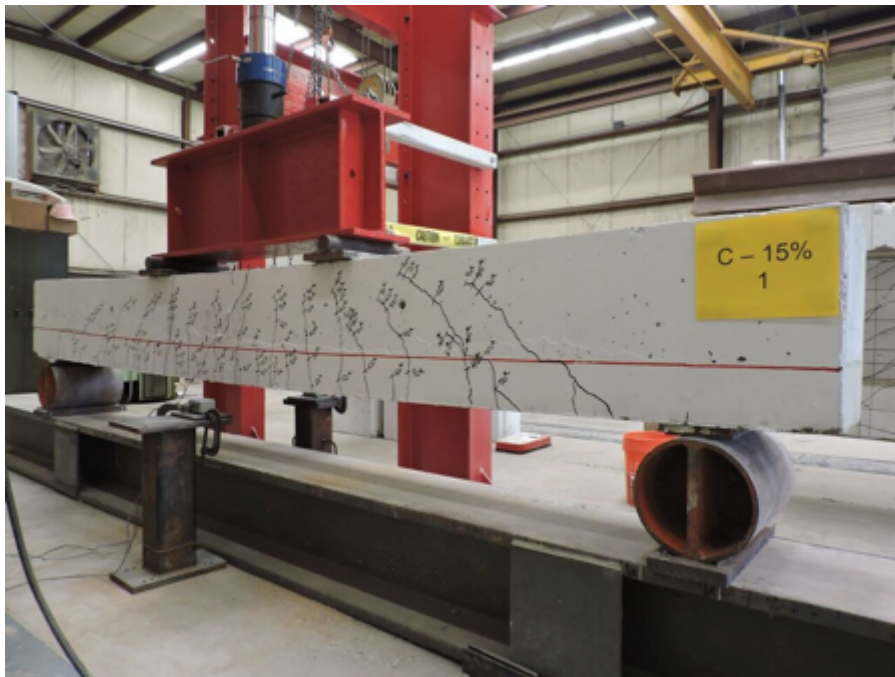
Figure C.7b C-15%-1 at Failure
