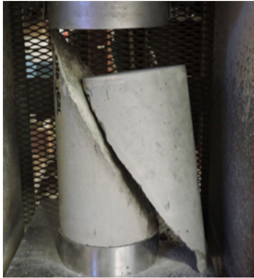
Figure 5.6 Typical Bond Strength Failure
