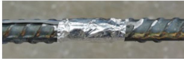
Figure 4.5 Wrapped Strain Gauge
