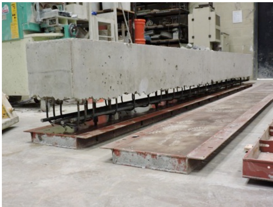
Figure 4.20 FR-SCC Repair Beam Placed on Form Bottom
