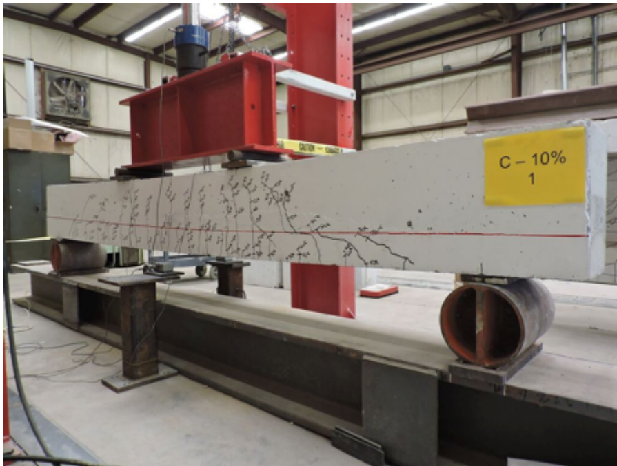
Figure C.4b C-10%-1 at Failure
