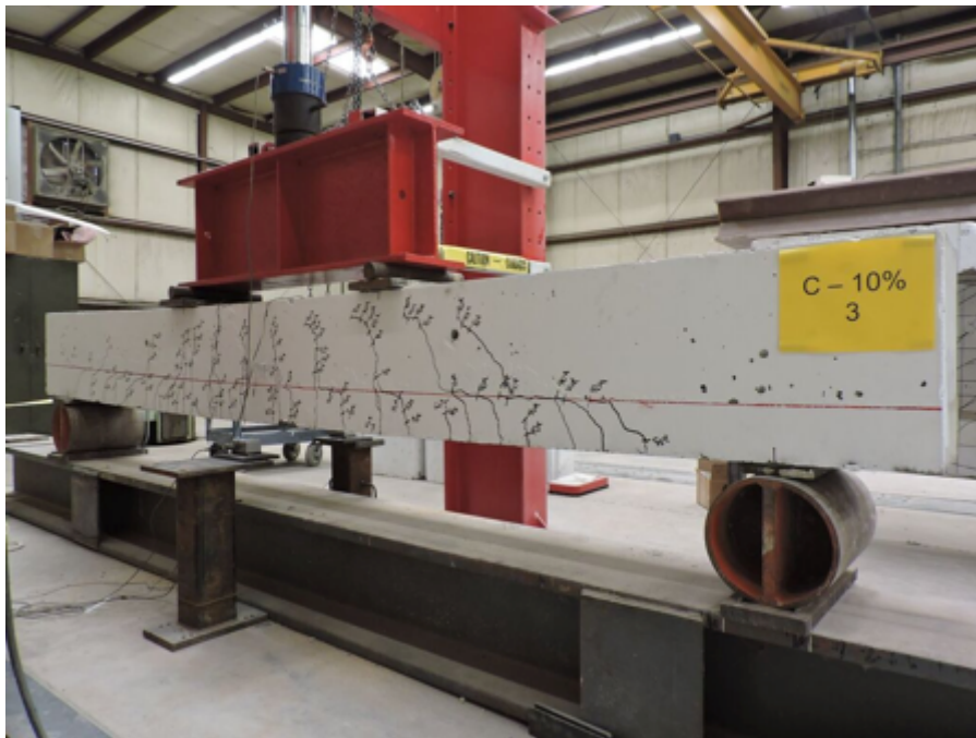
Figure C.6b C-10%-3 at Failure
