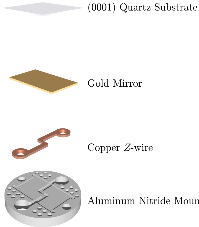
Figure 4.6: An exploded view of the quartz mount.
