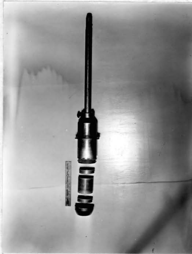
Figure 1. An exploded view of the Pomona soil sampler with the parts in their relative position.
