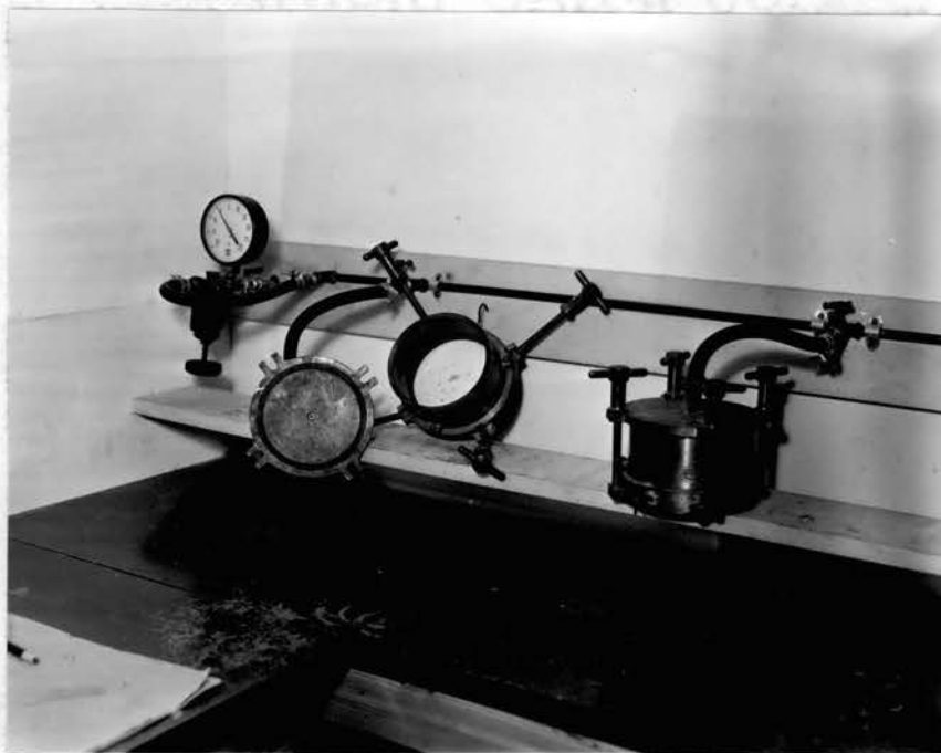
Figure 3. The panel arrangement of the porous ceramic plate apparatus and pressure regulator.
