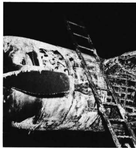
Fire trailed aft from the left engine, destroying the nacelle and wing.
