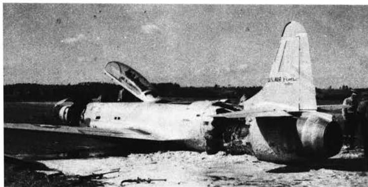
Mismanagement of the fuel system caused a flameout.
