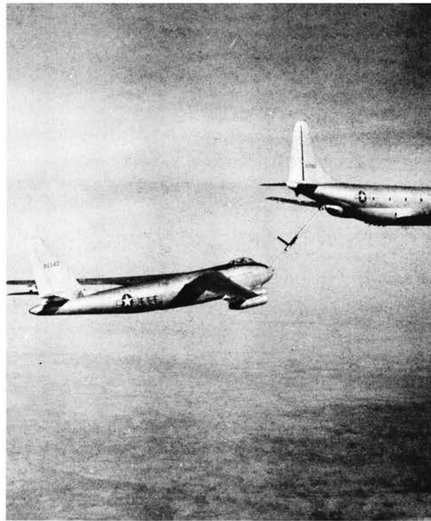
COMPRESSOR STALL is frequently experienced during air refueling and can result in a critical over-temperature condition.
