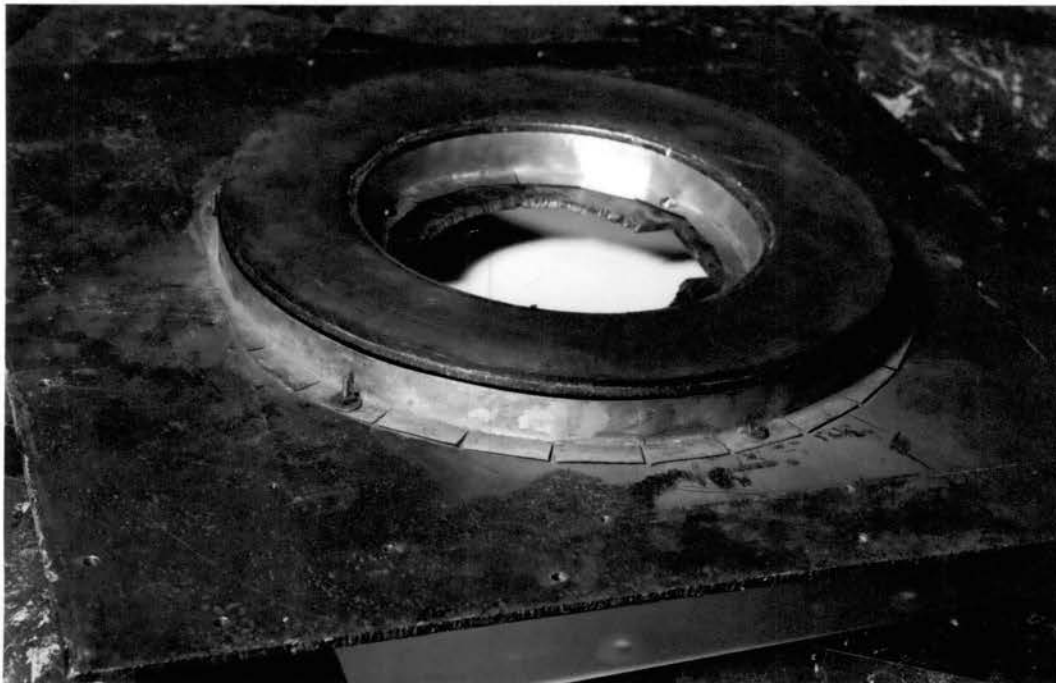
Figure 6. View of 18 Inch Diameter Stationary Disk Equipped With 1/4 Inch Thick Rubber Facing of Durometer Hardness No. 55 as Based on Company Specifications.
