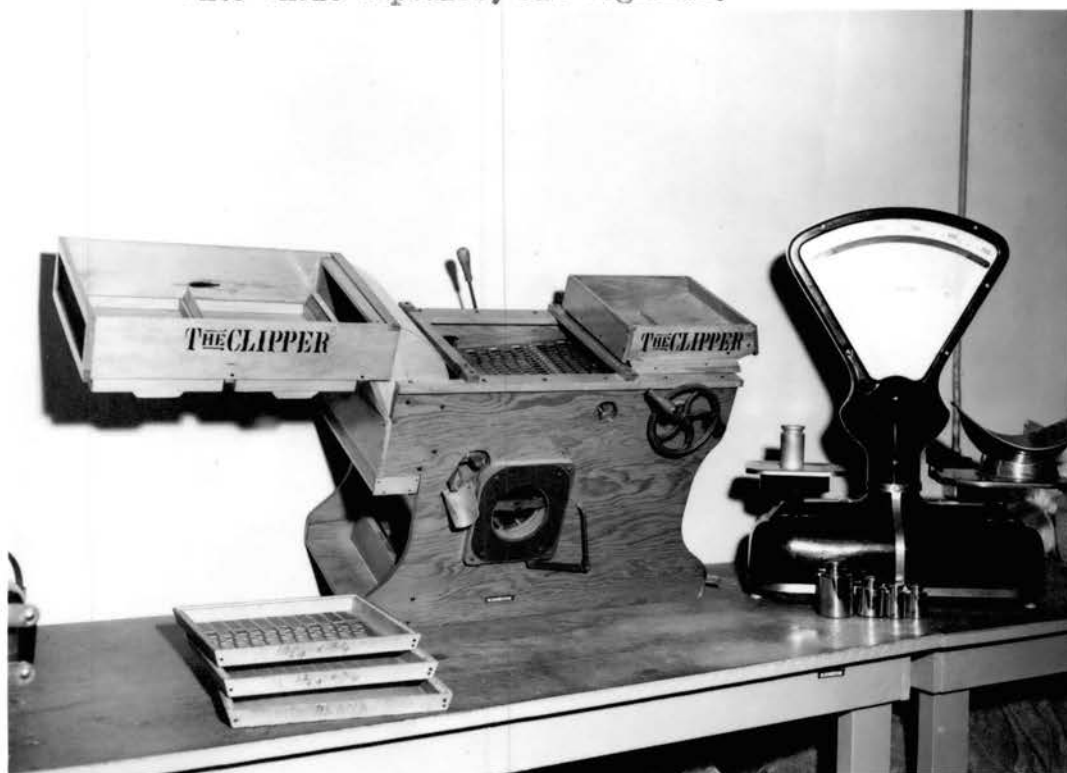
Figure 9. Sampling Apparatus Consisting of Toledo Scale Balance, Small Hand Clipper and 3 Separating Screens Used to Evaluate the Products in the Sack and in the Cleanings.
