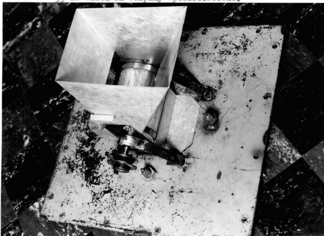
Figure 7. View of Rotating Drum Feeder and Two of the Four Adjusting Screws Used to Align the Disks.
