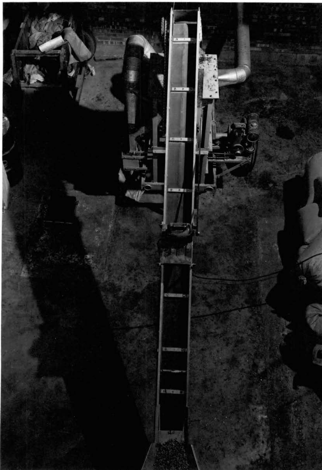
Figure 1. Top View of Complete Castor Bean Huller Unit Showing Position of Elevator as Used in Tests.
