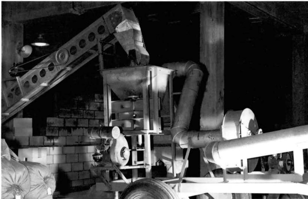
Figure 3. Left Side View of Castor Bean Huller Showing Position of Huller Engine and Handwheel Used to Adjust Spacing Between the Disks.
