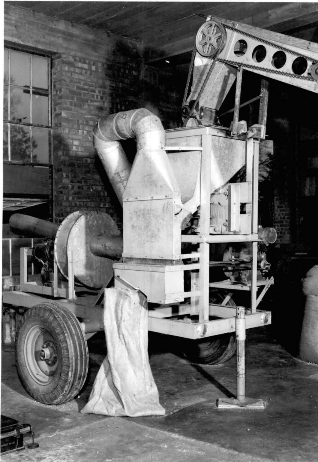
Figure 2. Right Side View of Castor Bean Huller Showing Arrangement of Rotating Drum Feeder, Cleaning Unit and Two Way Discharge Valve for Sacking.
