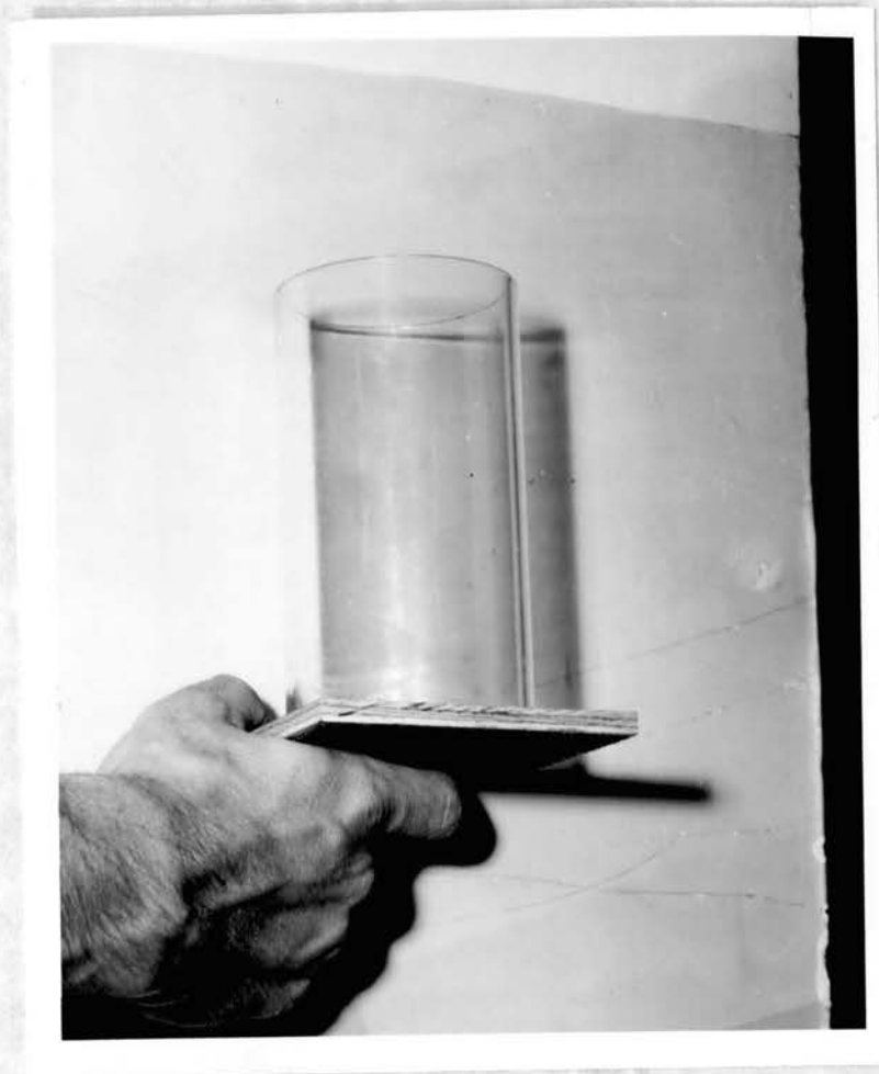
Fig. 3. Mounted lucite grain container for holding grain samples.
