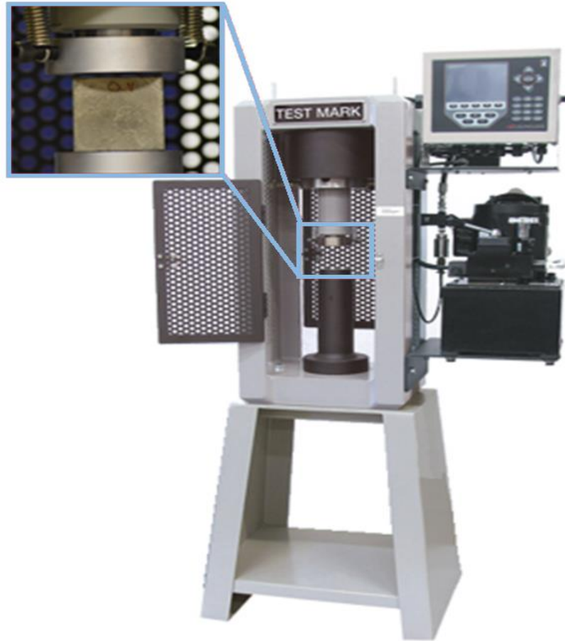
Figure 12 – Crush test apparatus for determining the UCS of target material
