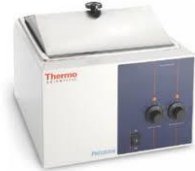
Figure 11 – Example of a thermally active aqueous curing environment
