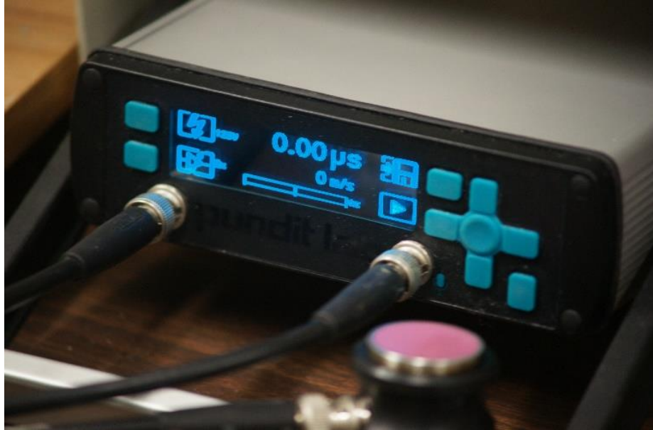
Figure 14 – UPV indicator screen connected to transducers
