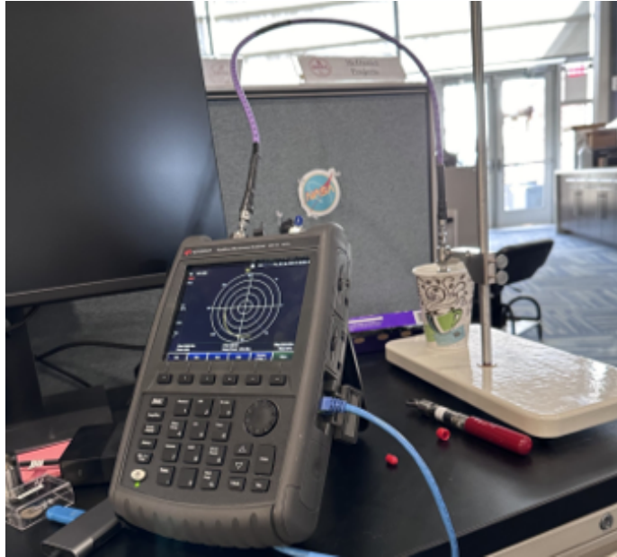
Figure 2.1: Measurement configuration for Keysight N1501A High Temperature Probe and Keysight Fieldfox
