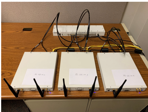
(a) Five-antenna transmitter with USRPs.
