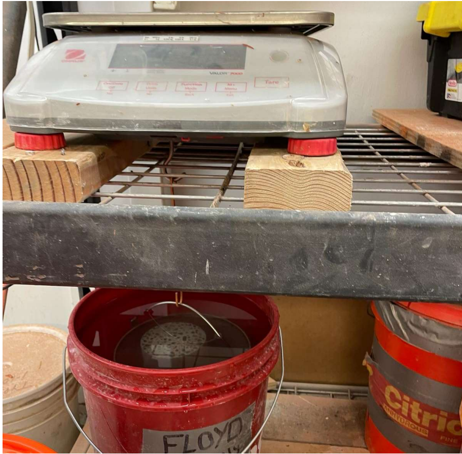
Figure 14 - Mechanism at Fears Lab to weight apparent mass of suspended-immersed cylinder.
