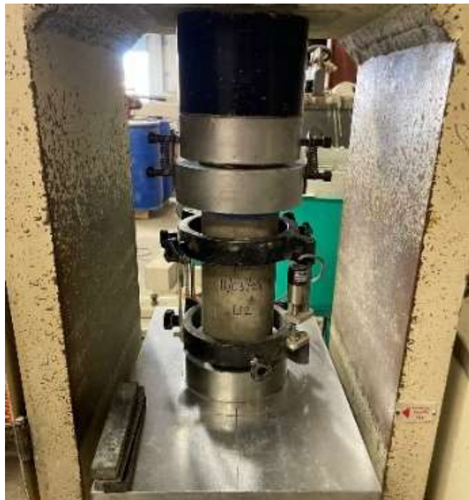
Figure 12 - Modulus of elasticity testing set-up.
