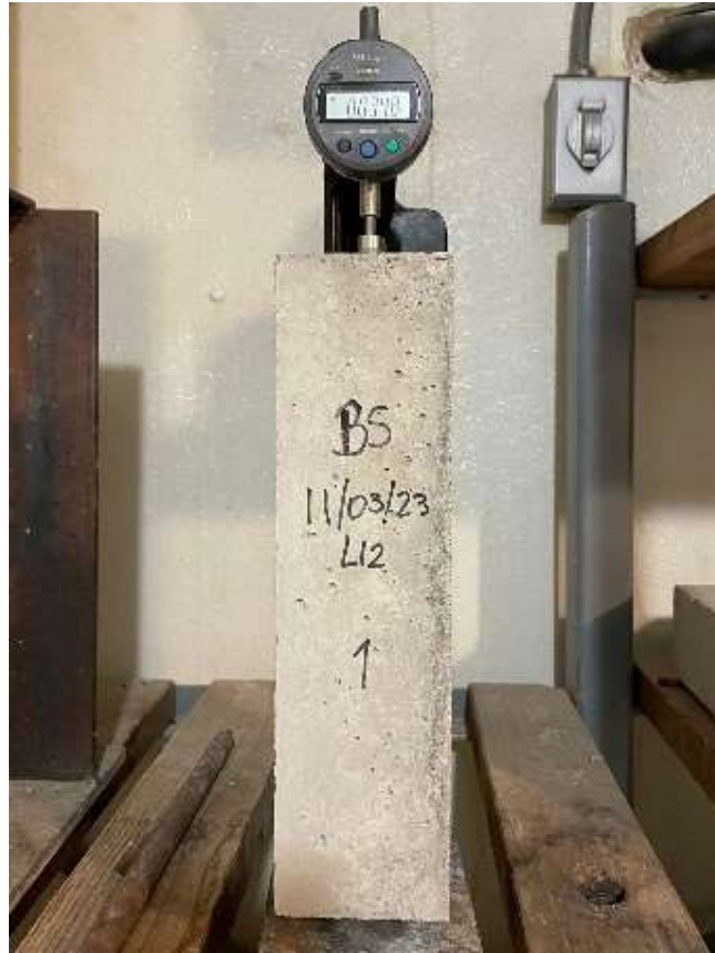
Figure 15 - Comparator testing set-up for shrinkage specimens.
