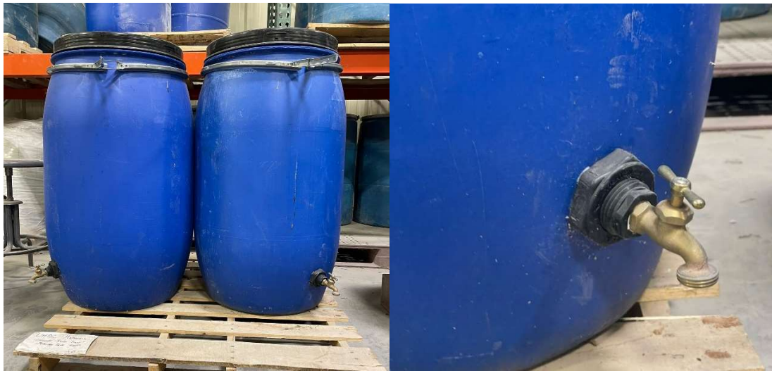
Figure 8 - Draining barrel mechanism for presoak of LWA.
