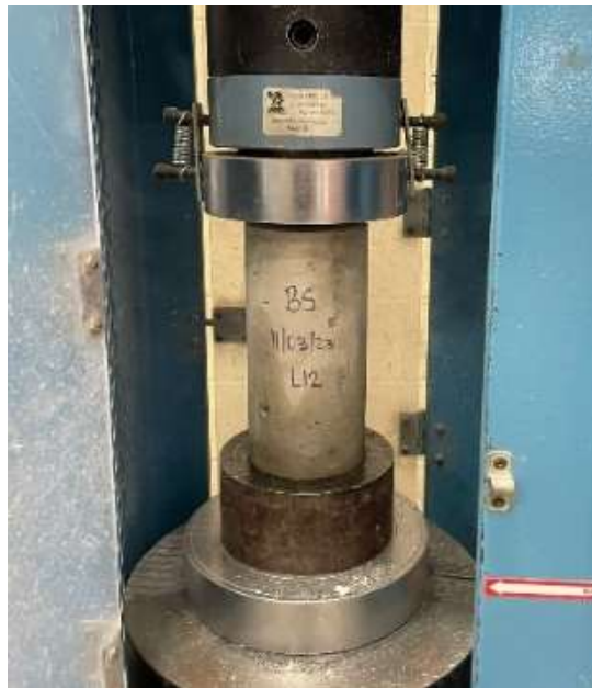
Figure 11 - Compressive strength testing
