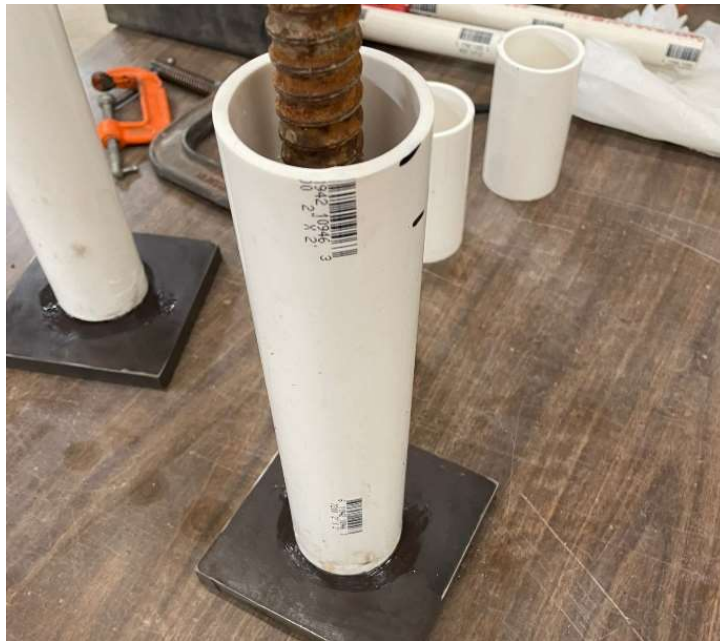
Figure 29 - Supports with steel base plate, bolt and nut and PVC fixed with silicone to the base plate.
