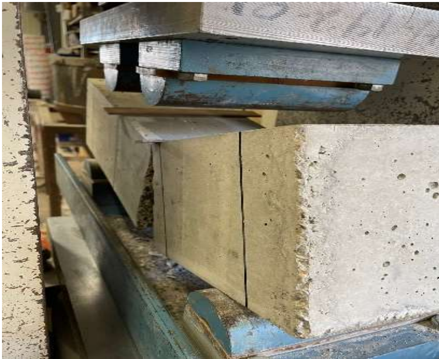
Figure 13 - Modulus of rupture test after failure of specimen.
