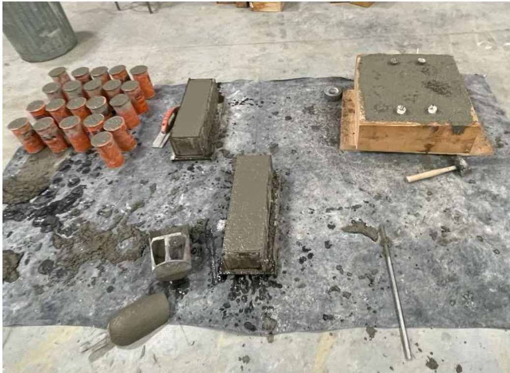
Figure 33 – Scaled slab immediately after demolding at seven days.
