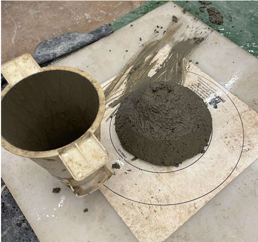
Figure 10 - Slump test performed at Fears Lab showing slump cone with an approximate slump of 7 in.
