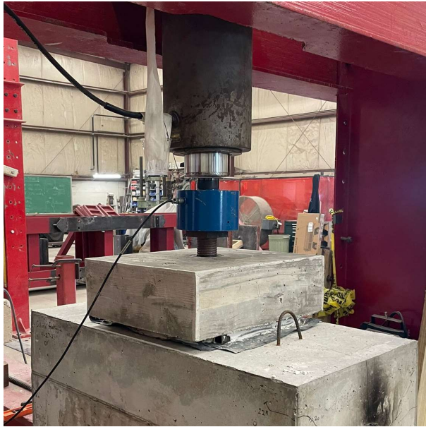
Figure 79 - Punching shear testing set-up for support B.
