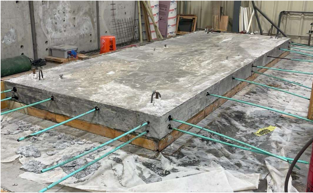
Figure 33 – Scaled slab immediately after demolding at seven days.
