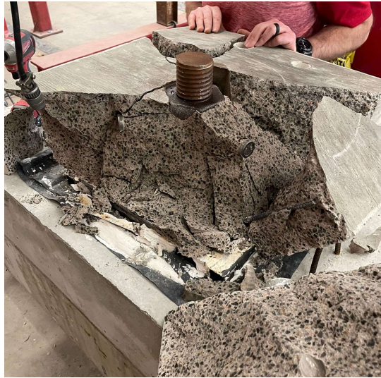
Figure 80 - Punching shear failure for support B test specimen.
