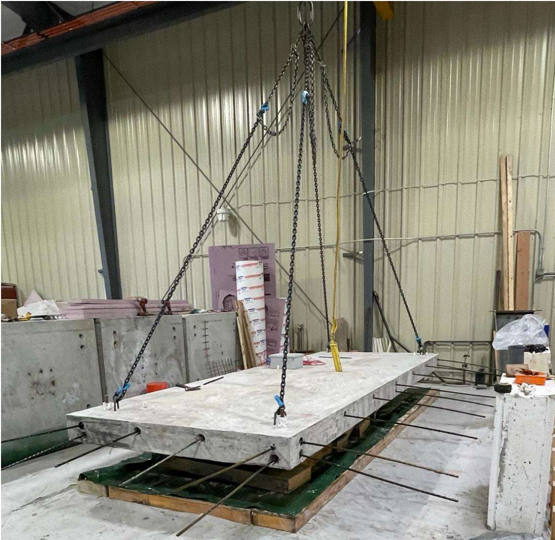
Figure 37 - Slab being pick up from four lifting hooks using overhead crane at Fears Lab.
