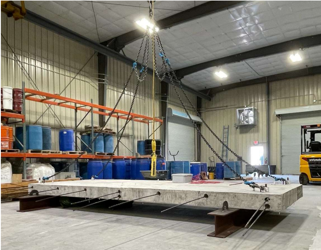
Figure 38 - Slab supported by steel W beams.
