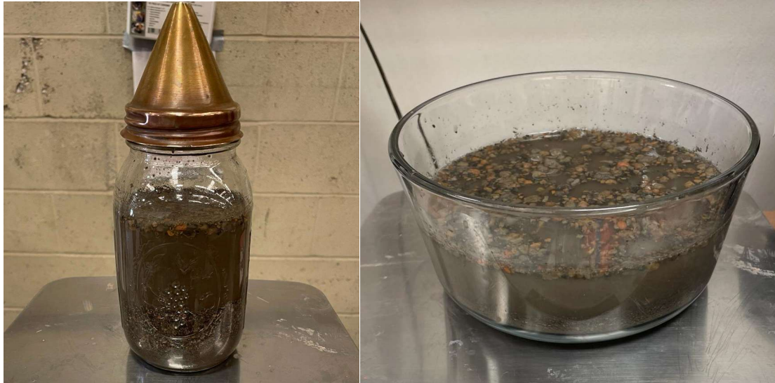
Figure 9 - Specific gravity test (left) and absorption test (right)
