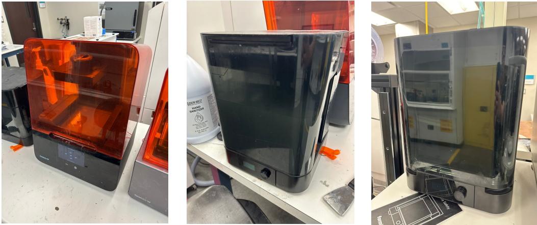
Figure 4.1: FormLabs additive manufacturing equipment. Form3 3D printer (left), Iso-propil alcohol cleaner (center) and UV light curing device (right).
