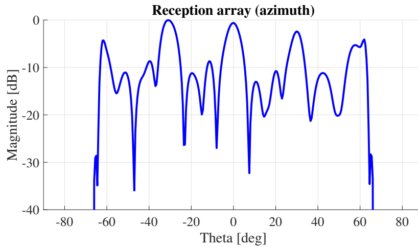
Figure 4.25: Measured azimuth radiation pattern of the reception antenna array with two-wavelength spacing. The data is truncated at \pm 70^\circ due to the maximum scan window in the chamber and the NSI 2000 software ( 5' \times 5' ).
