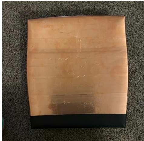
Figure 3.24: Second 3D printed reflector in the process of being coated with copper tape.
