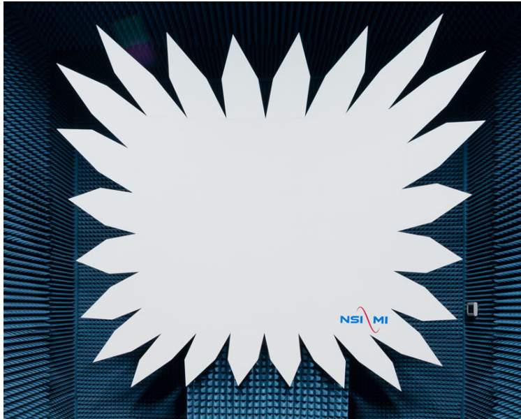
Figure 1.6: Example CATR reflector created by NSI-MI Technologies, an antenna metrology company [31]. Piece-wise petal-shaped serrations are used.
