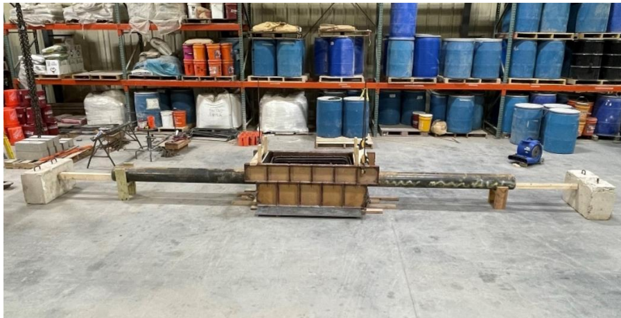
Figure 18. Complete formwork of a small-scale HC-FCS column connection specimen
