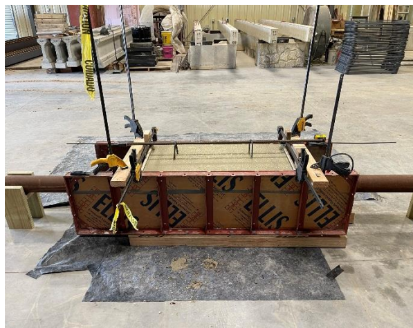
Figure 12. Trial specimen before removing the formwork
