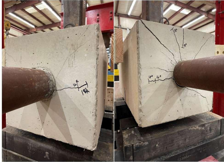
Figure 14. Pullout connection failure from each end of the footing
