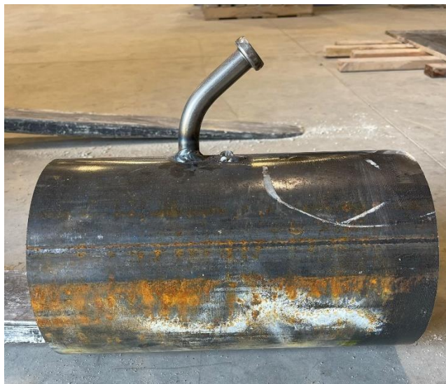
Figure 20. Result of stud bending test
