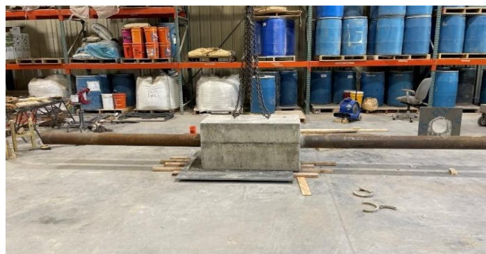
Figure 19. Column footing specimen 1 at 7 days of age
