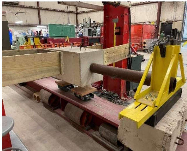
Figure 13. Testing setup for the trial footing-column connection specimen
