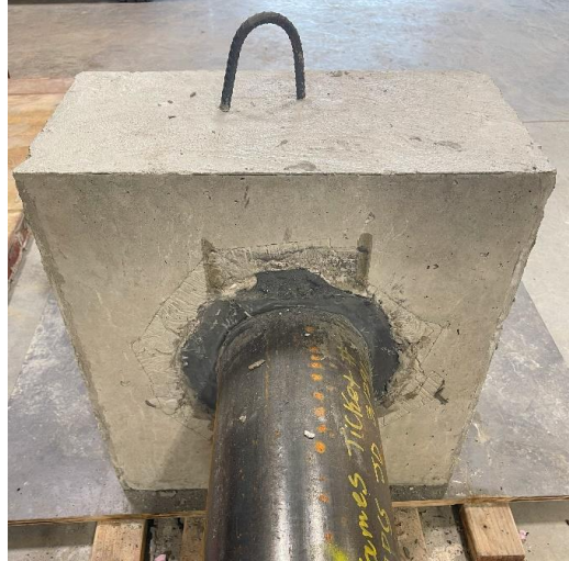
Figure 25. Complete trial socketed connection specimen
