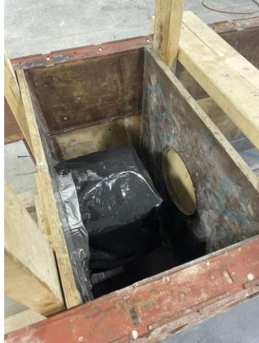
Figure 23. CSP covered in plastic sheeting inside formwork for socketed trial specimen 2
