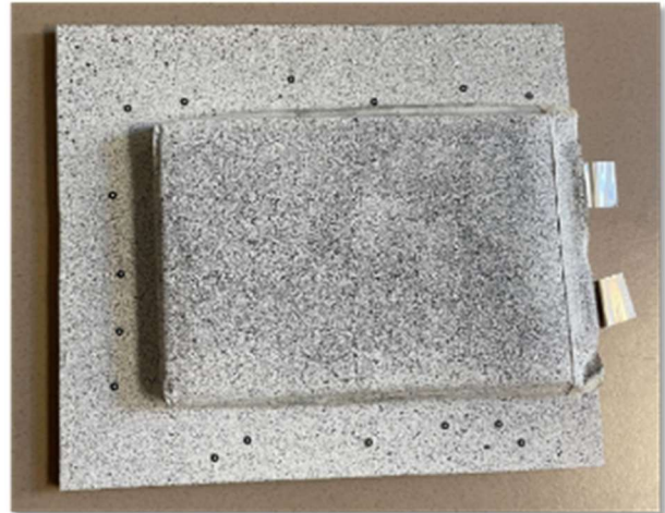
Figure 4: Battery 1 Glued to Plates with Speckle Pattern and Reference Dot Stickers
