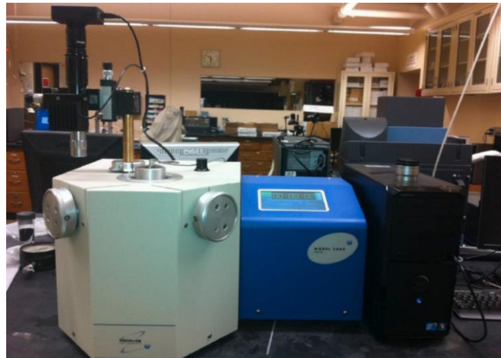
Figure 28. Model 1060 Fischione broad beam argon mill used for final polishing sample surface prior to SEM imaging.
