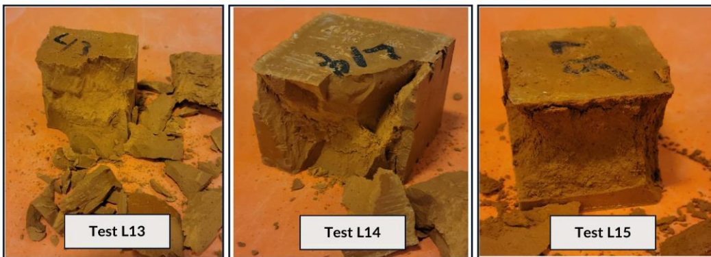
Figure C-15: Images of 28-day Ambient Curing for Tests L13-L15
