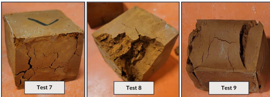
Figure C-6: Images of Oven Curing for Tests 7-9
