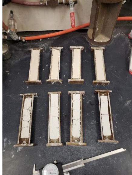
Figure 5. Oven-dried specimens for the bar linear shrinkage.
