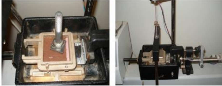
Figure 5: Setup for interface shear tests by Esmaili (2014)
