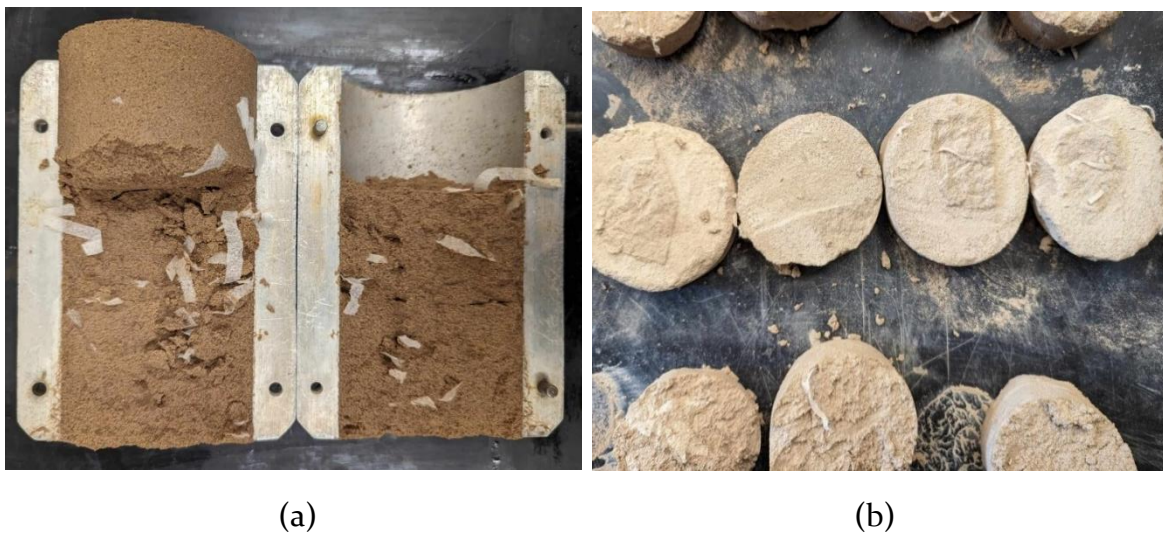
Figure 27: Dissected FRS specimens (a) FM-D50-Co.8 (discarded, not tested), (b) FM-C25-Co.8 and FM-C25-C1.2 after triaxial tests
