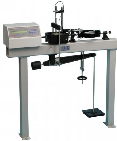
Figure 15: Direct/Residual Shear Test Set used in the study
