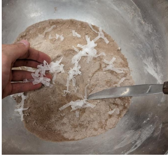
Figure 23: Manual mix of soil and fiber strips
