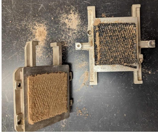
Figure 13: Interface shear test load cell with geotextile after test
