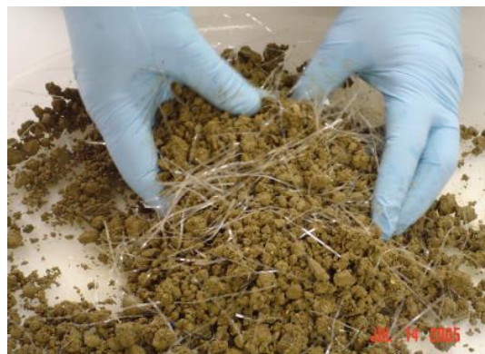
Figure 4: Mixing of polymer fibers and soil to prepare individual FRS specimens (Gregory 2006)
