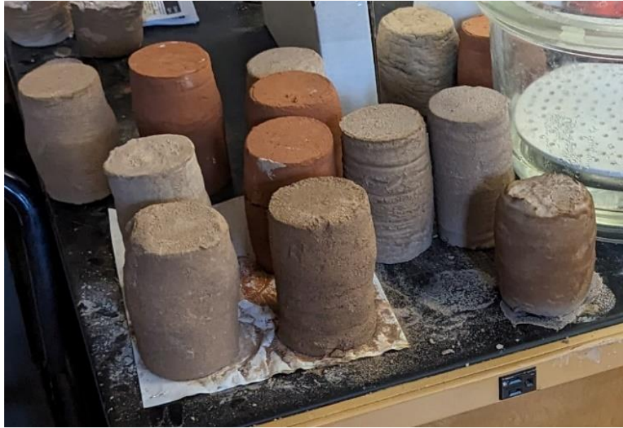
Figure 18: Preliminary test specimens after triaxial testing
