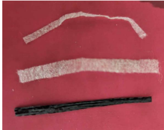
Figure 17: From top to bottom, facemask fibers of 2.5 x 51 mm, 5.1 x 51 mm and geotextile fibers of 2.5 x 51 mm
