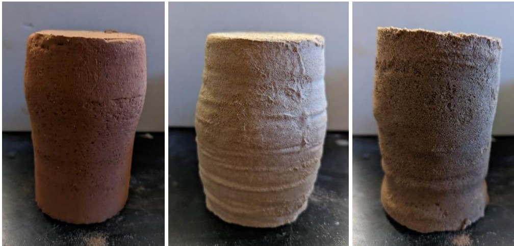
Figure 19: Clay, 30% Limestone Sand, and 20% Limestone Sand specimens after triaxial tests
