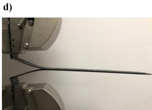
Figure 20: (a) Stress-strain relationship, (b) mean interfacial adhesion strength, (c) peel interface, (d) specimen during testing, and (e) specimen after failure for neat, pristine 1%, and functionalized 1% CFRP cured at room temperature.
