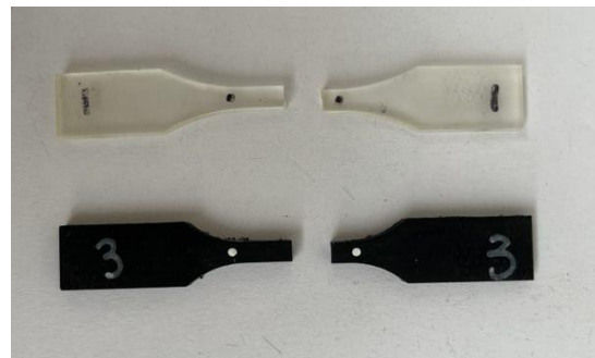
Figure 17: Representative neat (top) and nanomodified (bottom) epoxy resin specimens after tensile testing.
