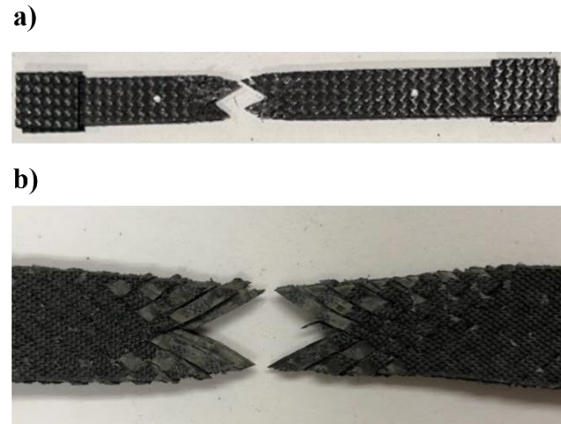
Figure 19: (a) Representative CFRP tensile specimen after failure; (b) Failure mode of CFRP tensile specimen.
