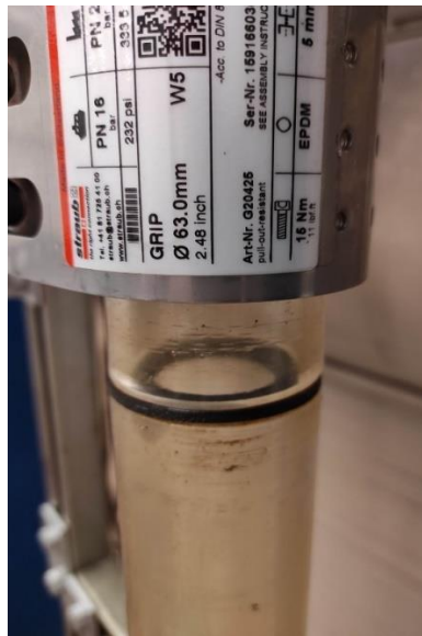
Figure 3.3 Insert installed between two pipes in the test section with Straub clamp unadjusted
