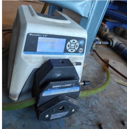
Figure 3.4 Peristaltic pump used to flow liquid into the test section
