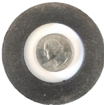
Figure 3.1 An insert used as a partial restriction, with a coin for size reference
