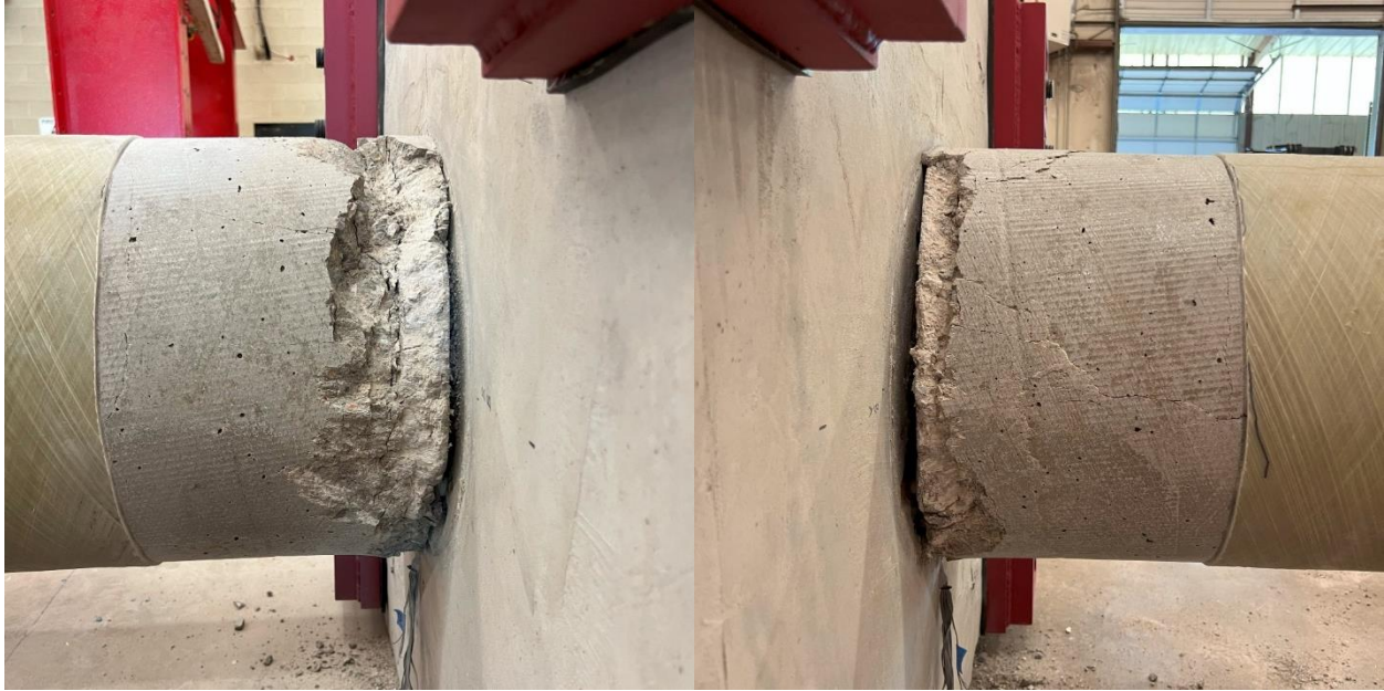
Figure 6-14: HS-SCC 1 Concrete Core After Testing and Light Removal of Concrete
