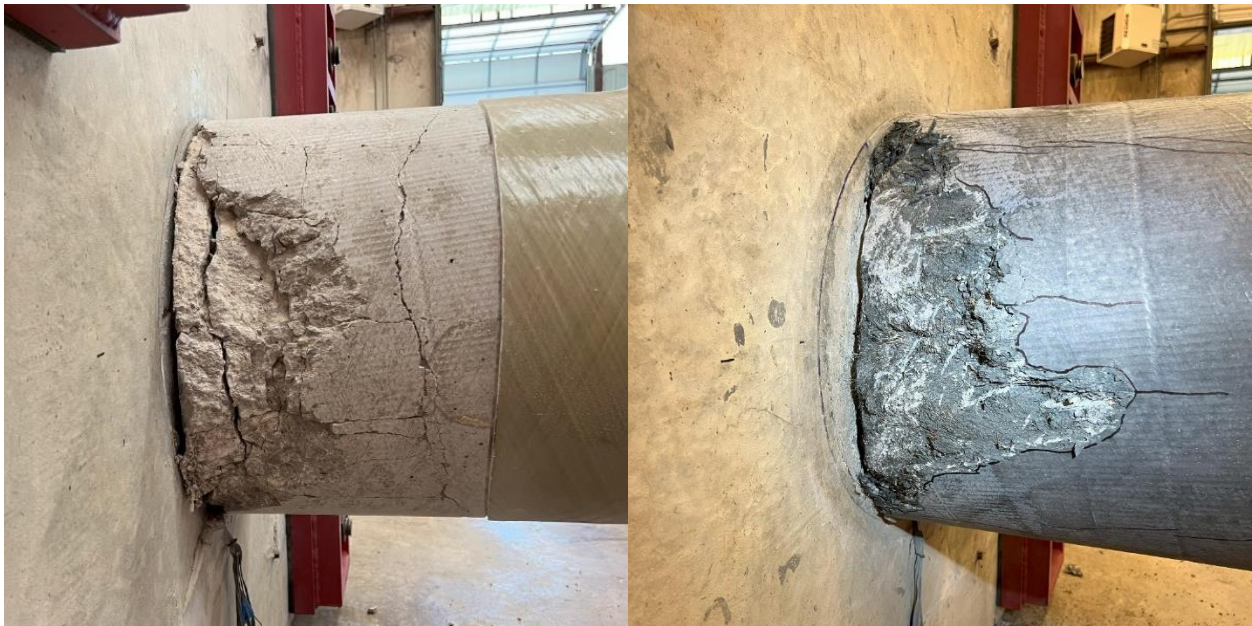
Figure 8-13: Comparing HS-SCC 2 (l) and UHPC 2 (r) Concrete Core East Side After Testing and Light Removal of Concrete
