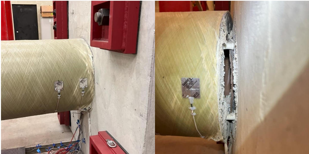
Figure 6-12: HS-SCC 1 GFRP Tube Compression (l) and Fractured Steel Tube (r) During Testing
