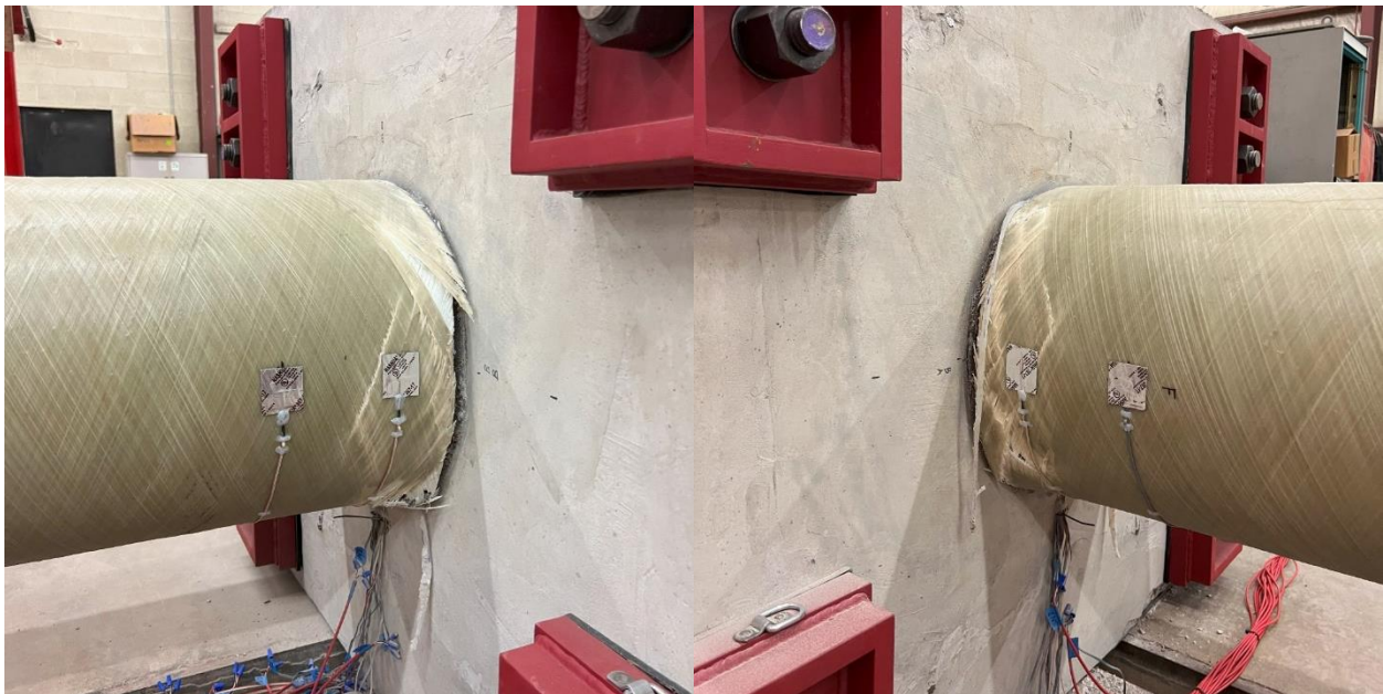
Figure 6-13: HS-SCC 1 GFRP Tube West Side (l) and East Side (r) Damage After Testing
