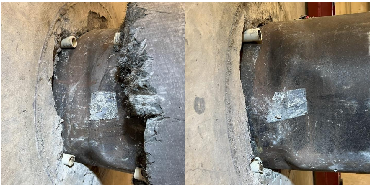
Figure 7-40: Comparing UHPC 1 (l) and UHPC 2 (r) Steel Tube Damage After Testing
