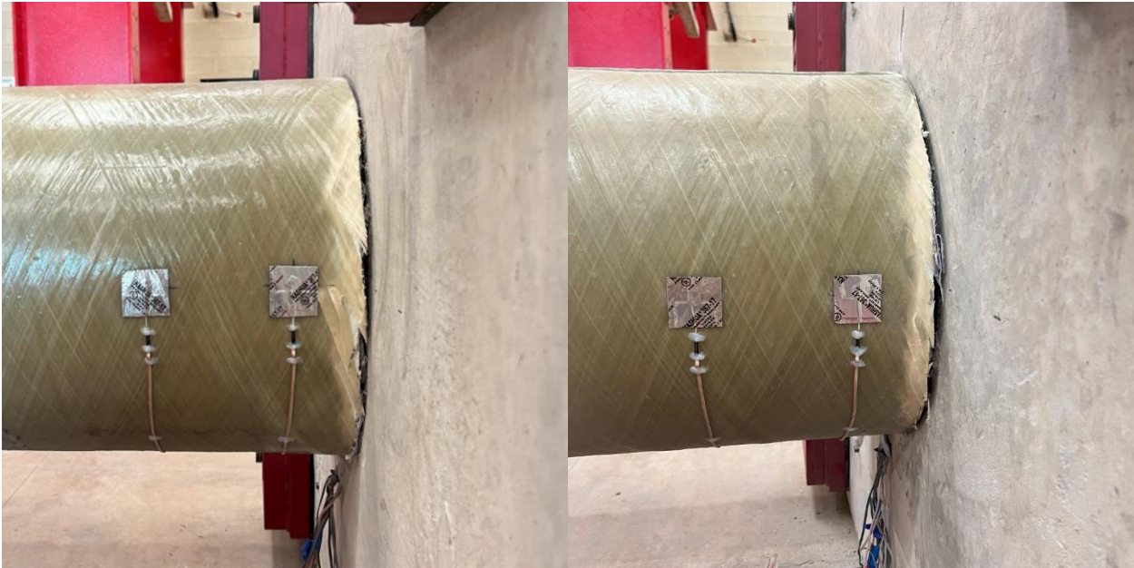
Figure 8-10: Comparing HS-SCC 2 (l) and UHPC 2 (r) GFRP Tube West Side After Testing
