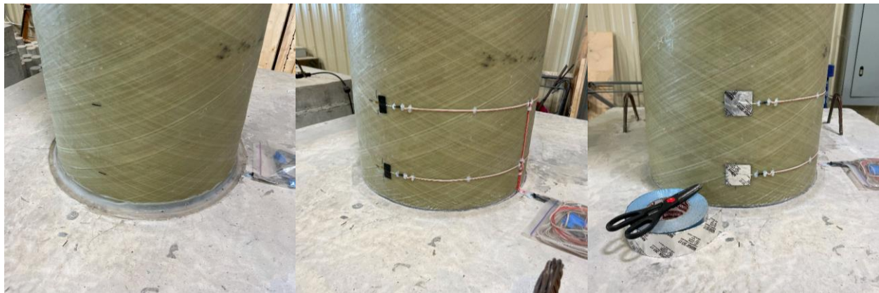
Figure 4-31: HC-FCS Column Application of External GFRP Instrumentation
