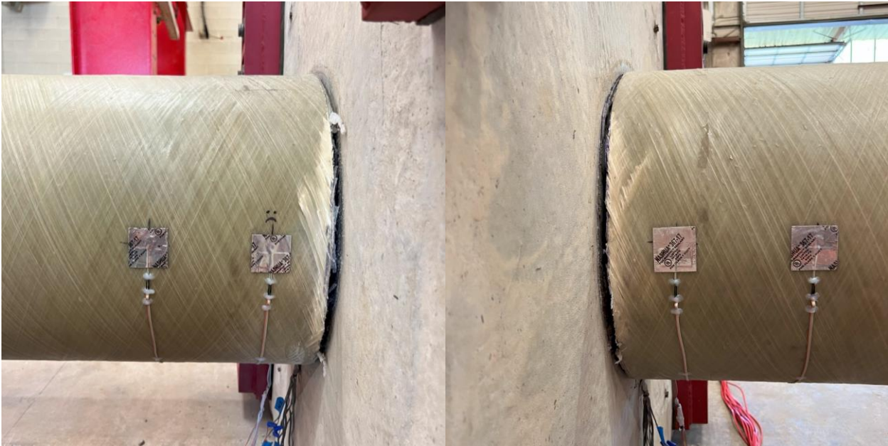
Figure 5-32: UHPC 1 GFRP Tube West Side (l) and East Side (r) Damage After Testing
