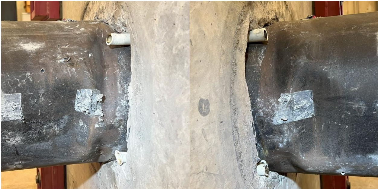
Figure 7-32: UHPC 2 Steel Tube West (l) and East Side (r) Damage After Testing
