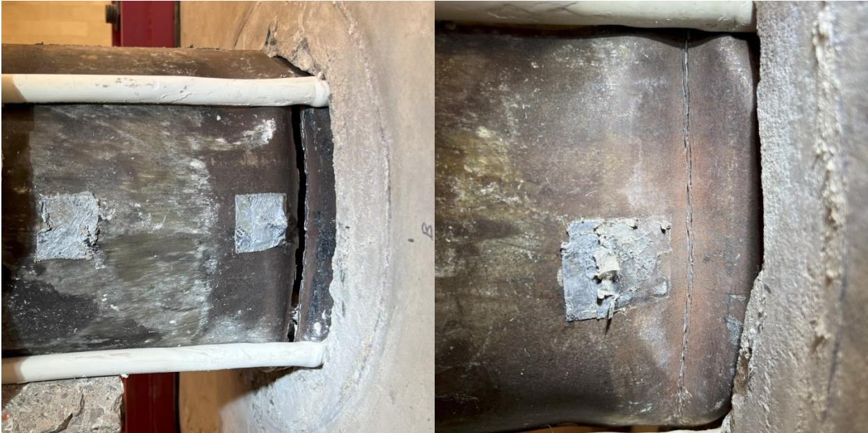
Figure 6-34: Comparing HS-SCC 1 (l) and HS-SCC 2 (r) Steel Tube Damage After Testing
