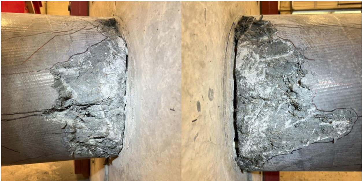
Figure 5-43: UHPC 2 Concrete Core After Testing and Light Concrete Removal
