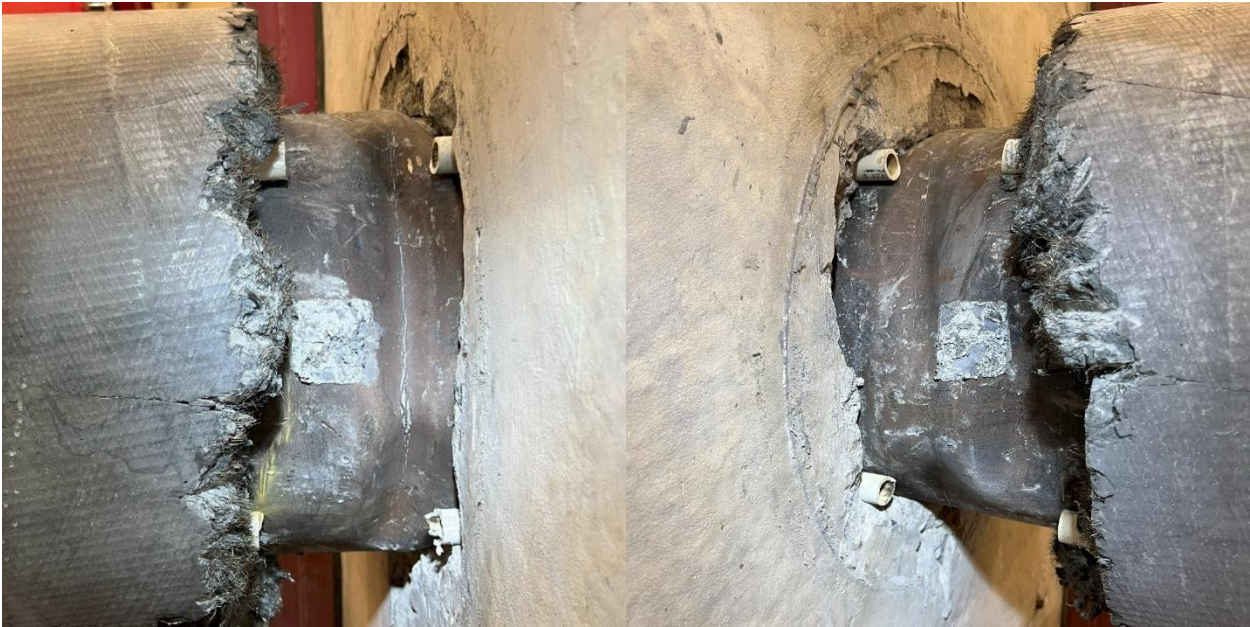
Figure 7-14: UHPC 1 Steel Tube West (l) and East Side (r) Damage After Testing
