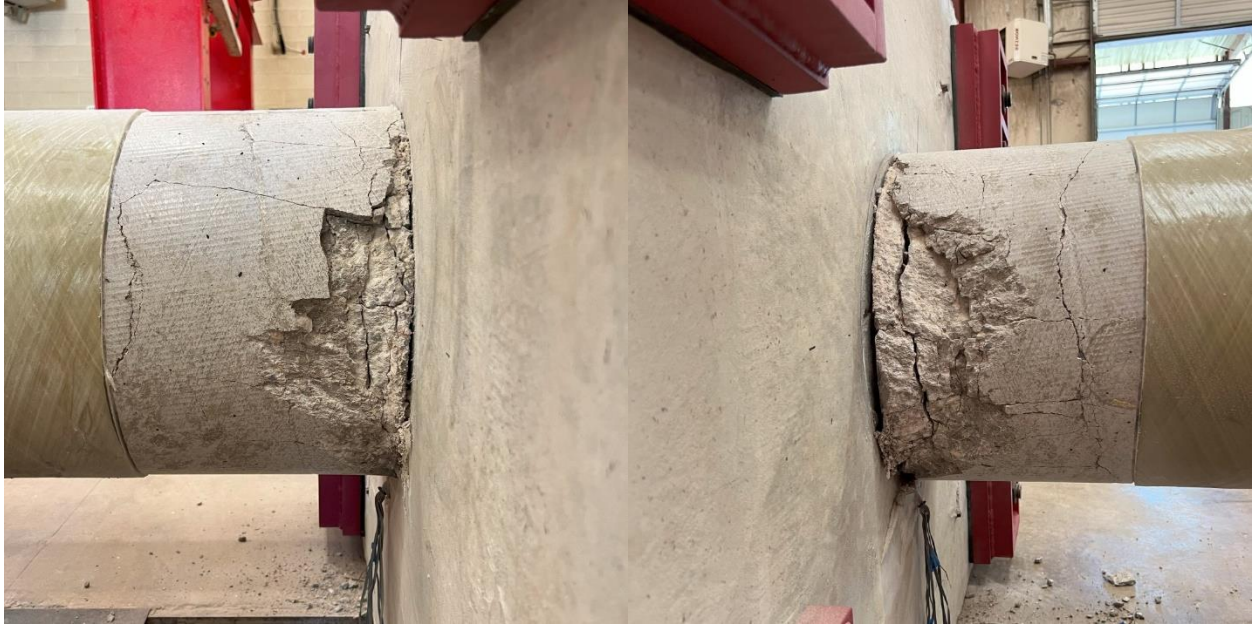
Figure 6-26: HS-SCC 2 Concrete Core After Testing and Light Removal of Concrete
