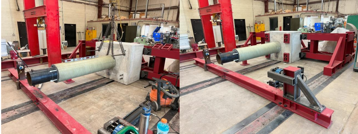
Figure 4-34: Column Specimen Placement and Fixation to the Testing Frame
