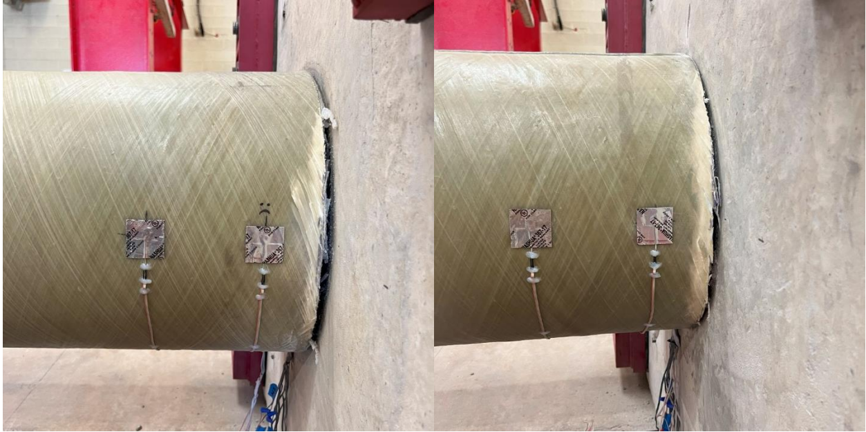
Figure 7-37: Comparing UHPC 1 (l) and UHPC 2 (r) GFRP Tube Damage After Testing
