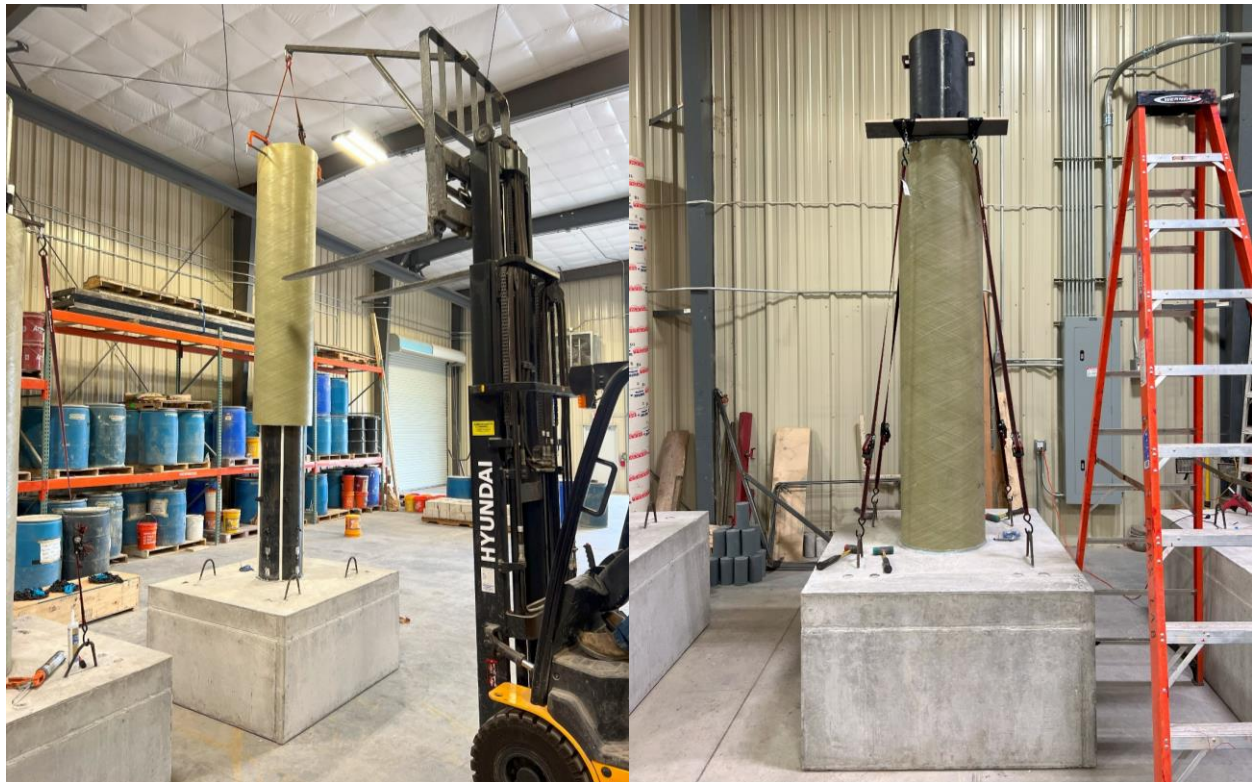
Figure 4-27: HC-FCS Column GFRP Placement and Specimen Ready for Casting
