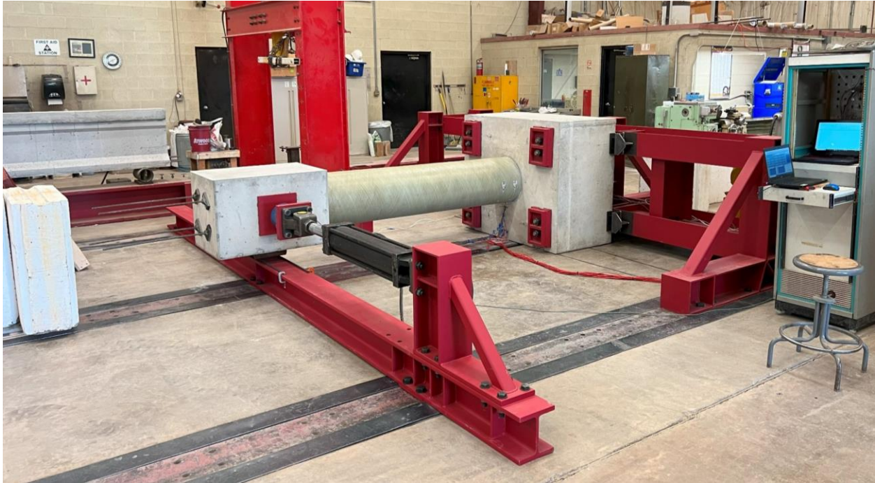
Figure 5-12: HS-SCC 1 Column Specimen Before Testing
