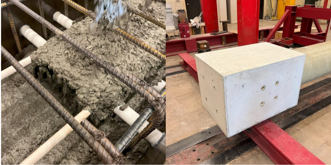
Figure 4-39: Column Cap During Casting and Completed and Ready for Testing
