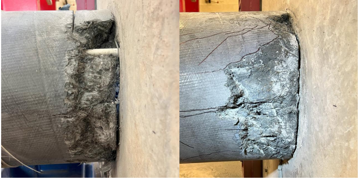
Figure 7-39: Comparing UHPC 1 (l) and UHPC 2 (r) Concrete Core After Testing and Light Removal of Concrete
