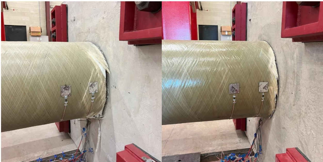
Figure 6-32: Comparing HS-SCC 1 (l) and HS-SCC 2 (r) GFRP Tube Damage After Testing
