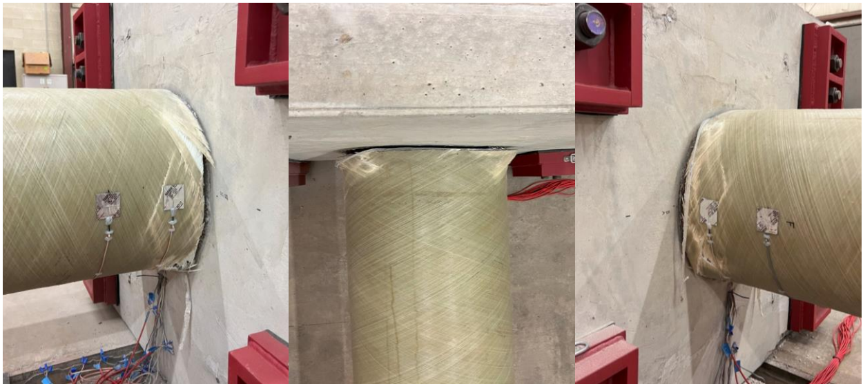
Figure 5-15: HS-SCC 1 GFRP Tube West (l), Top (m), and East Side (r) Damage After Testing
