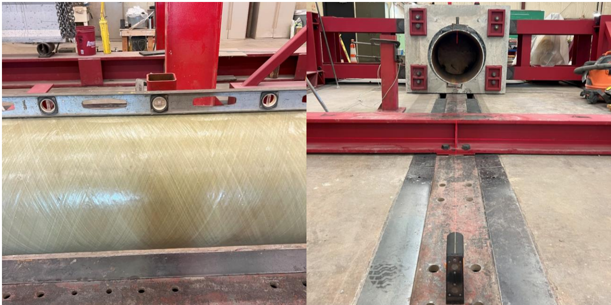
Figure 4-35: Specimen Alignment Checks, Checking for Level (l), Checking for Square (r)
