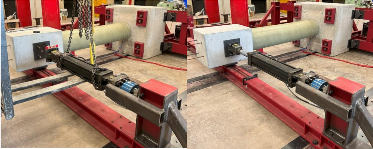
Figure 4-40: Attachment of Loading System Assembly
