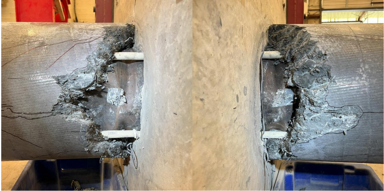
Figure 7-30: UHPC 2 Concrete Core After Testing and Significant Concrete Removal
