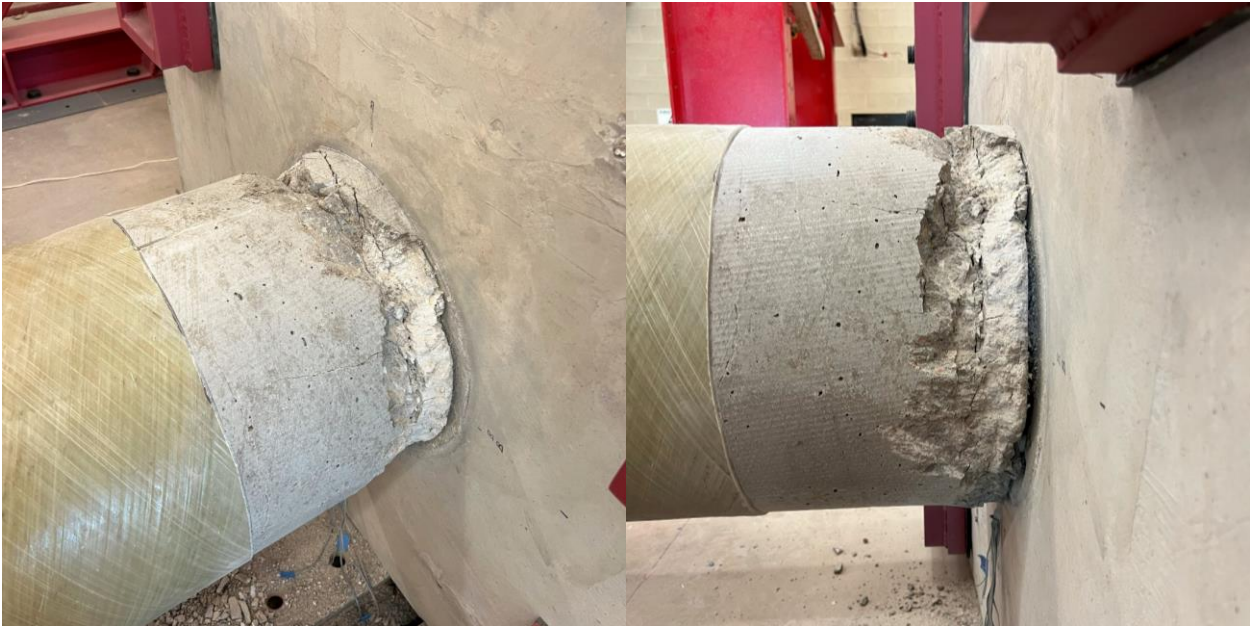
Figure 5-16: HS-SCC 1 Concrete Core After Testing and Light Removal of Concrete
