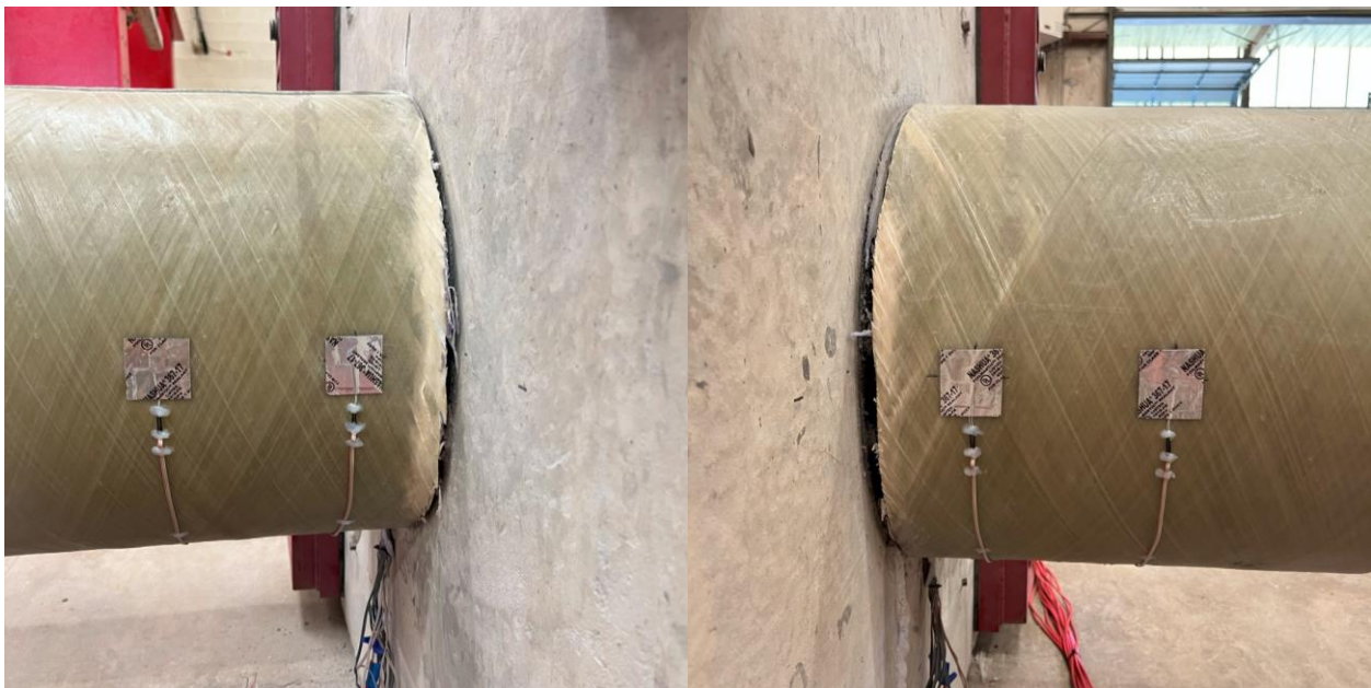
Figure 5-41: UHPC 2 GFRP Tube West Side (l) and East Side (r) Damage After Testing
