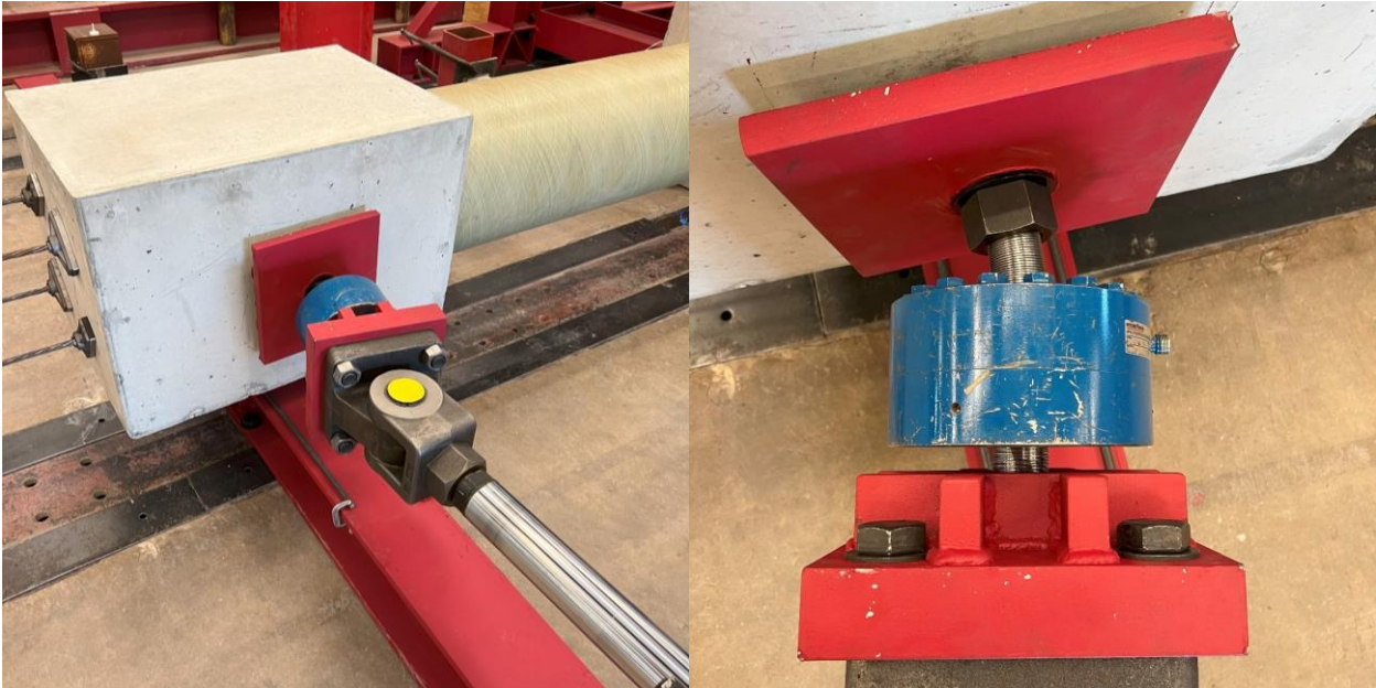
Figure 5-3: Buckling Failure of Original Loading System
