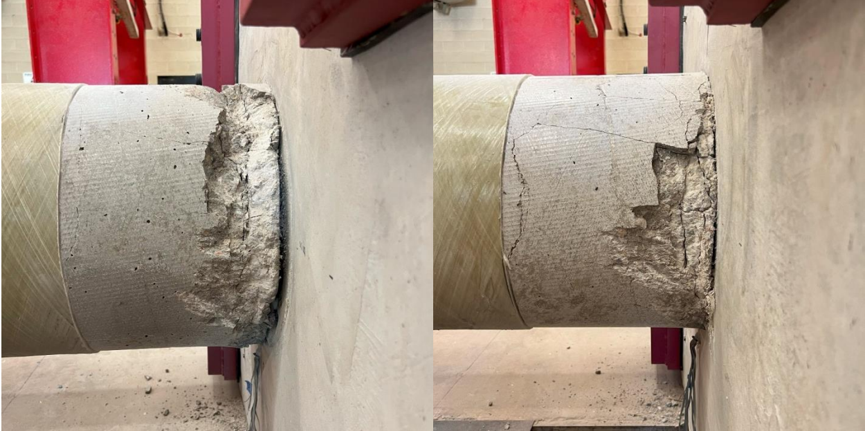
Figure 6-33: Comparing HS-SCC 1 (l) and HS-SCC 2 (r) Concrete Core After Testing and Light Removal of Concrete
