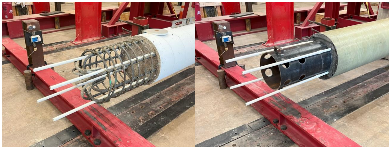
Figure 4-37: Column Specimens Before Column Cap Addition, RC (l) and HC-FCS (r)
