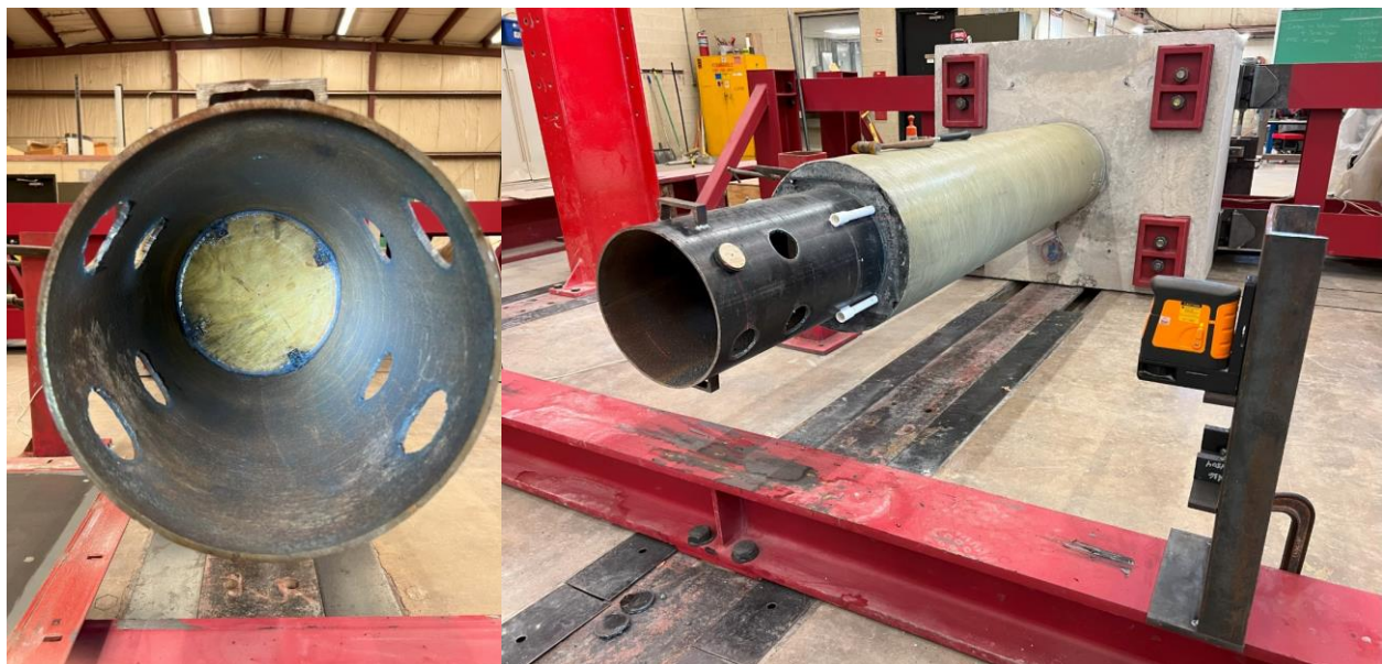
Figure 4-36: HC-FCS Column Cap Preparation, Plug Installation (l) and Laser and Jig Used to Determine Through-Hole Locations (r)
