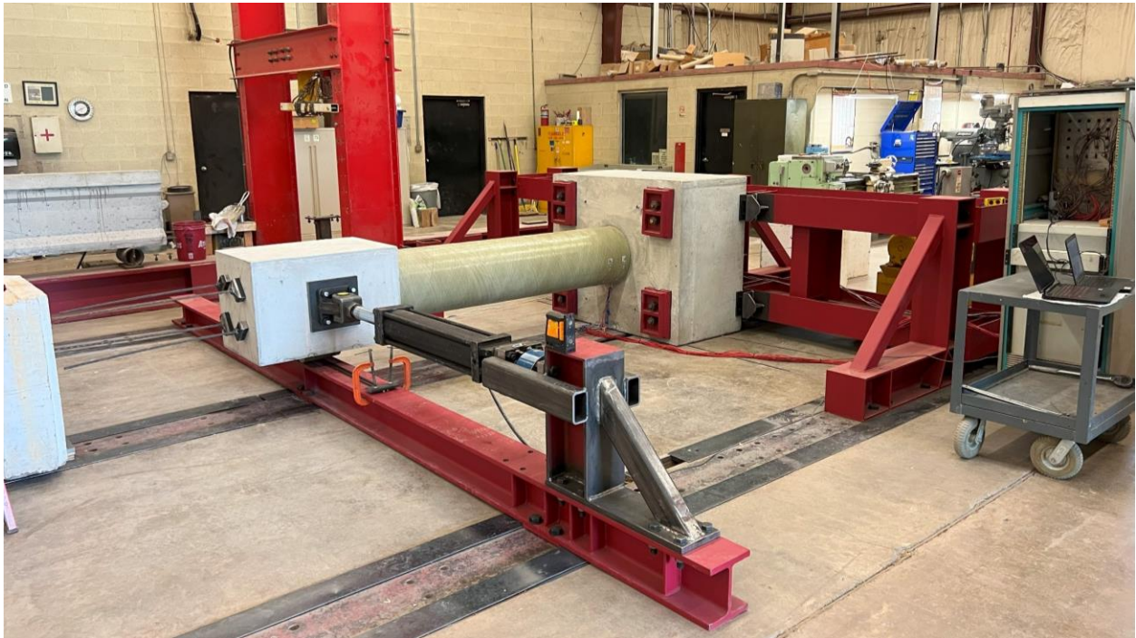
Figure 5-22: HS-SCC 2 Column Specimen Before Testing
