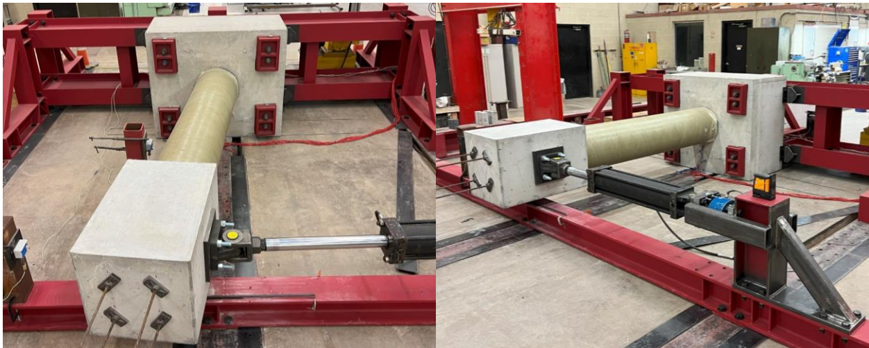
Figure 5-13: HS-SCC 1 Column Specimen During (l) and After Testing (r)
