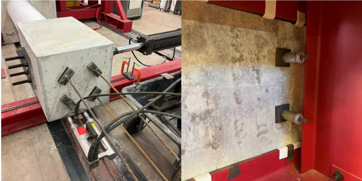
Figure 4-41: Constant Axial Load Application Utilizing Post-Tensioning
