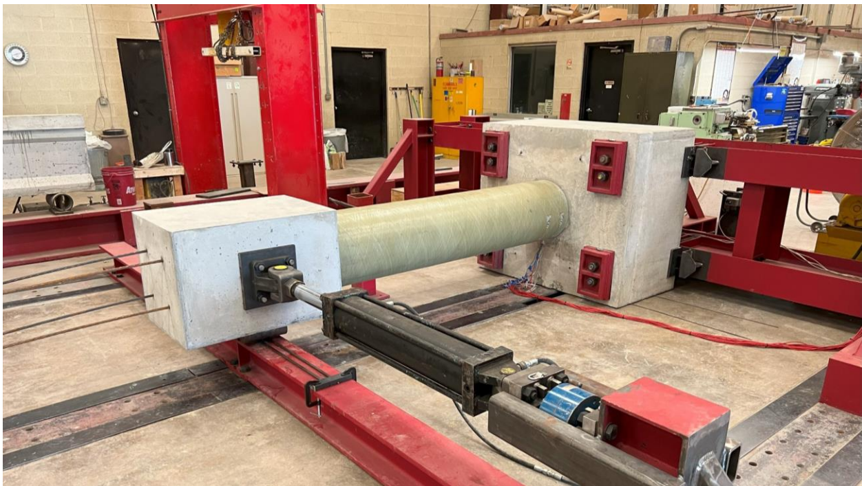
Figure 5-39: UHPC 2 Column Specimen Before Testing
