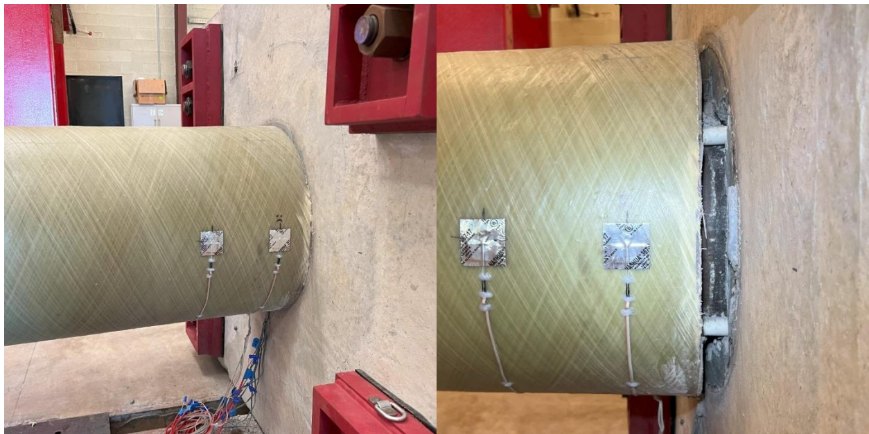
Figure 7-10: UHPC 1 GFRP Tube Compression (l) and Separation (r) During Testing
