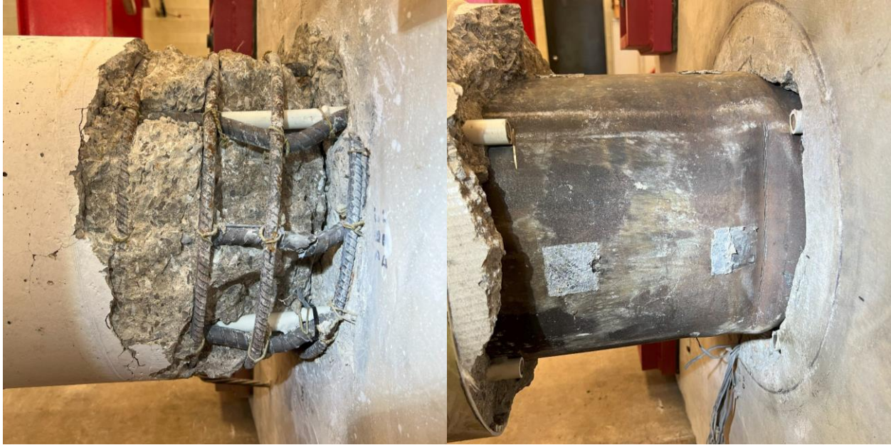
Figure 8-5: Comparing RC (l) and HS-SCC 2 (r) Steel Reinforcement After Testing
