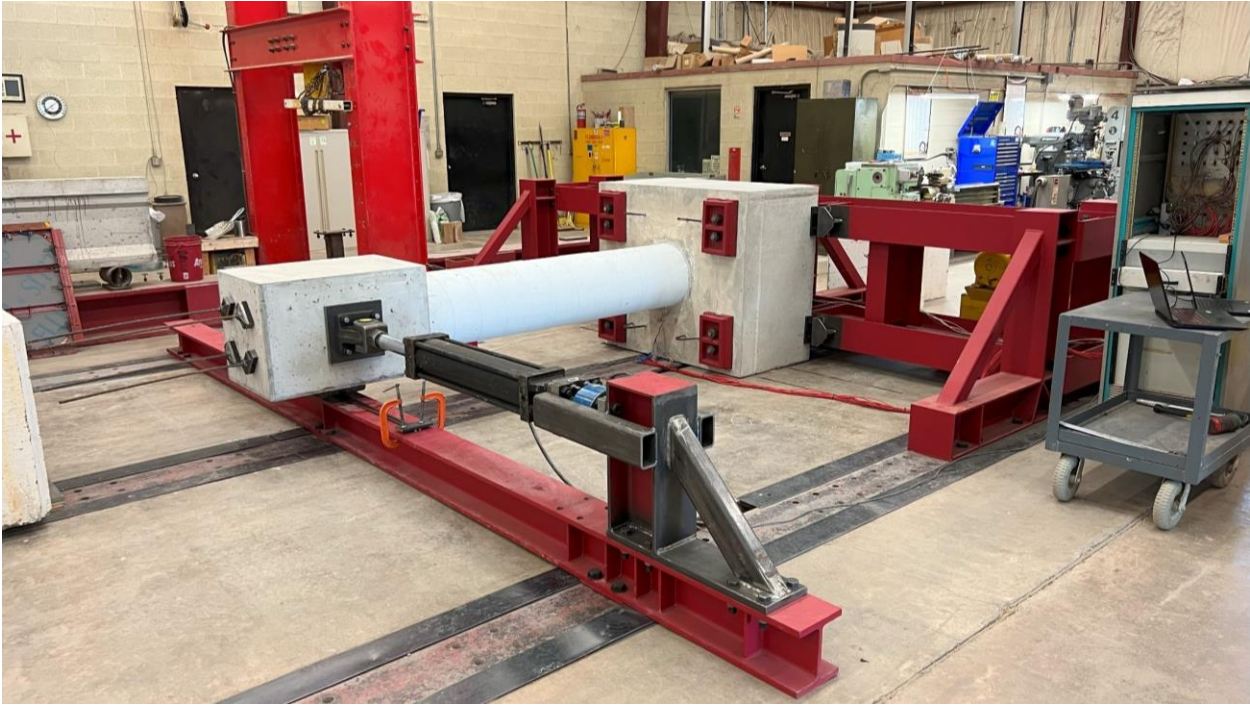
Figure 5-5: RC Column Specimen Before Testing
