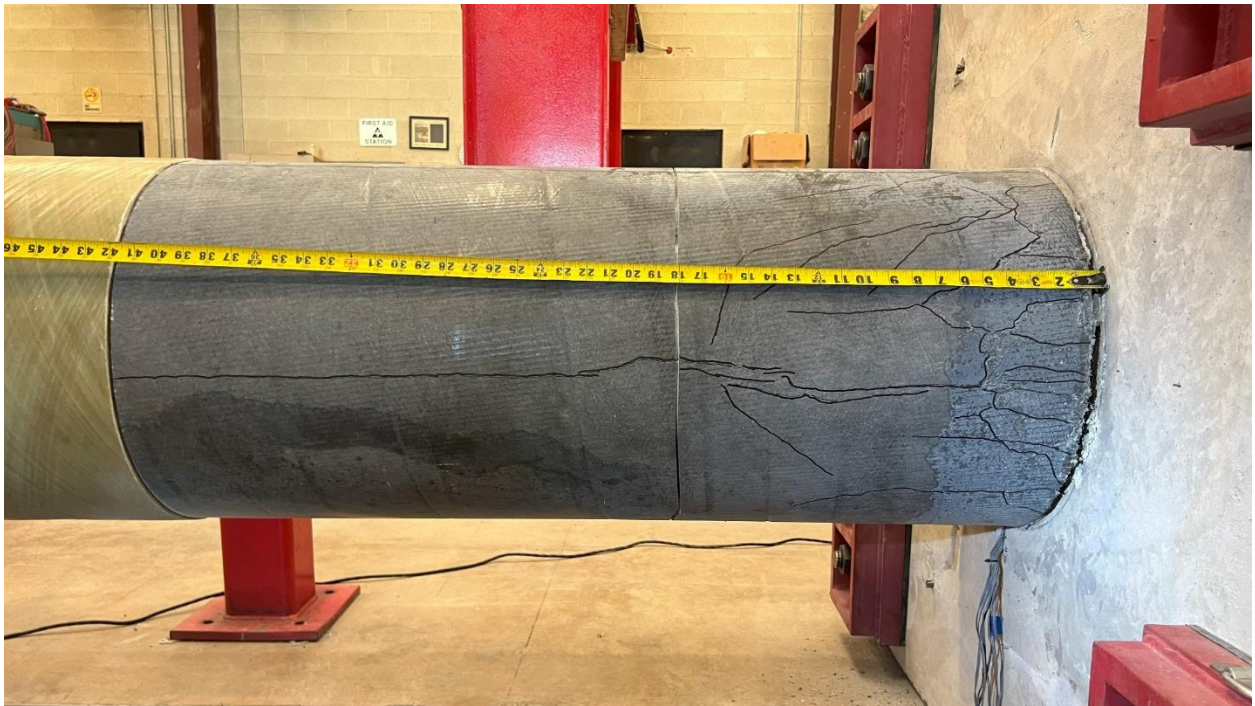
Figure 7-27: UHPC 2 Concrete Core West Side Cracking Along Column Height
