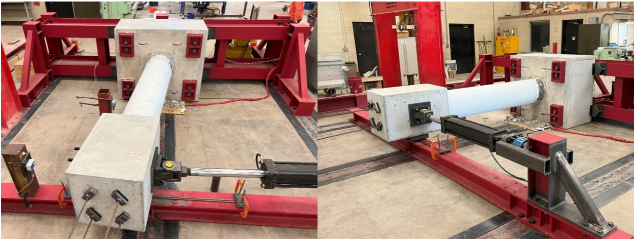
Figure 5-6: RC Column Specimen During (l) and After Testing (r)
