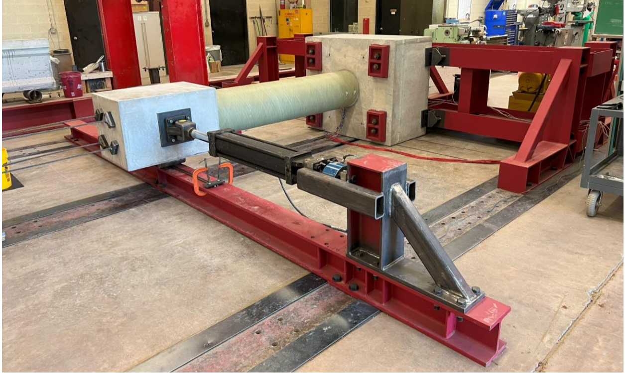
Figure 4-43: Completed Column Specimen Testing Arrangement
