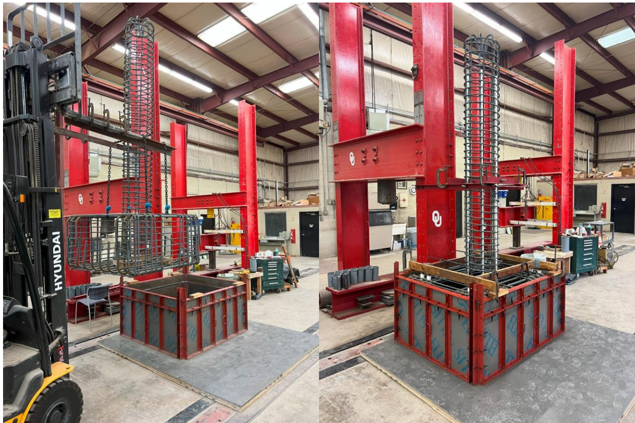
Figure 4-12: RC Column Base Assembly, Combined Cage Transportation and Placement (l) and Finalized Specimen Ready for Casting (r)
