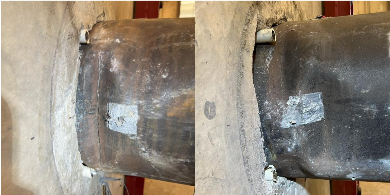
Figure 8-15: Comparing HS-SCC 2 (l) and UHPC 2 (r) Steel Tube East Side After Testing
