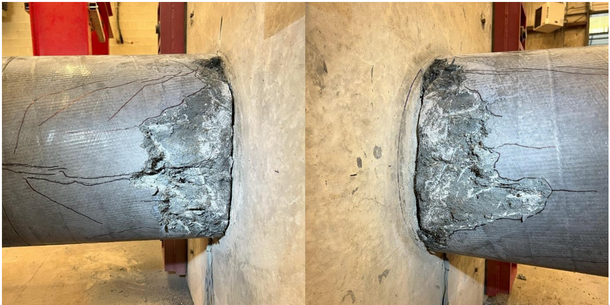
Figure 7-29: UHPC 2 Concrete Core After Testing and Light Concrete Removal
