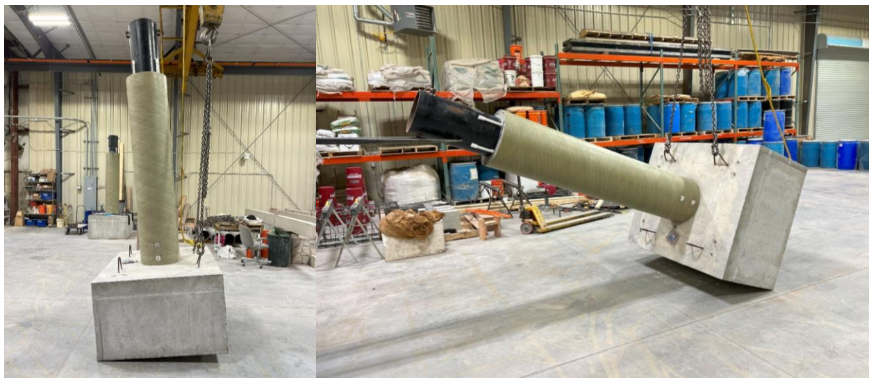
Figure 4-32: Column Specimen Tilting Process
