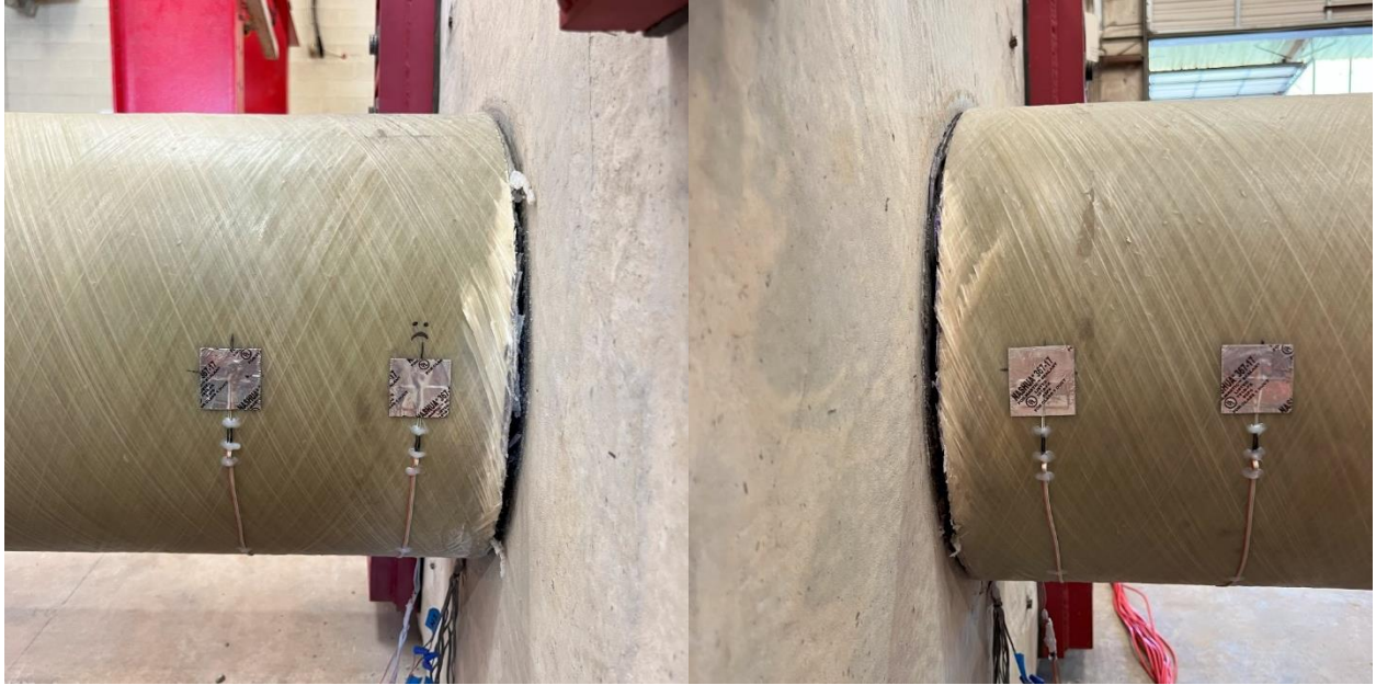
Figure 7-11: UHPC 1 GFRP Tube West Side (l) and East Side (r) Damage After Testing
