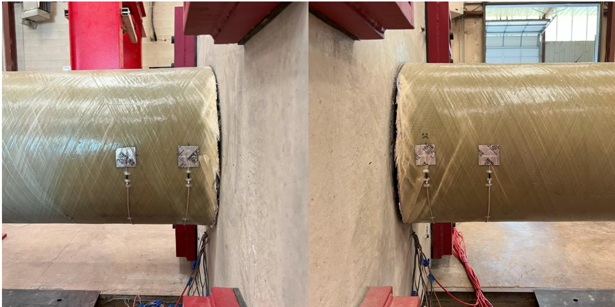
Figure 6-25: HS-SCC 2 GFRP Tube West Side (l) and East Side (r) Damage After Testing
