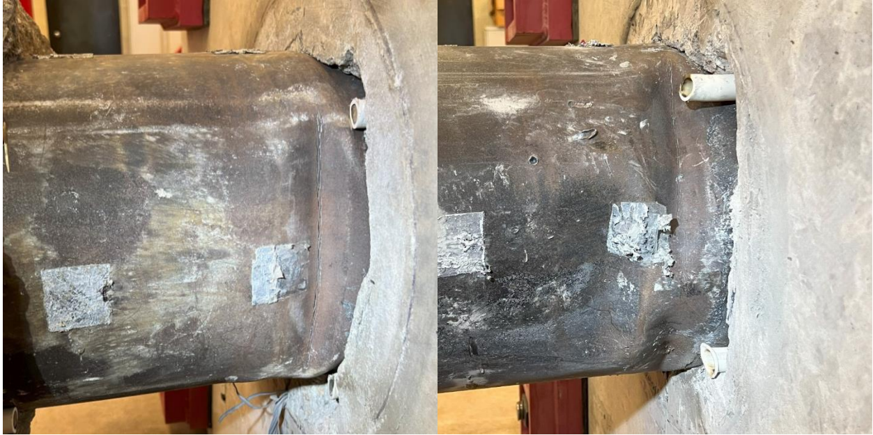
Figure 8-14: Comparing HS-SCC 2 (l) and UHPC 2 (r) Steel Tube West Side After Testing
