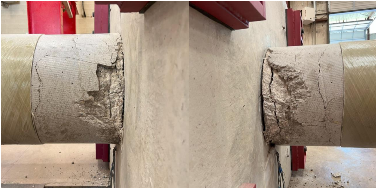
Figure 5-24: HS-SCC 2 Concrete Core After Testing and Light Removal of Concrete
