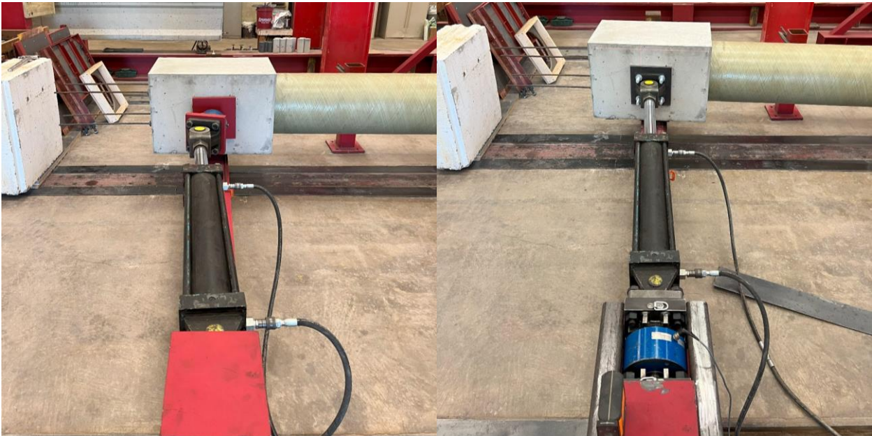
Figure 5-4: Original Loading System Failure (l) and the Redesigned Loading System (r)
