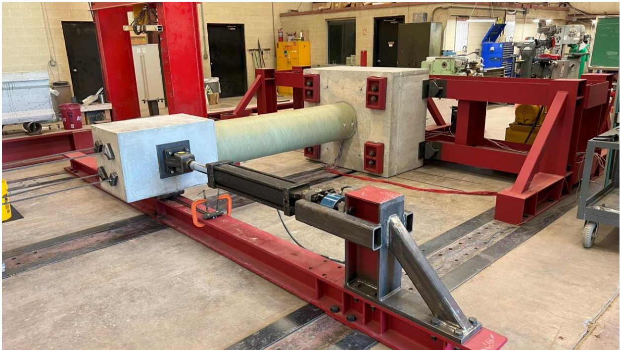
Figure 5-30: UHPC 1 Column Specimen Before Testing
