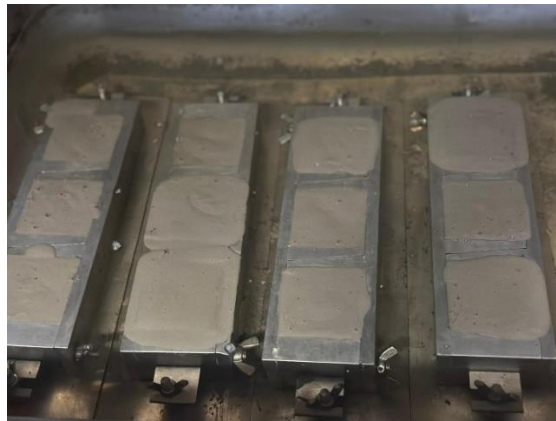
Figure 9. Class G + 20% FA being cured at high temperature.
