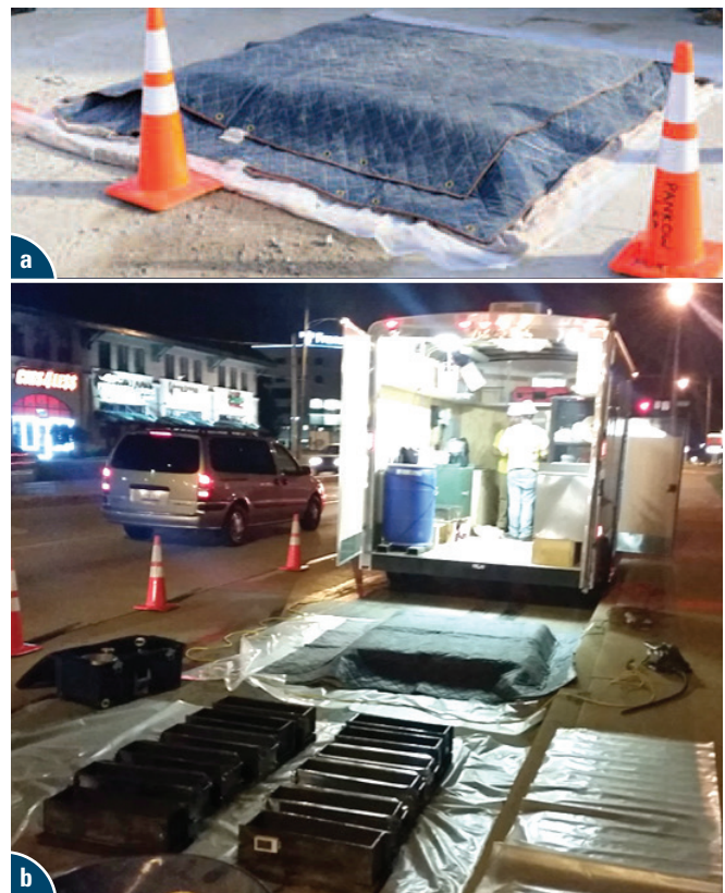
Figure 2. Field images of (a) temperature-matched curing beams from a trial batch and (b) temperature-matched curing beams and air-cured beams during a site visit
