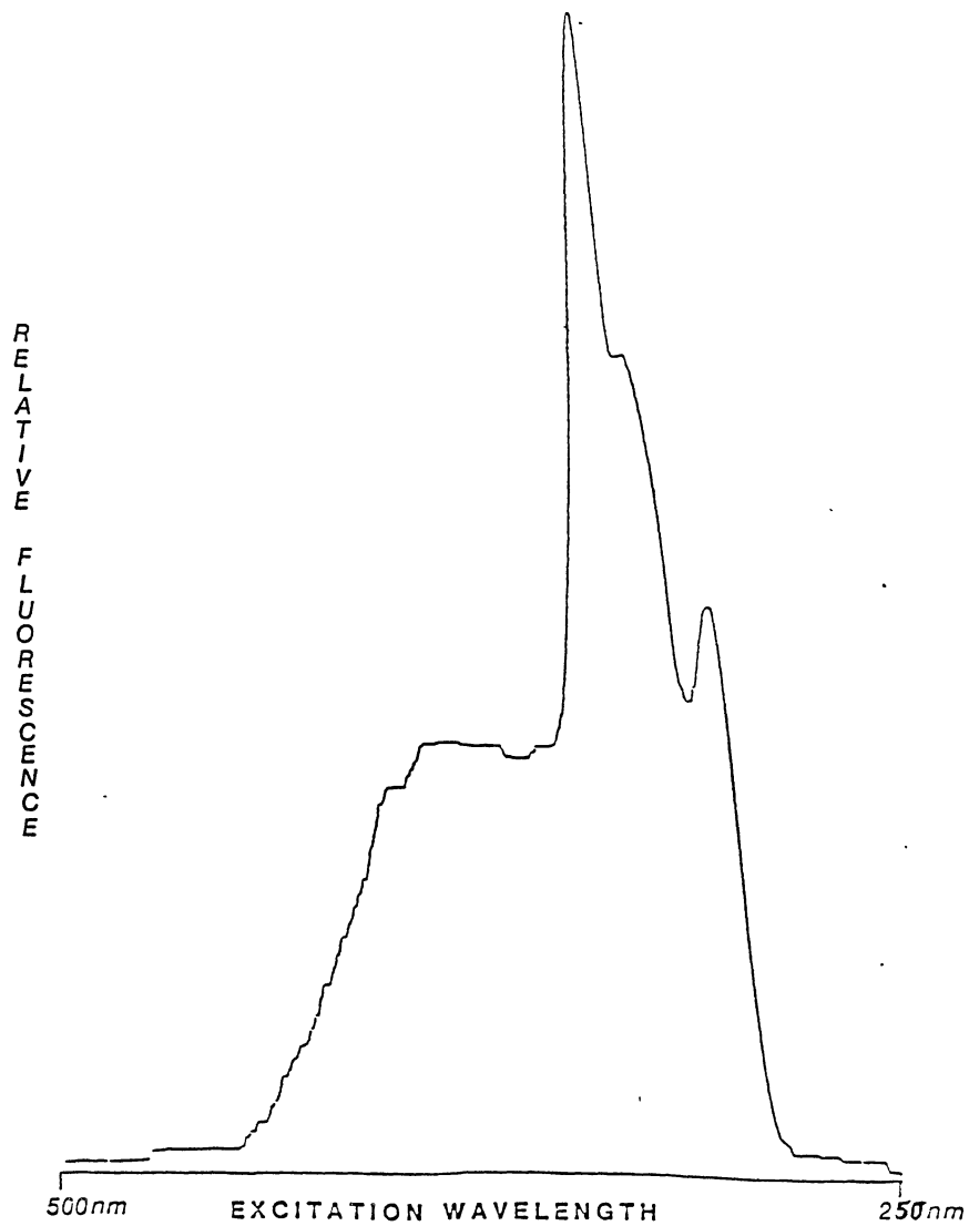
Figure 4. Excitation spectrum of the europium-diphacinone complex. Conditions: 7.88 \times 10^{-6} M diphacinone, 1 \times 10^{-4} M europium, 7.2 \times 10^{-4} M trioctylphosphine oxide, 1% pyridine in acetonitrile. Emission wavelength 613 nm. Excitation max. 328 nm.
