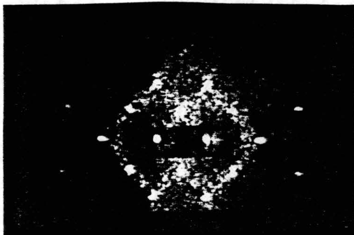
Figure 35a. Self-Diffraction Pattern. The Average Particle Separation is 2.5 \mu\text{m} , the Fringe Spacing is 1.77 \mu\text{m} and the Two Central Bright Spots Partially blocked by Tape are the Emerging main Beams
