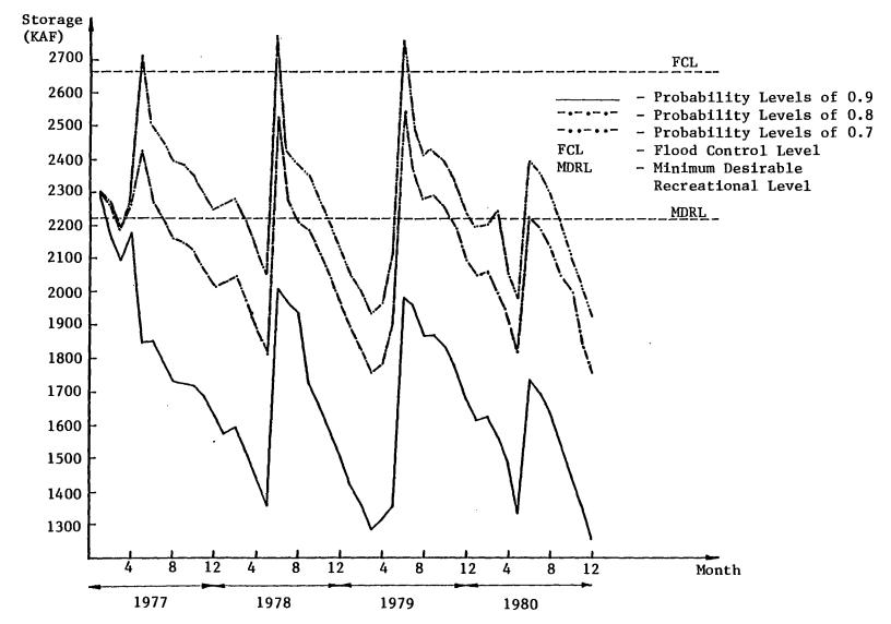
Figure 10. Projected Storage of Denison Reservoir With Priority Structure: FC, M&I, D, P, R
