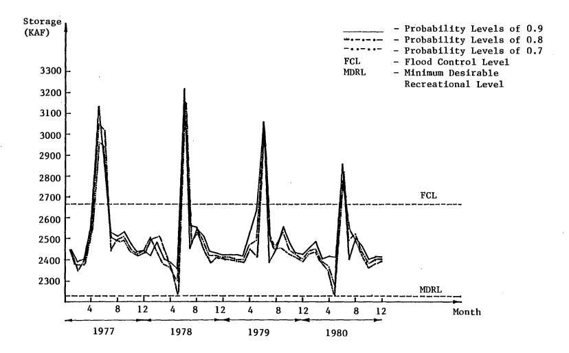
Figure 9. Projected Storage of Denison Reservoir With Priority Structure: M&I, D, R, P, FC
