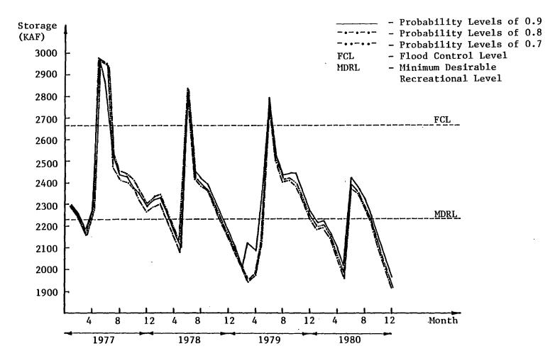
Figure 12. Projected Storage of Denison Reservoir With Priority Structure: M&I, D, P, R, FC
