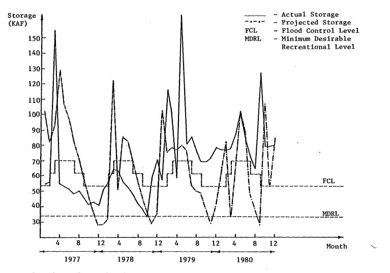
Figure 8. Plots of Actual and Projected Storages for Pine Creek Reservoir from 1977-1980
