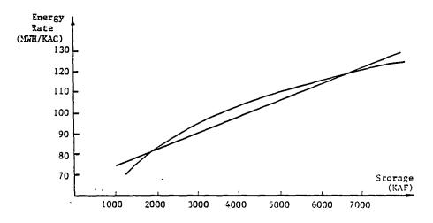
Figure 14. Plots of Energy Rate Against Storage for Denison Reservoir
