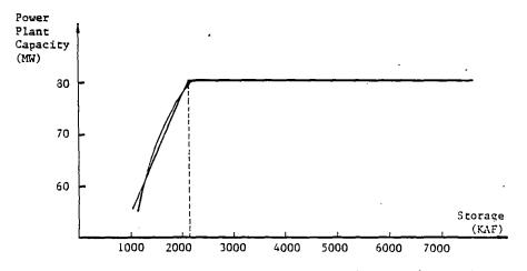
Figure 15. Plots of Power Plant Capacity Against Storage for Denison Reservoir
