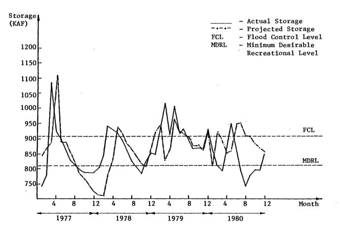
Figure 7. Plots of Actual and Projected Storages for Broken Bow Reservoir from 1977-1980
