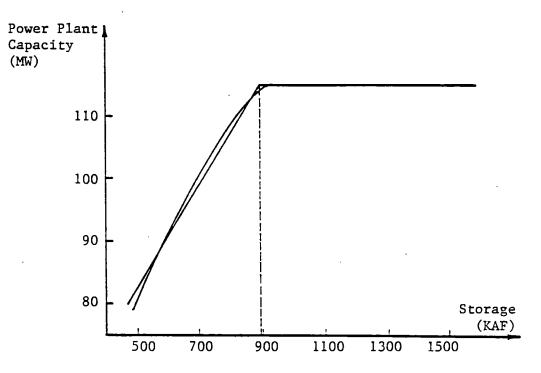
Figure 18. Plots of Power Plant Capacity Against Storage for Broken Bow Reservoir
