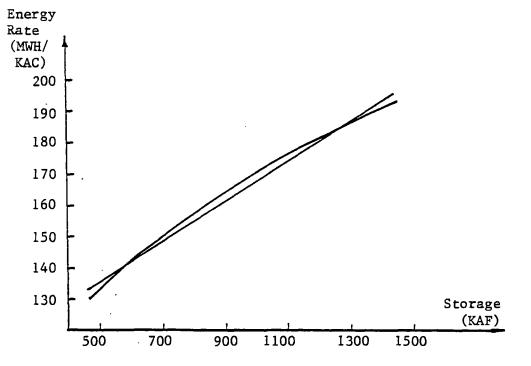
Figure 17. Plots of Energy Rate Against Storage for Broken Bow Reservoir
