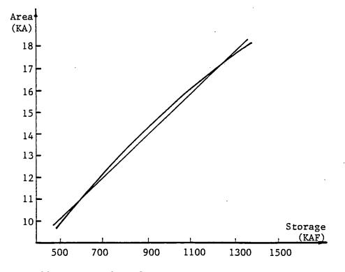
Figure 19. Plots of Surface Area Against Storage for Broken Bow Reservoir
