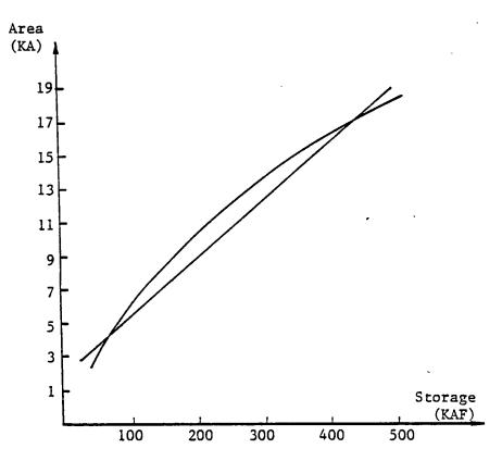
Figure 20. Plots of Surface Area Against Storage for Pine Creek Reservoir
