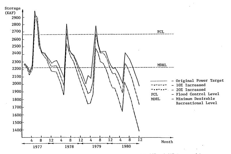
Figure 11. Projected Storage of Denison Reservoir With 10% and 20% Increased in Power Targets (Priority Structure is: M&I, D, P, R, FC)
