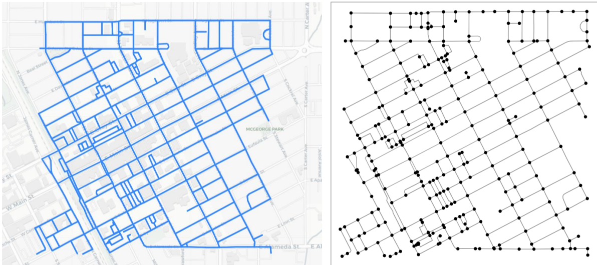
Figure 14: Bicycle network from the Norman, Oklahoma (left) & graphical representation of the network as set of nodes and edges (right)
