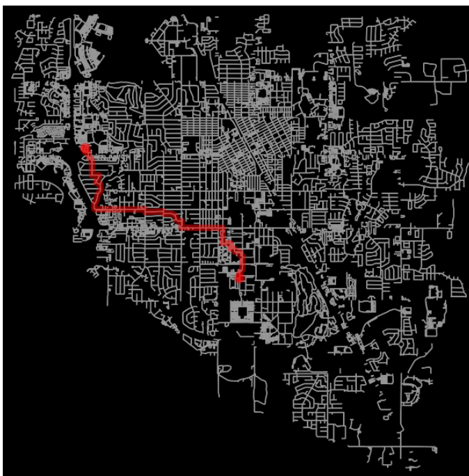
Figure 5: Finding shortest route using Dijkstra's algorithm and graph theory.
