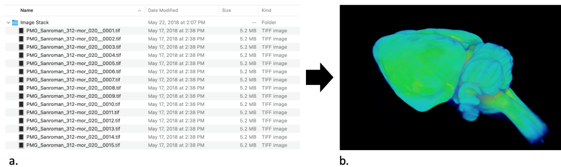
Figure 2.4. Avizo visualizes an image stack. (a) The output of a CT scan is an image stack that (b) imaging software, such as Avizo, combines into a 3-D rendering of a specimen.
