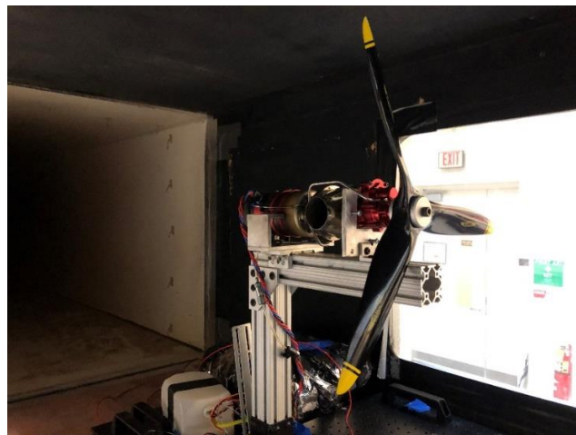
Figure 42. Turboprop with Propeller Locked.
