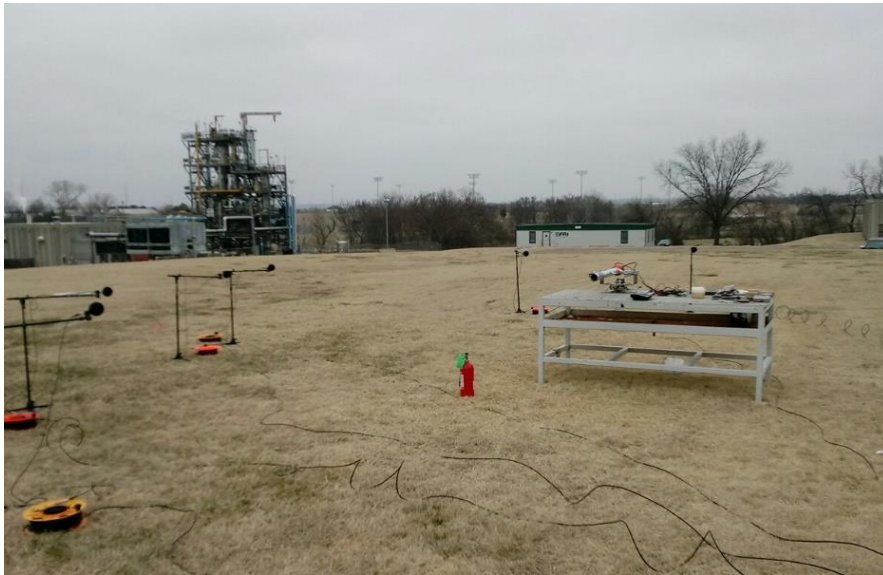
Figure 33. Acoustic Testing Microphone Semi-Circle.
