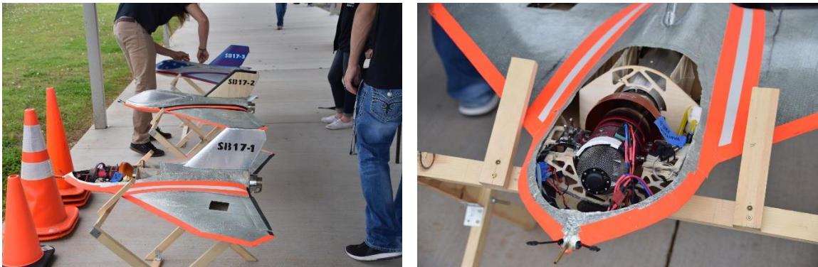
Figure 1. Example of a Small Turbojet Integrated into an Airframe.
