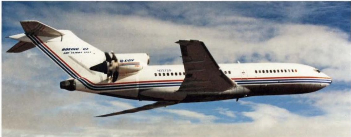
Figure 7. Unducted Fan Flight Tests during the Advanced Turboprop Project [7].
