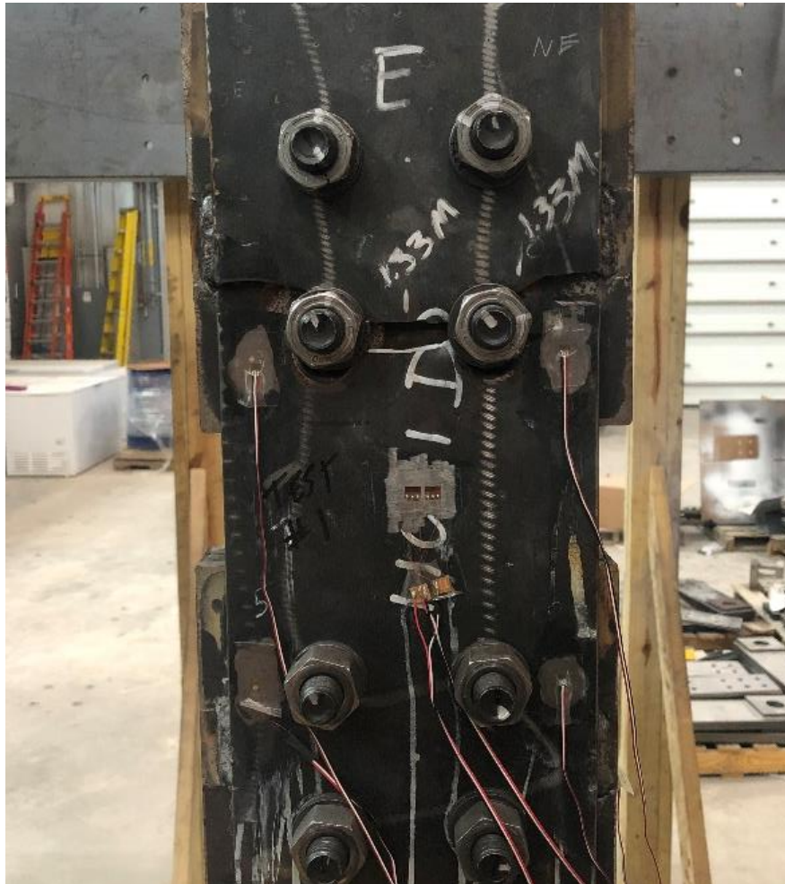
Figure 5.16: Fatigue Test Specimen after Failure
