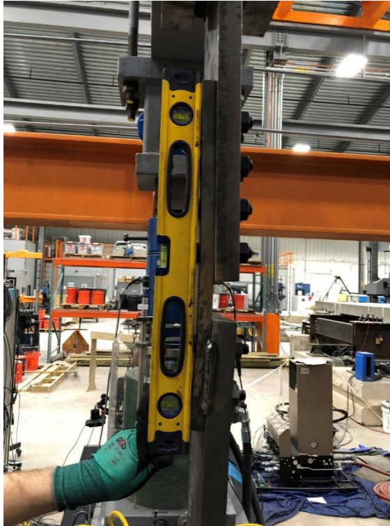
Figure 5.6: Image of Bending that occurred in Single Shear Splice Plate after Test 4A at Bert Cooper Lab in Stillwater, OK
