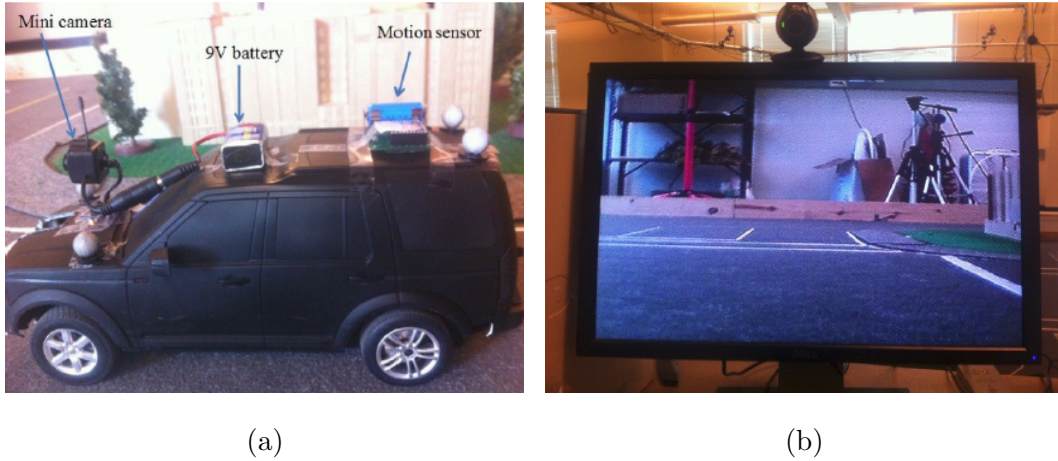
Figure V.10: Manual driving experiment setup. (a) The miniature camera setup, (b) An image streamed back from the miniature camera.
