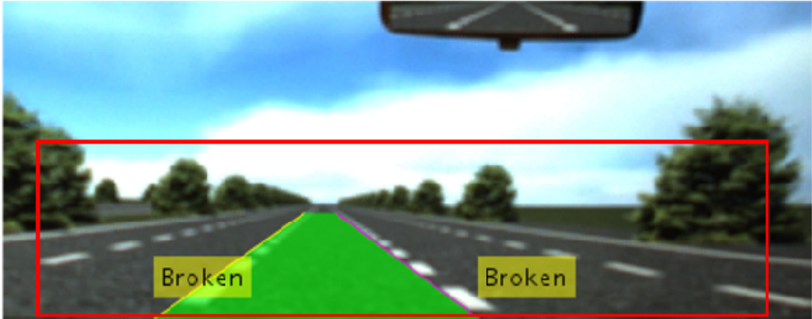
(a) Detected broken lines
