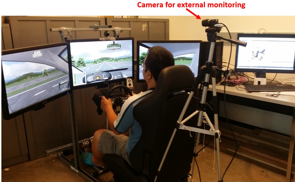
Figure VII.1: The overall experimental setup of the video-based external risk assessment system.
