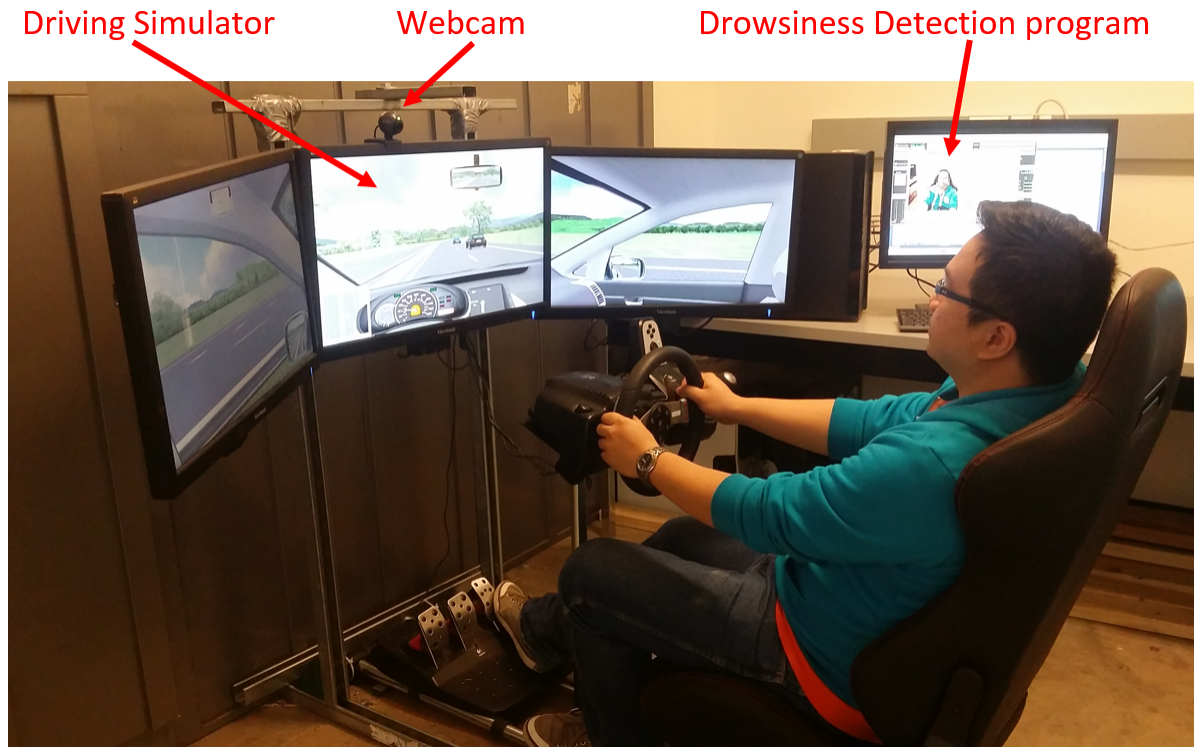
Figure V.2: The experimental setup of the drowsiness detection's application in the simulated testbed.
