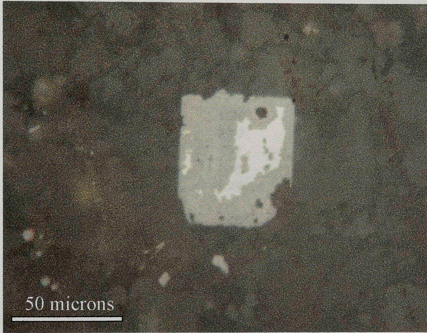
Figure 13: Thin section showing magnetite replacing pyrite in reflected light.
