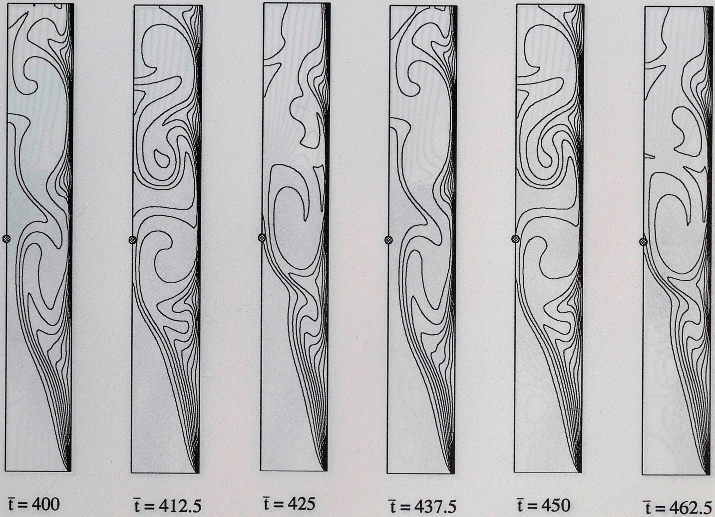
Figure 4.26d Development of Temperature Field - Aiding Flow (One and Half Period) Re=600 Gr=10^4
