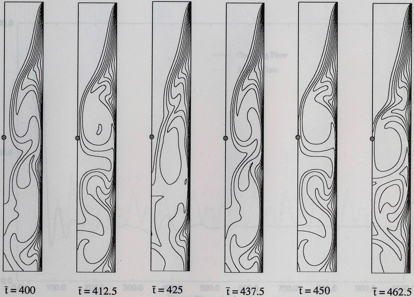
Figure 4.27d Development of Temperature Field - Opposing Flow (One and Half Period)
