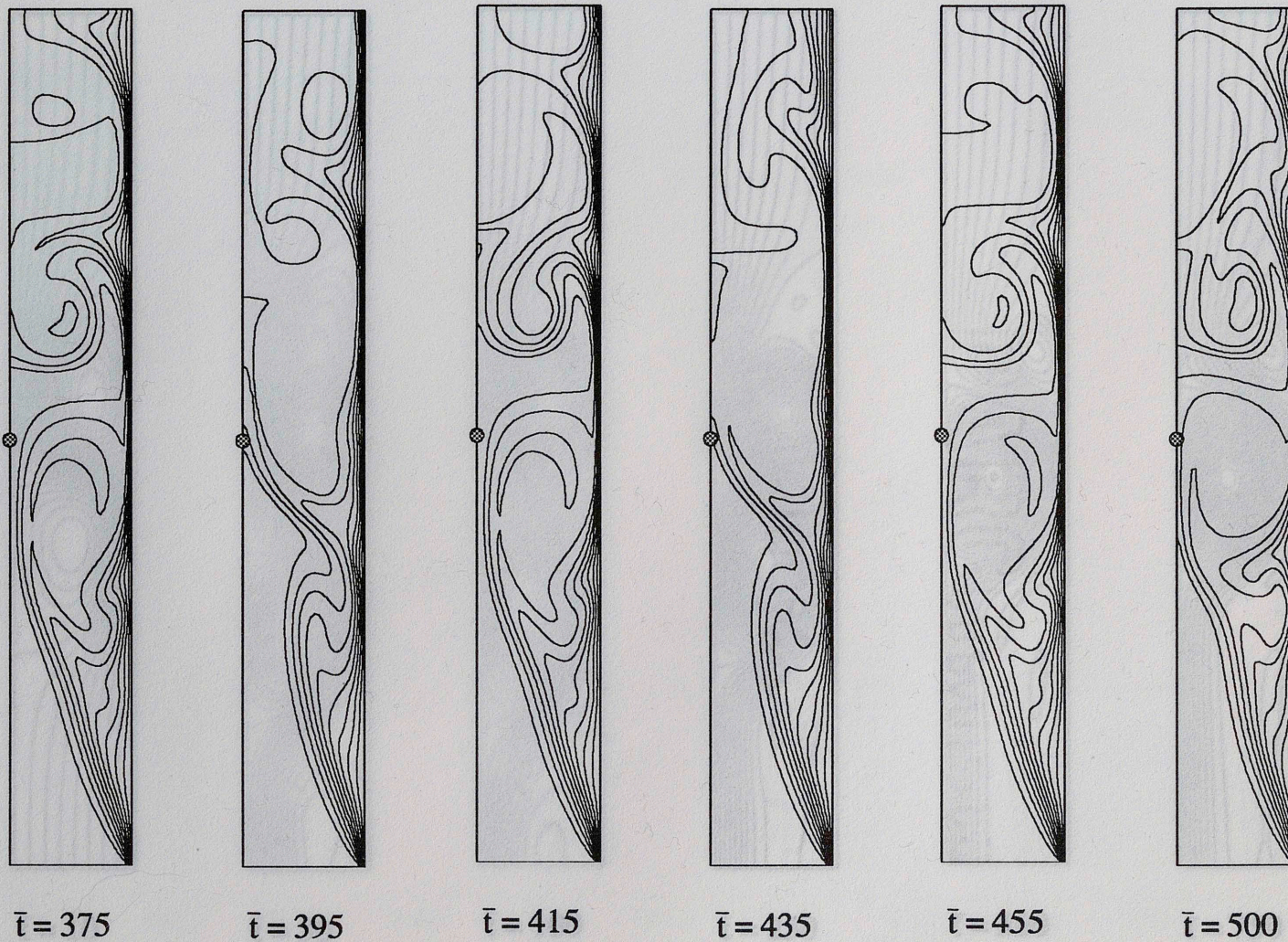
Figure 4.29d Development of Temperature Field - Aiding Flow (One Period) Re=600 Gr=10^5
