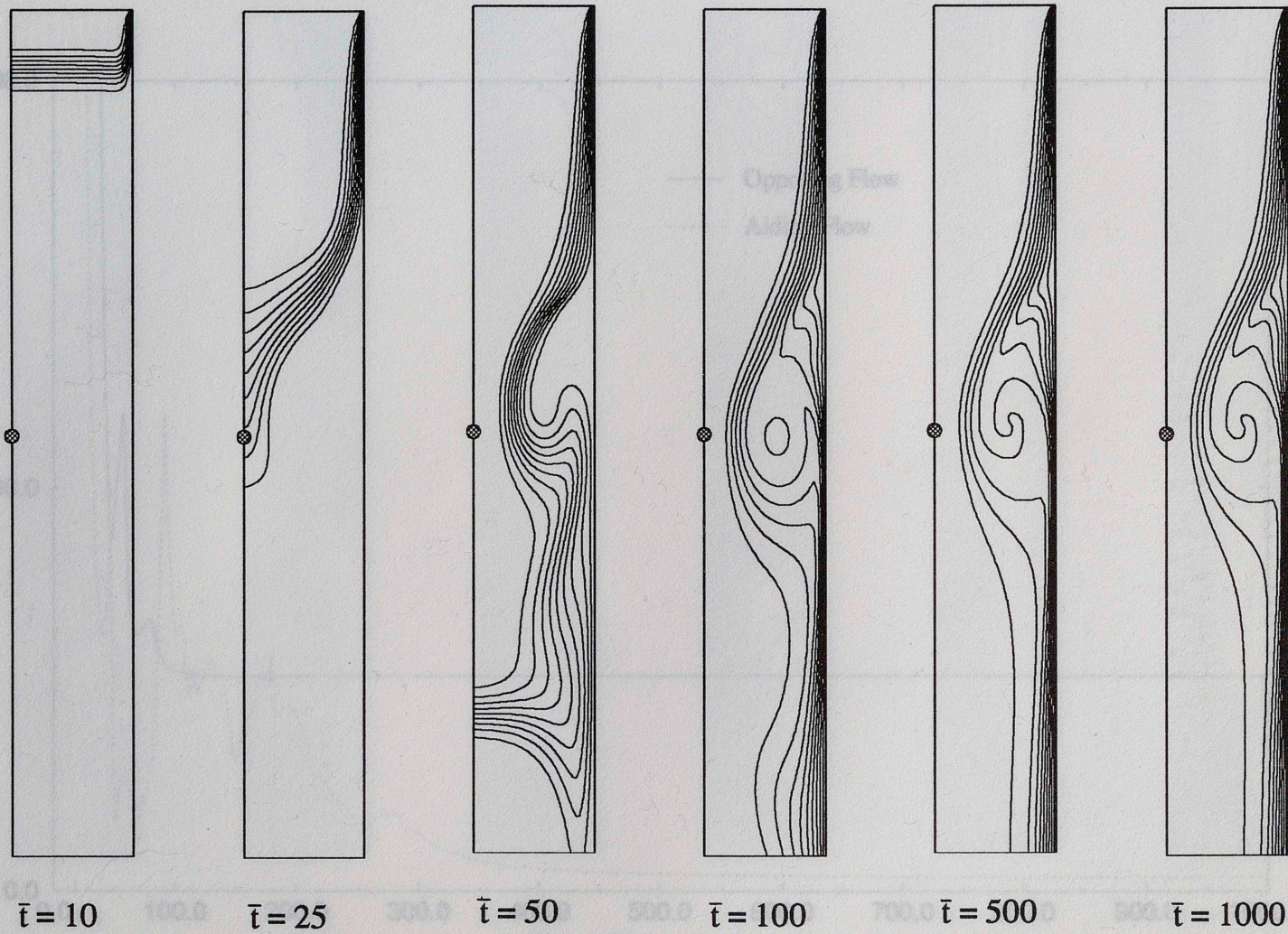
Figure 4.19b Development of Temperature Field - Opposing Flow
