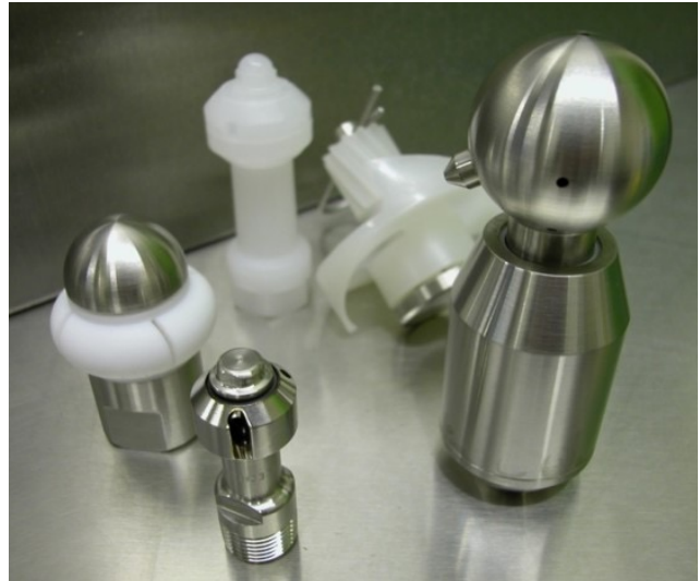
Figure 4. Fluid driven dynamic spray devices. Photo courtesy of the Robert M. Kerr Food and Agricultural Products Center, Oklahoma State University.
