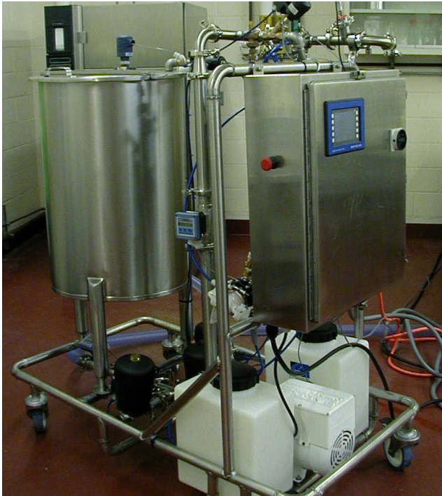
Figure 1. Single-use CIP system. Photo courtesy of the Robert M. Kerr Food and Agricultural Products Center, Oklahoma State University.
