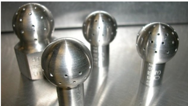
Figure 3. Fixed spray balls, Photo courtesy of the Robert M. Kerr Food and Agricultural Products Center, Oklahoma State University.
