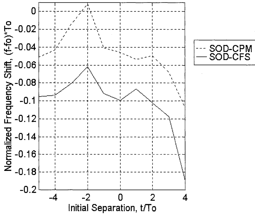
Figure 5.26.2 STG-NOLM gate output control pulse frequency shift against initial separation at L = 11l_{wo} .
