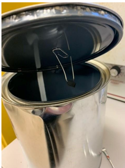
Figure 27. A picture of a C-strip suspended by a paper clip for passive headspace extraction.
