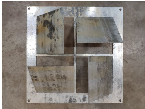
Figure 91 Air mixer types tested: (a) Baseline louvered mixer, (b) Orifice mixer, (c) Perforated target plate for orifice-target mixer, (d) Orthogonal pattern louver mixer with 6 by 6, (e) 4 by 4, and (f) 2 by 2 louver arrays.
