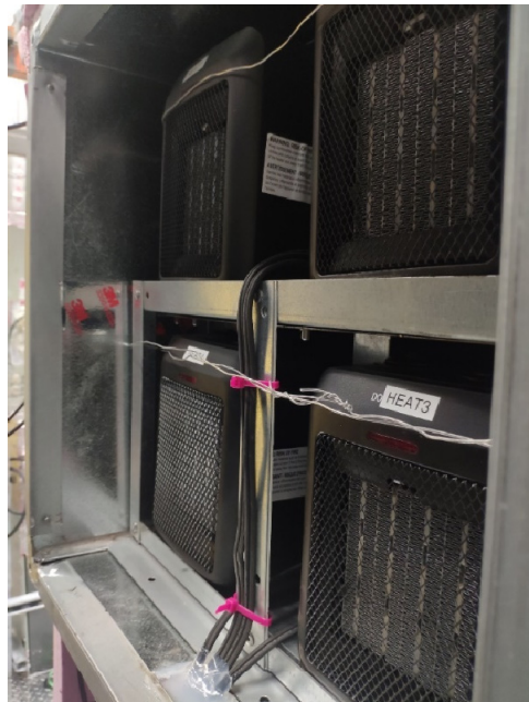
Figure 85 Experimental setup for in-situ testing: (a) Single orthogonal pattern louver mixer with 4 by 4 louver array and 60° louver angles, and (b) Four electric heaters installed in quadrants.
