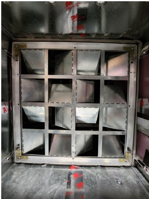
Figure 85 Experimental setup for in-situ testing: (a) Single orthogonal pattern louver mixer with 4 by 4 louver array and 60° louver angles, and (b) Four electric heaters installed in quadrants.
