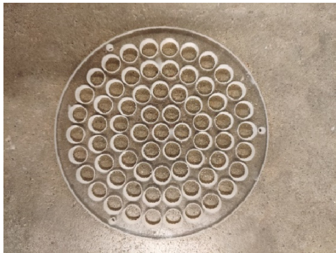
Figure 91 Air mixer types tested: (a) Baseline louvered mixer, (b) Orifice mixer, (c) Perforated target plate for orifice-target mixer, (d) Orthogonal pattern louver mixer with 6 by 6, (e) 4 by 4, and (f) 2 by 2 louver arrays.
