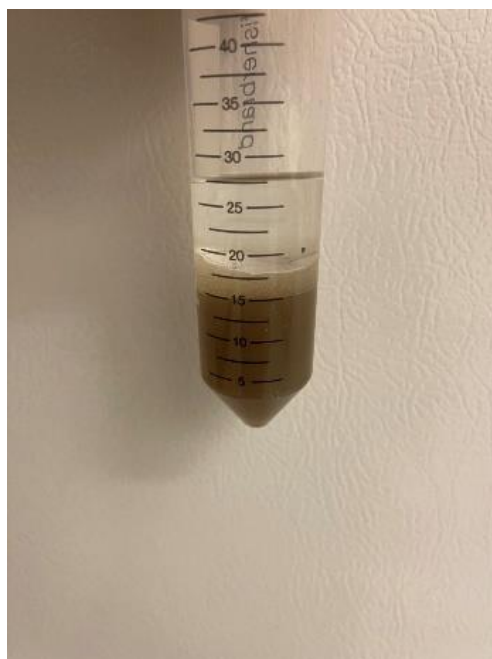
Figure A.7: Prevention of the adsorption of nanostructures to the water-oil interface in the presence of triton X-100.
