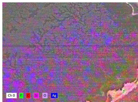
Figure A.3: The elemental map collected by EDX analysis of the same sample in figure A.2 in which air was used as the secondary phase.
