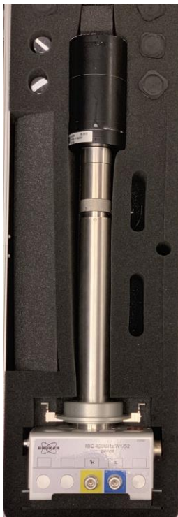
Figure 24. Diffusion probe, gradient strengths up to 2900 Gauss/cm
