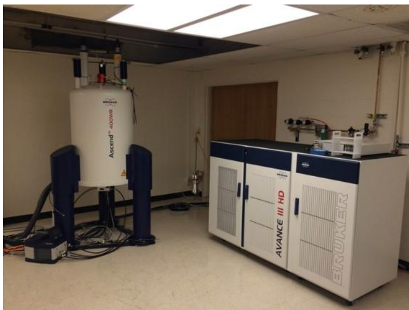
Figure 23. NMR Bruker 400 MHz (9.4 T) NMR spectrometer
