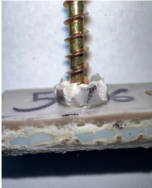
Figure 4.38: cPET/rPET with screw partially withdrawn from material.
