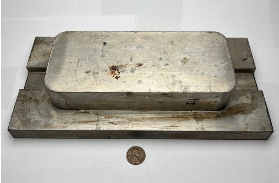
Figure 3.4: Top/bottom section of mold.
