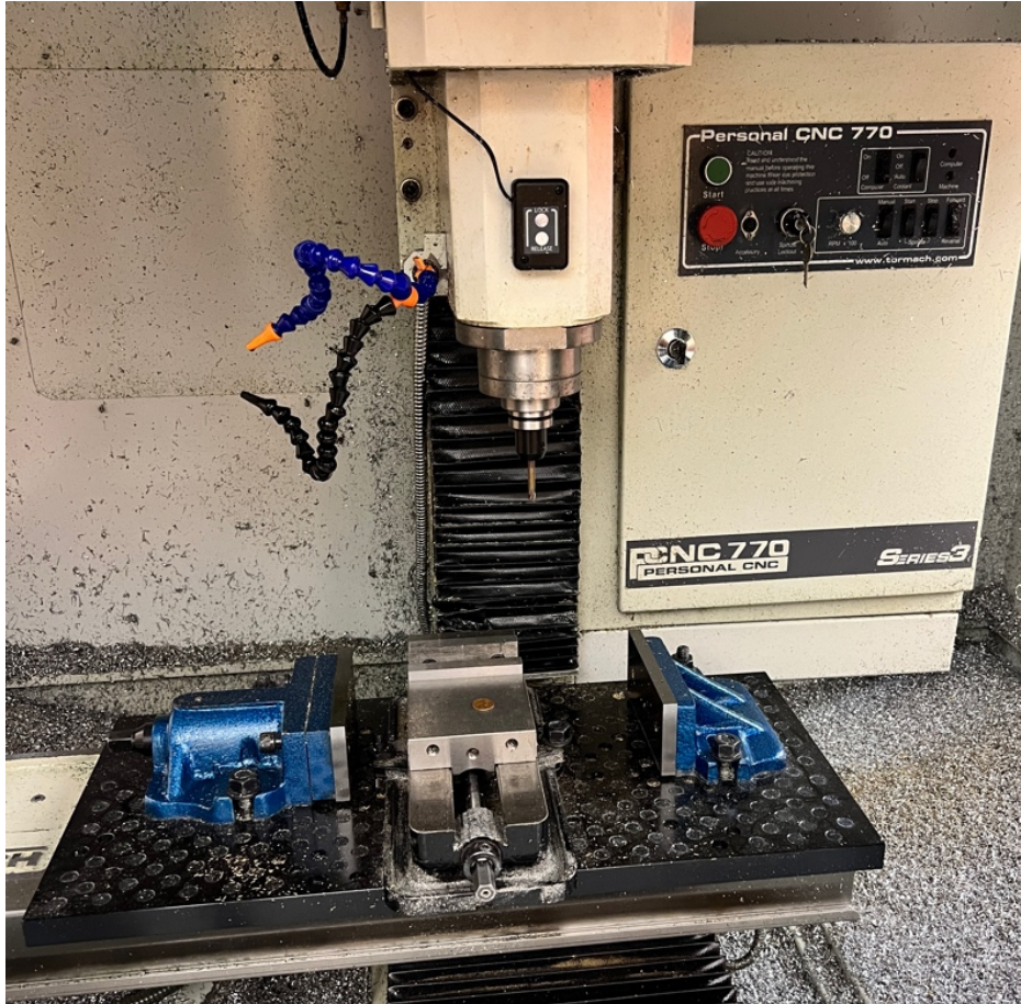
Figure 3.2: Tormach PCNC 770 CNC milling machine.
