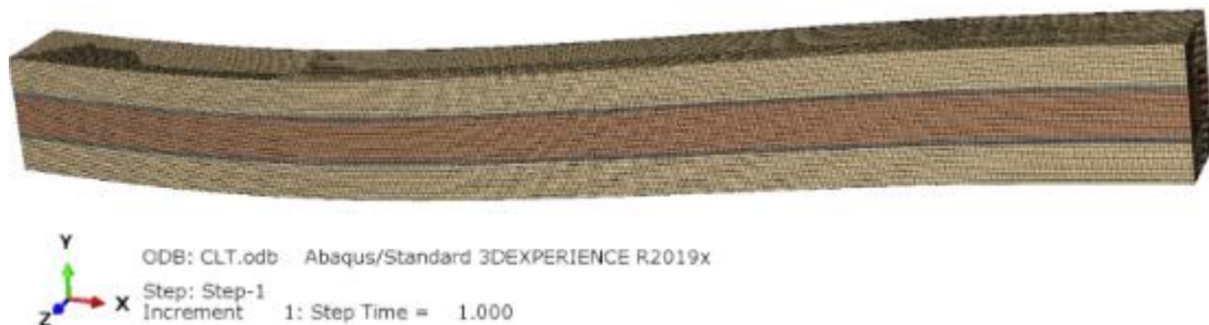
Figure 24: Abaqus FEA Model for 1/4 Length of Spruce 5-Layer Beam [18]
