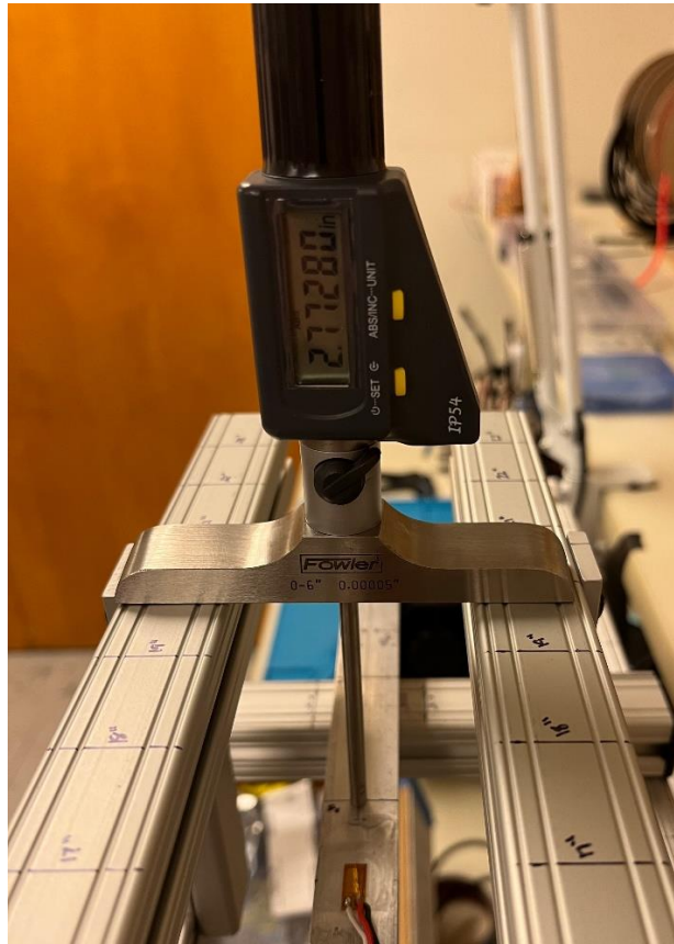
Figure 36: Beam Deflection Measurement Technique Using Depth Gauge
