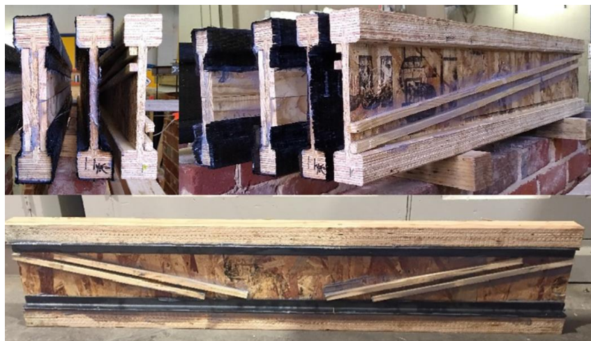
Figure 18: Composite Timber I-beam Reinforcement Techniques [17]
