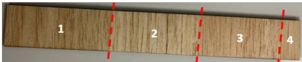
Figure 93: Example of Laminated Balsa Strips to Achieve Requested Density
