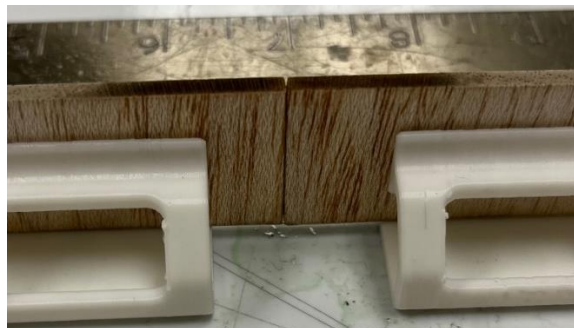
Figure 94: Process for Assembling Balsa Shear Web with CA
