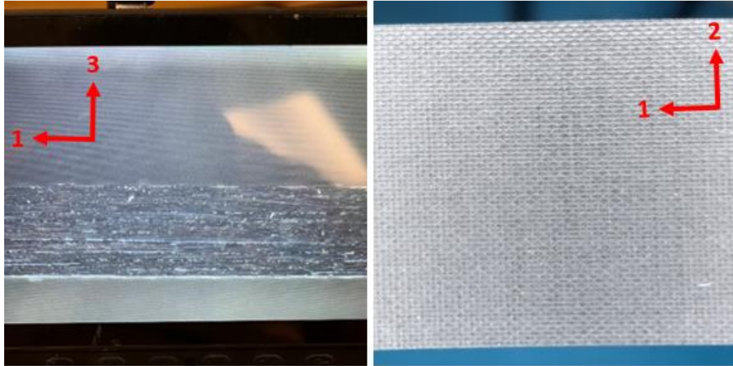
Figure 92: Unidirectional Carbon Laminate Fiber Direction and Surface Texture
