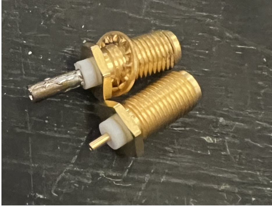
Figure 16: SMA bulkhead connectors used for measurement.
