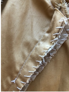
Figure 19, Seams of Garment. Note how there is no space between the straight stitches, indicating that this was done on a machine. Photo by author.
