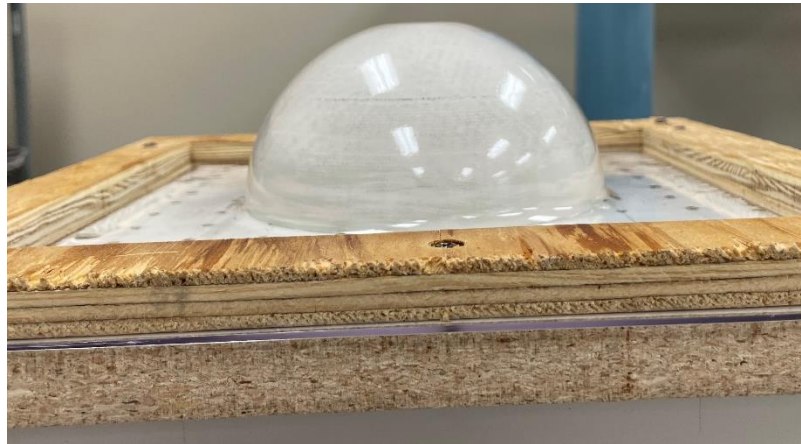
Figure 39: Formed and Cooled Part
