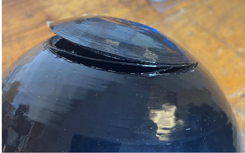
Figure 32: Nylon Tank Failure
