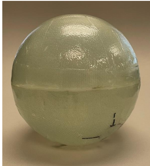
Figure 19: Completed Fiberglass Tank
