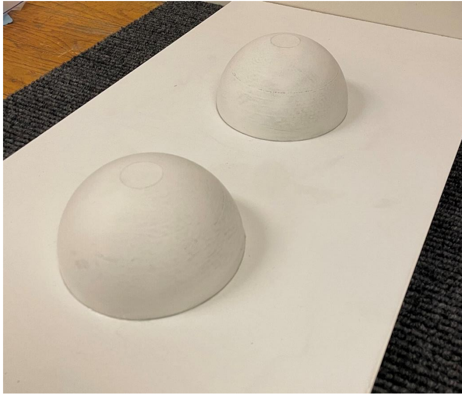
Figure 18: Finished Composite Mold
