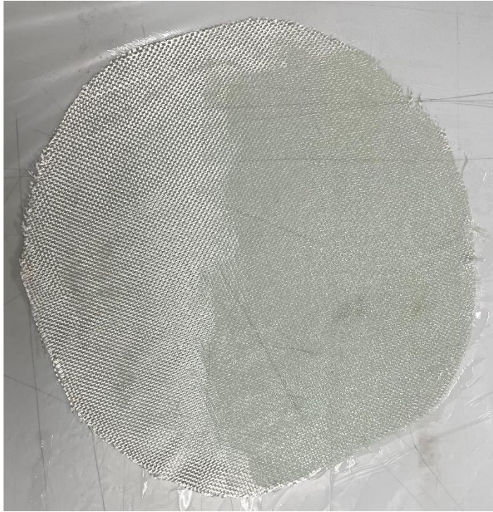
Figure 46: Dry (Left) and Wetted (Right) Fabric Comparison
