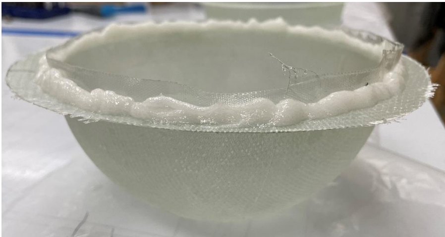
Figure 54: Thickened Epoxy Applied Along Exterior Perimeter
