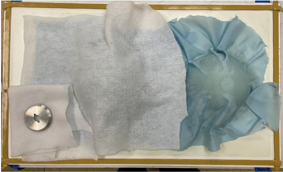
Figure 48: Chromate (Boarder), Separation Material (Right), Breather (Middle), Medallion (Left)
