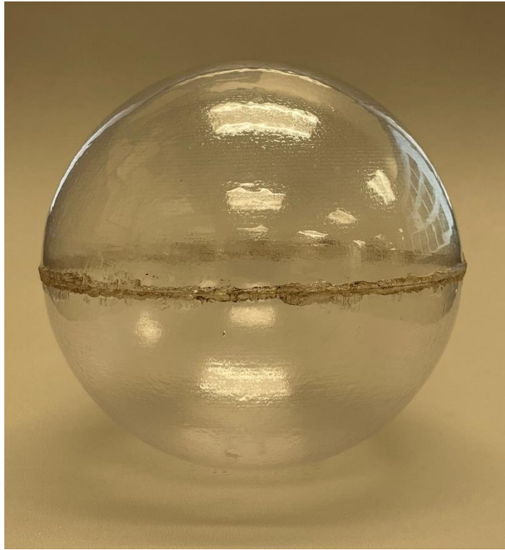
Figure 24: Completed Thermoformed Fuel Tank
