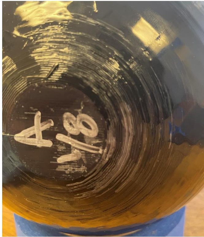
Figure 35: Damaged Sustained by ASA Tank (36in Drop)
