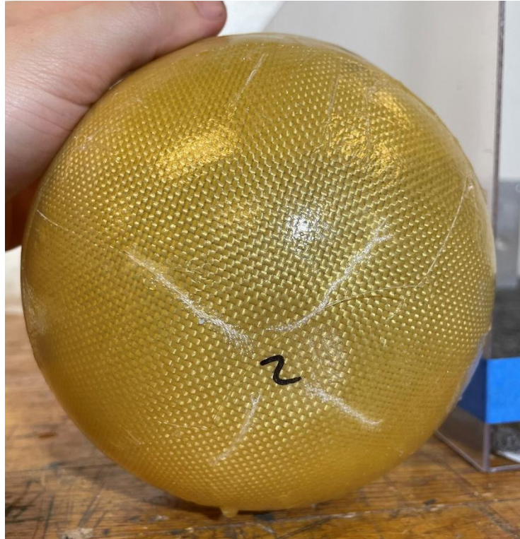
Figure 30: Sixteen Inch Drop Test Results (Kevlar)
