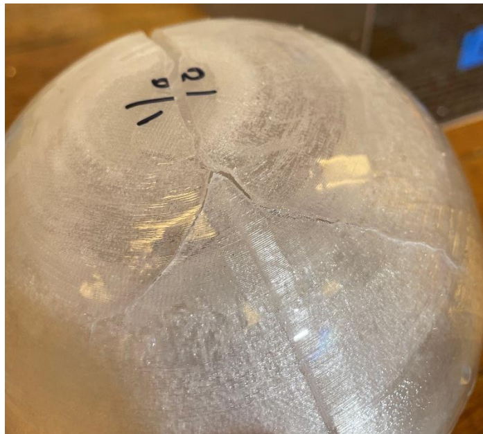
Figure 33: PETG Failure (Top View)
