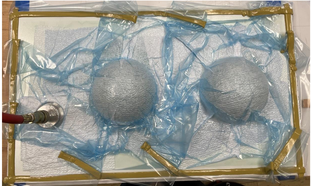
Figure 50: Example of Completed Bag at 24in-Hg
