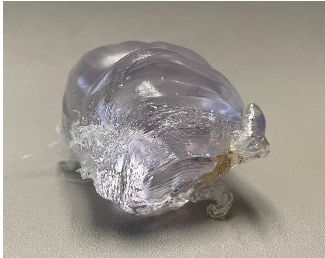
Figure 15: PETG Extrusion Failure
