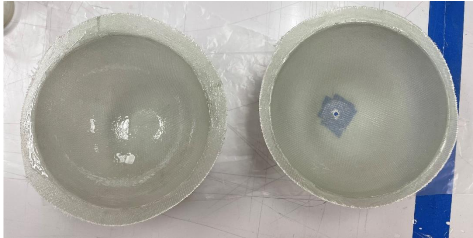
Figure 52: Laminated (Left) vs Unlaminated (Right) Composite Fuel Tank Halves
