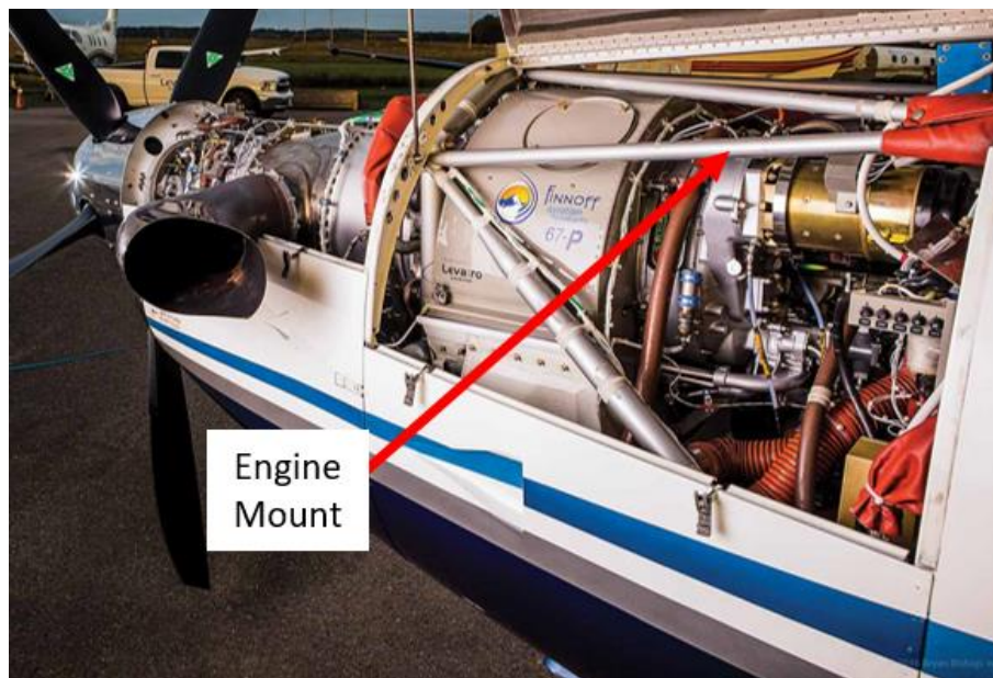
Figure 16. Typical Aviation Turboprop Engine Mount (Mark, 2019).
