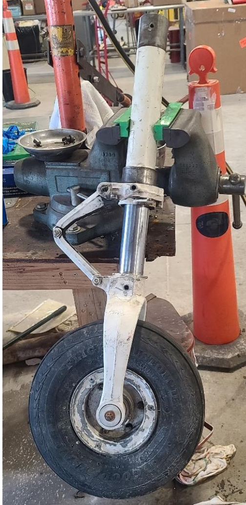
Figure 29. Reassembled and charged nose strut.
