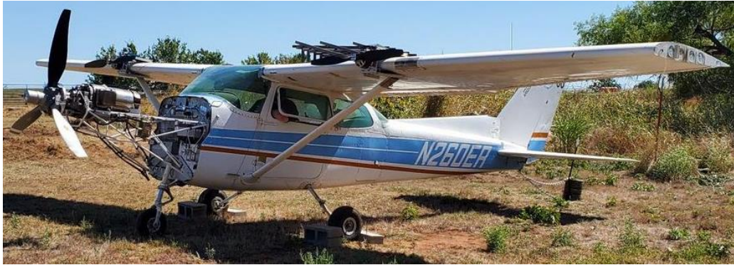
Figure 2. Turboelectric Ground Test Rig.
