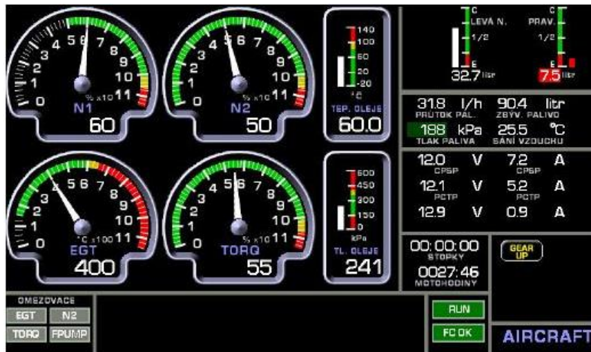
Figure 75. Engine Monitoring System (PBS Aerospace , 2014).
