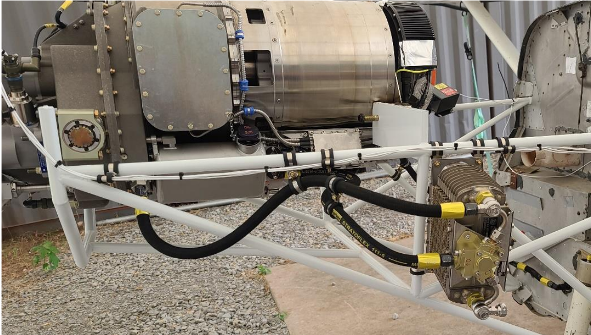
Figure 24. Oil Cooling Loop.
