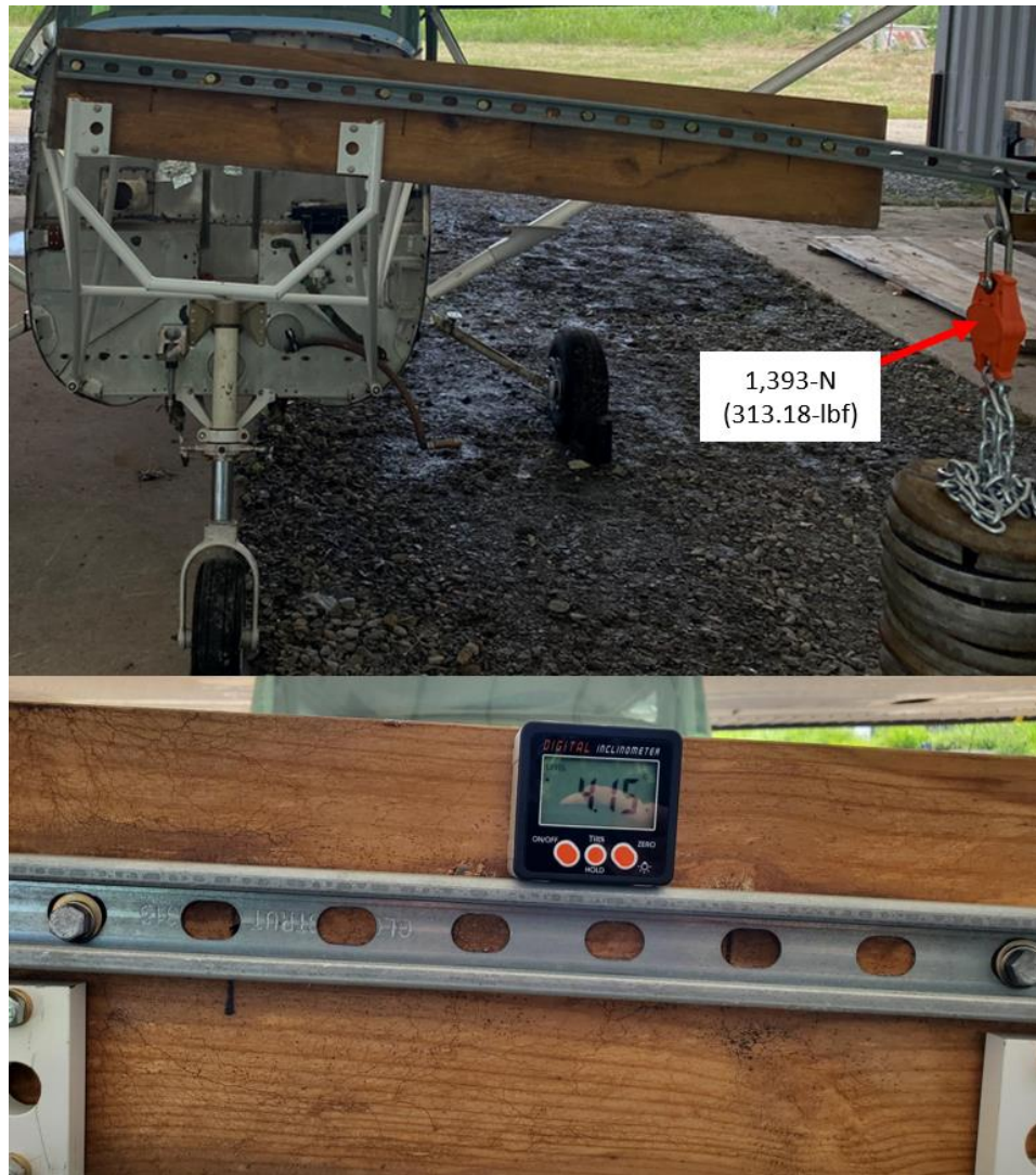
Figure 34. Engine Mount Static Torque Check.
