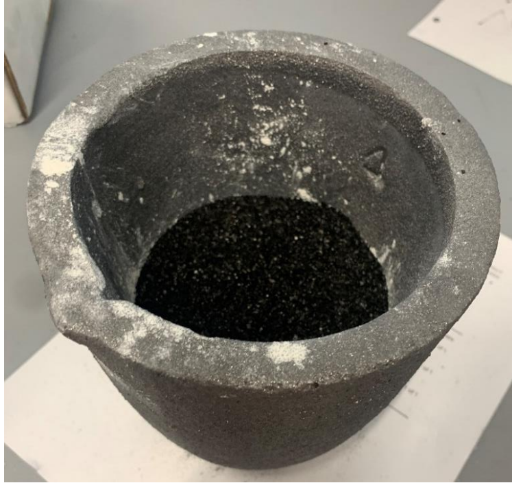
Figure 17: Copper Samples Buried in Talc and Sintering Carbon
