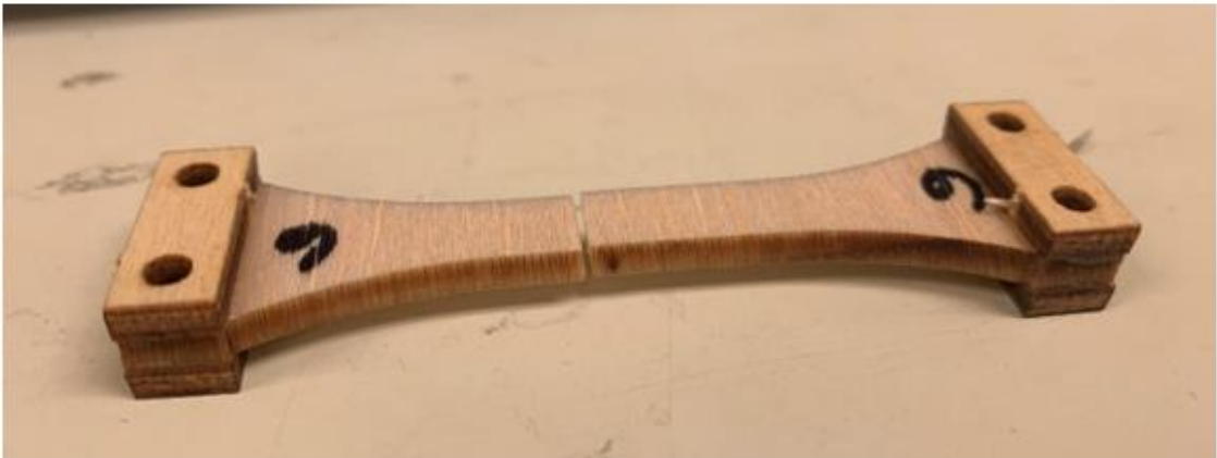
Figure 69: XL_6, 0.125", Incorrect Prediction of Failure Location
