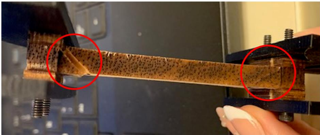
Figure 66: XH_13, Correct Failure Location Predicted
