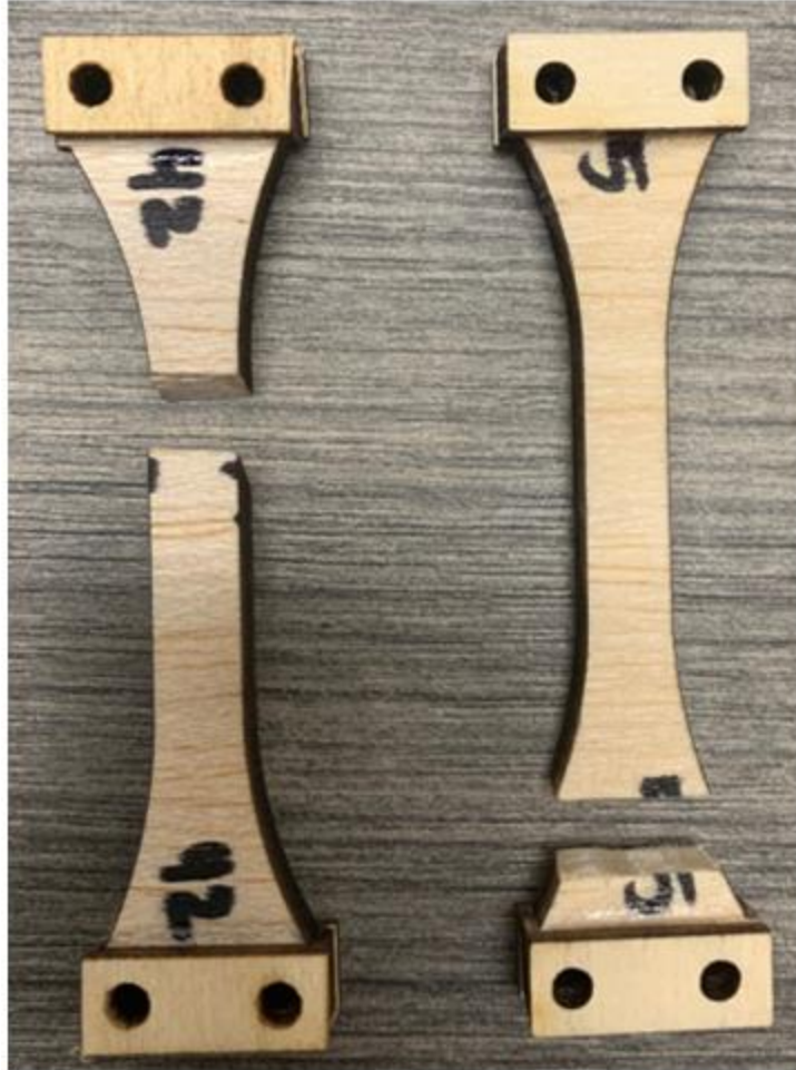
Figure 37: Failure Inside Gage Area (Left), Failure Outside Gage Area (Right)
