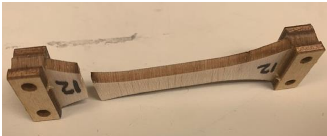
Figure 62: XL_12, Correctly Predicted Failure Location
