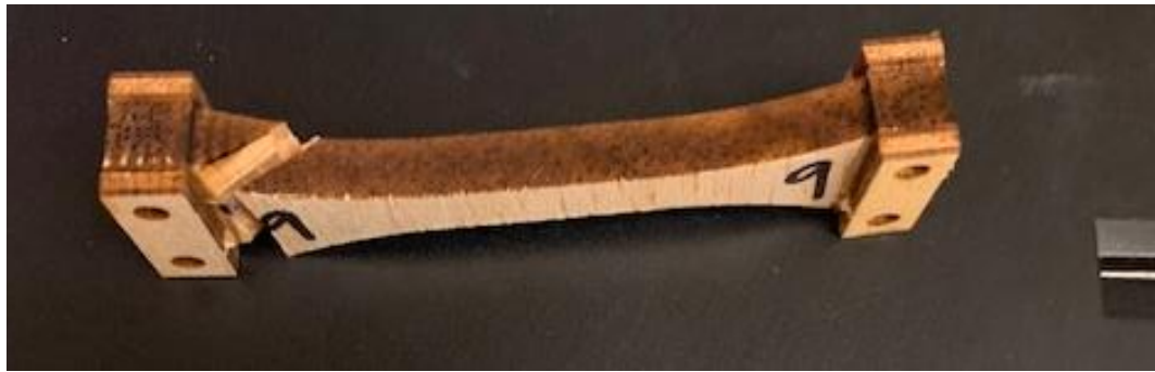
Figure 64: XH_9, 0.25" Correct Failure Location
