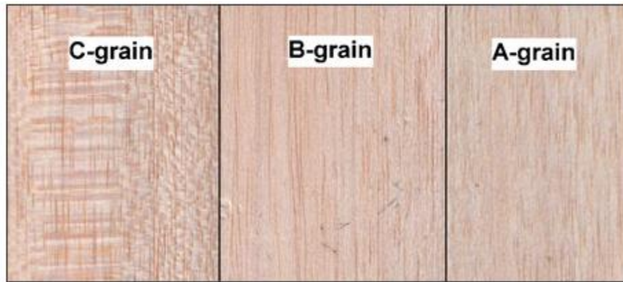
Figure 4: Grain Direction Shown on Broadside of Sheet [3]
