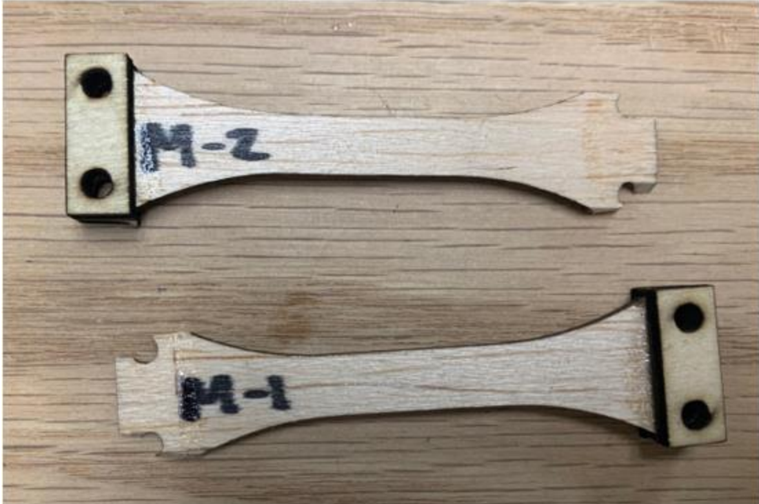
Figure 45: Failure Due to Bearing Stress
