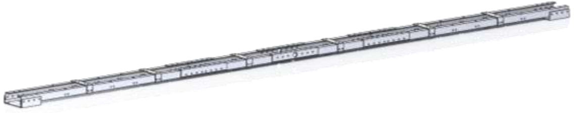
Figure 3.3. Skeletal structure housing the experimental wellbore and BHA, the power system.
