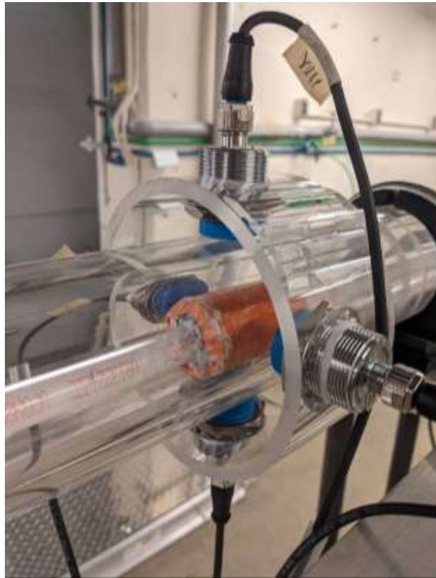
Figure 3.10. Proximity-sensor stations over the metallic stabilizer of the BHA.
