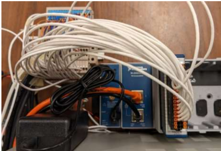
Figure 3.21. Simultaneous communication DAQ (cDAQ) and its terminal block.
